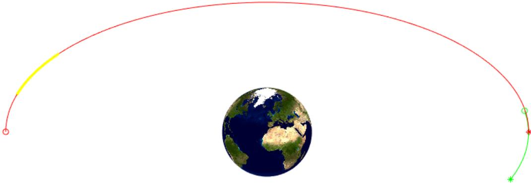
Figure 9.27: Phasing maneuver (Circular and equatorial orbit  $\rightarrow true\ longitude = 180^\circ$ ).
