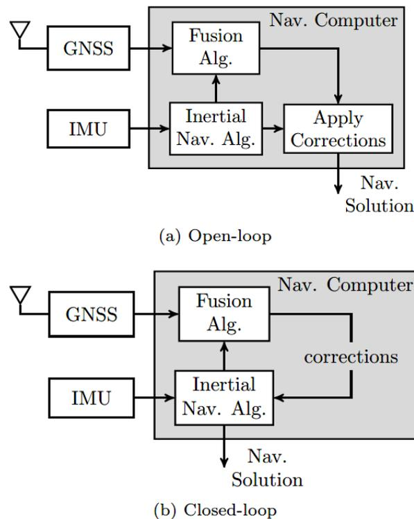
Figure 2.3: Open-loop and closed-loop architectures in hybrid IMU/GNSS system [7]
