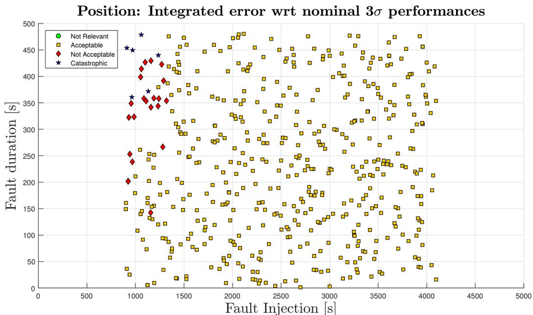
Figure 5.12: GNSS FDIR Validation: position performances (Simulation FD-04)
