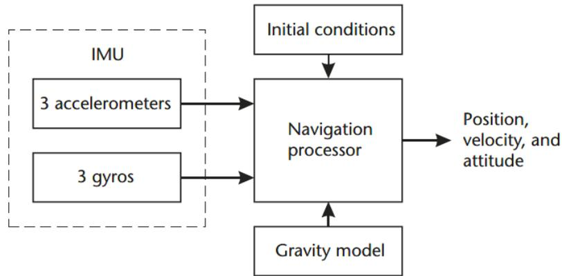
Figure 1.1: Inertial Navigation System (INS) basic scheme [2]
