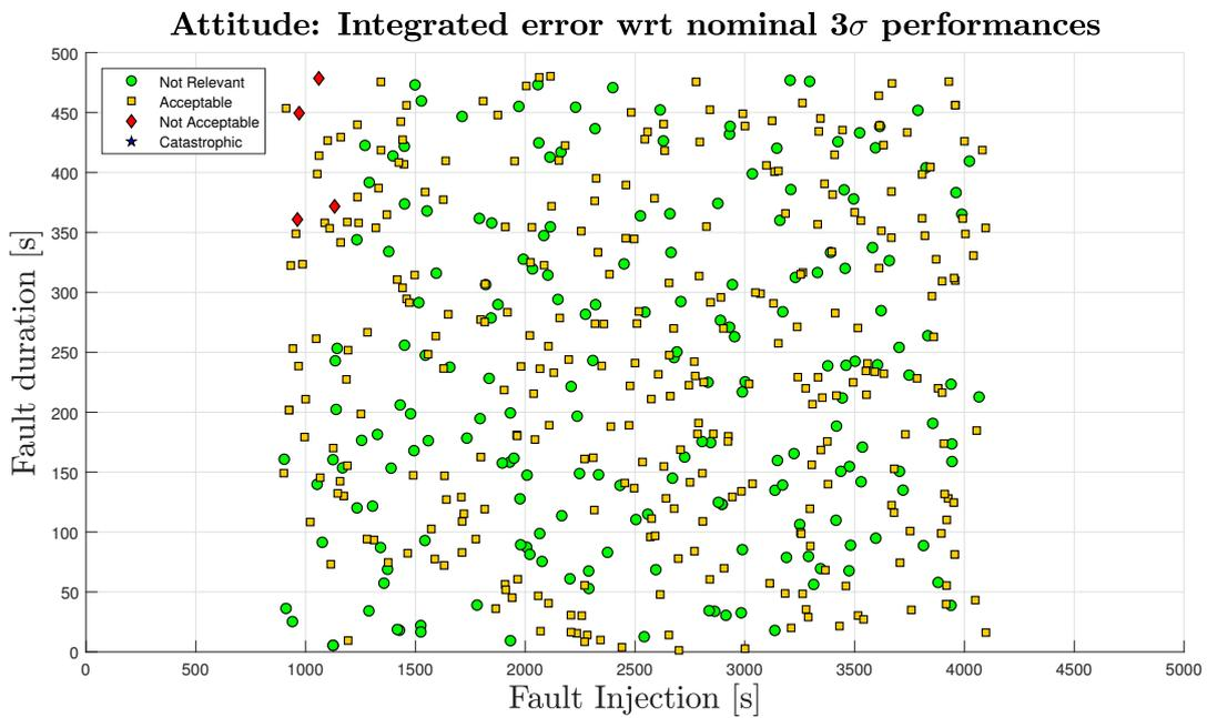
Figure 5.14: GNSS FDIR Validation: attitude performances (Simulation FD-04)
