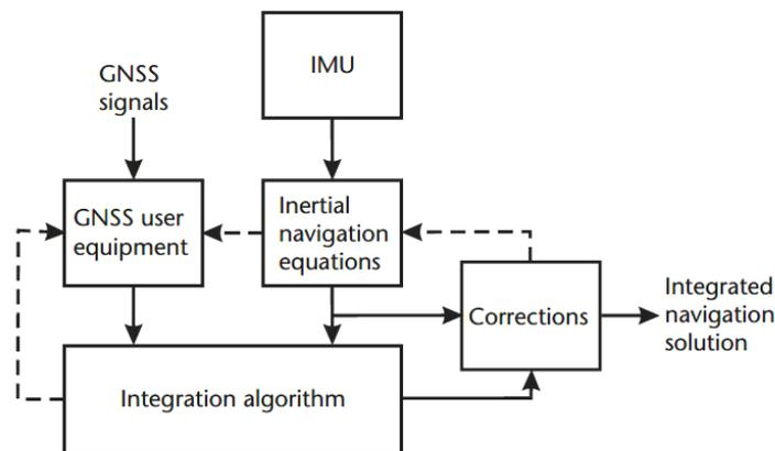
Figure 2.2: Basic integrated navigation system architecture [2]
