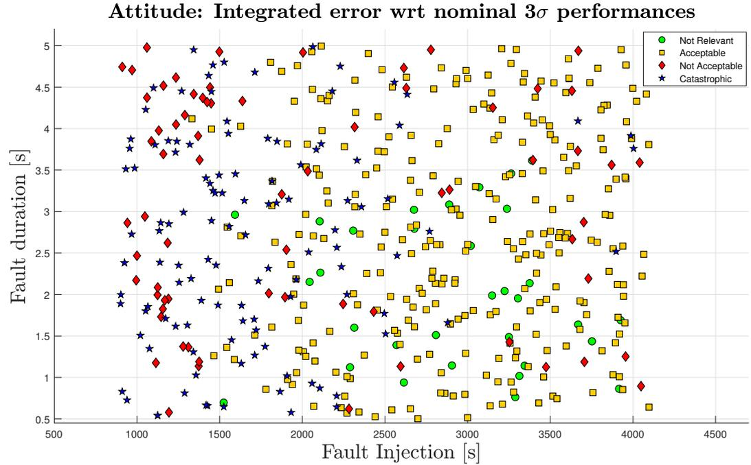
Figure 5.35: IMU FDIR Validation: attitude performances (Simulation FD-17)
