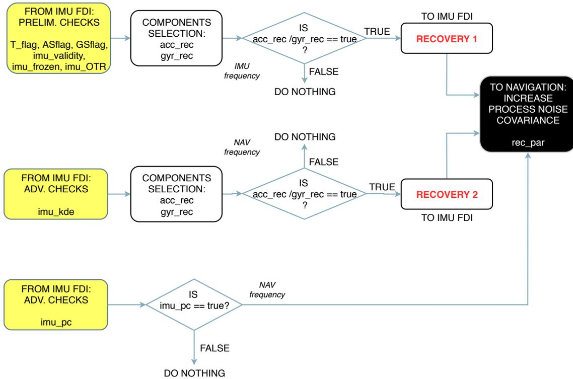
Figure 4.9: NAV\_FDIR: IMU (2nd level) logic
