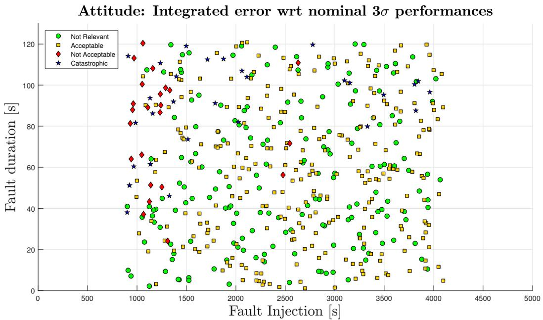
Figure 5.21: GNSS FDIR Validation: attitude performances (Simulation FD-06)
