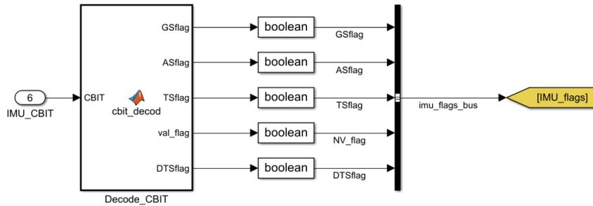
Figure 4.18: IMU's flags handling model
