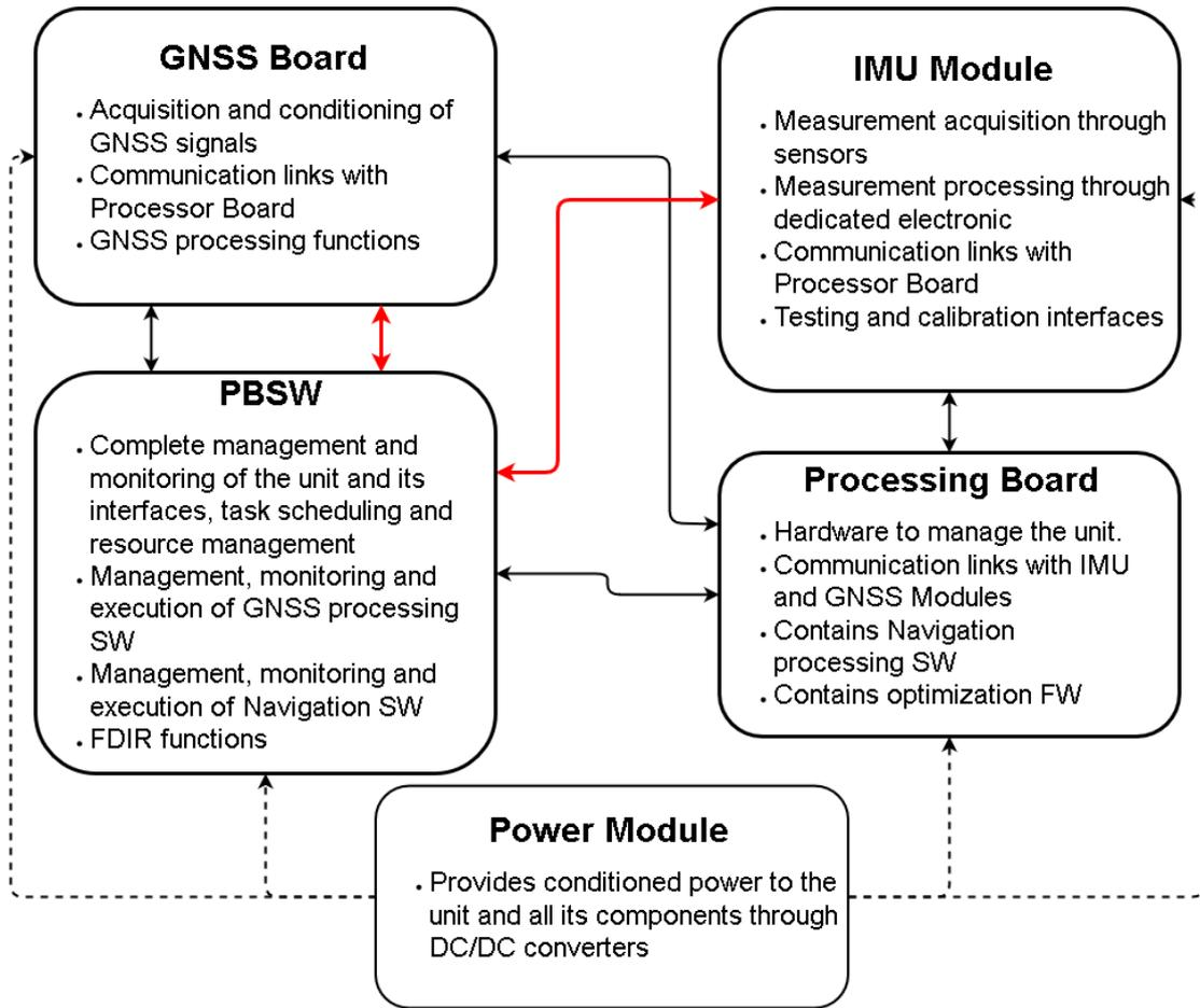
Figure 3.3: Hybrid Navigation Unit architecture and functions
