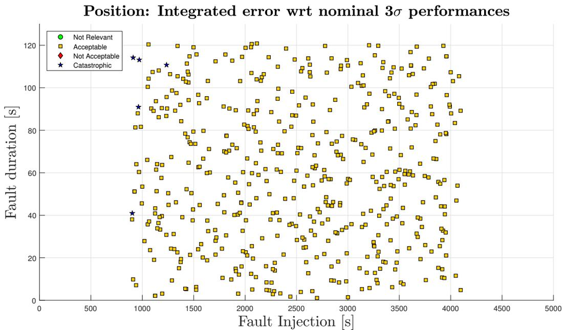
Figure 5.16: GNSS FDIR Validation: position performances (Simulation FD-05)
