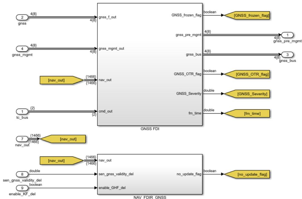
Figure 4.11: GNSS FDIR levels
