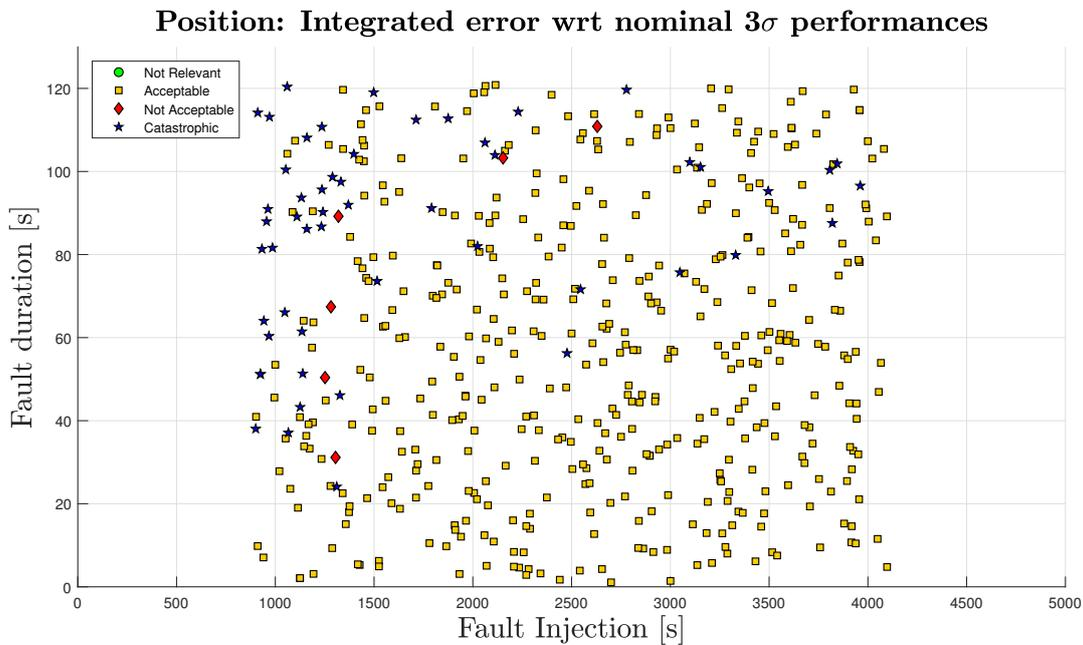
Figure 5.19: GNSS FDIR Validation: position performances (Simulation FD-06)
