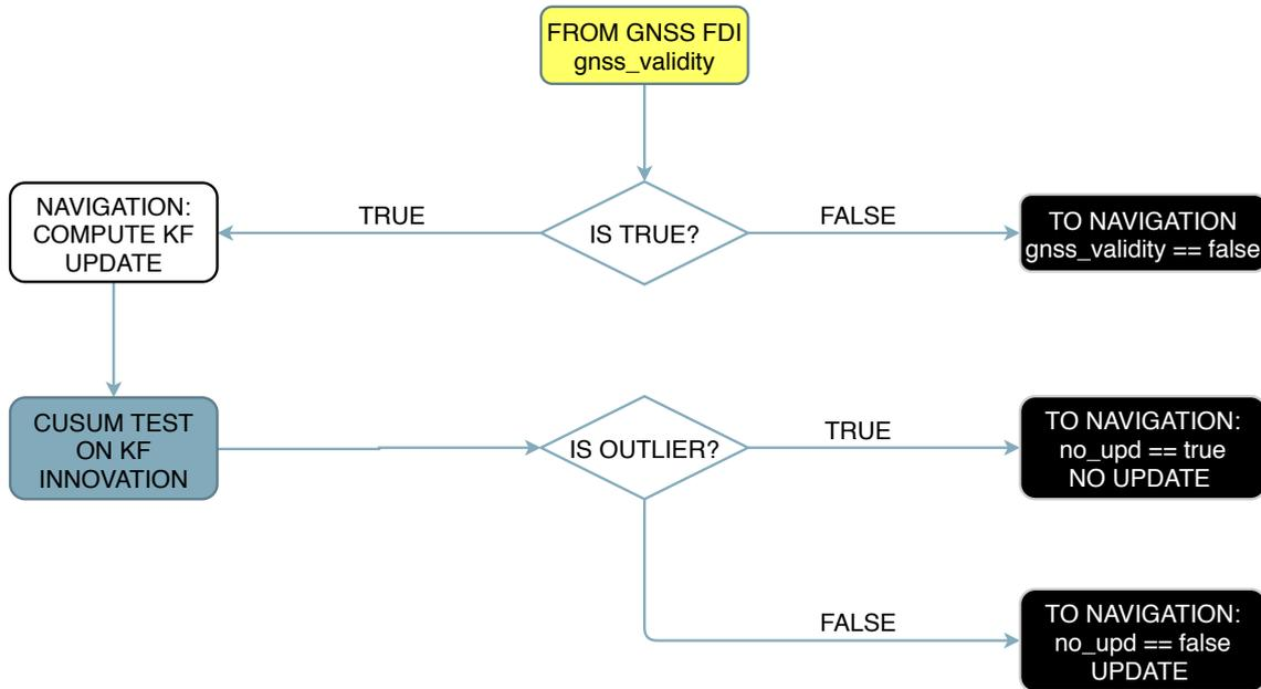
Figure 4.7: NAV\_FDIR: GNSS (2nd level) logic
