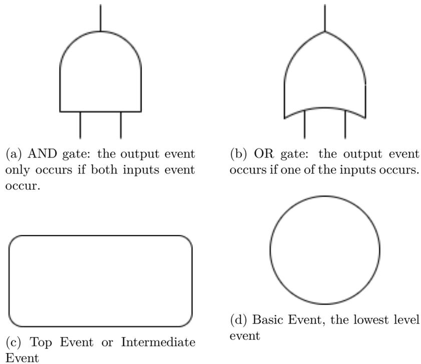
Figure 3.4: Symbols used for the Fault Tree Analysis [21]
