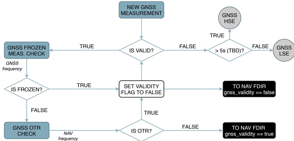
Figure 4.6: GNSS FDI (1st level) logic
