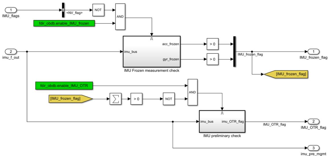
Figure 4.15: IMU FDI Preliminary Checks model
