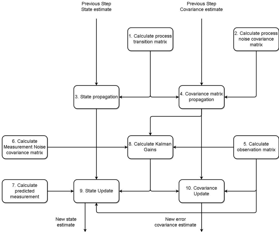
Figure 2.8: Schematic view of Kalman Filter Algorithm from [2]
