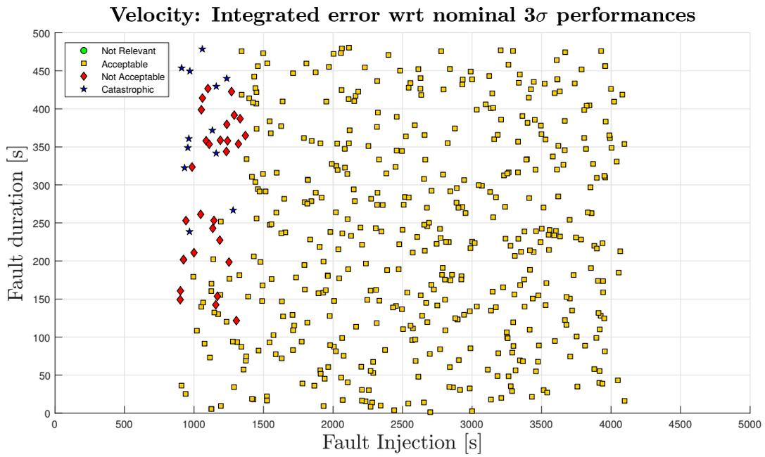
Figure 5.13: GNSS FDIR Validation: velocity performances (Simulation FD-04)
