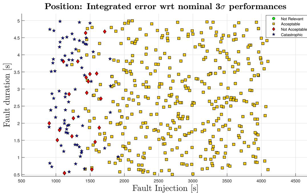
Figure 5.33: IMU FDIR Validation: position performances (Simulation FD-17)
