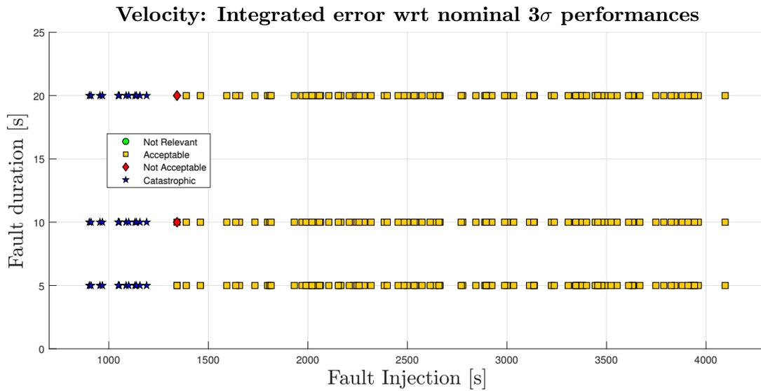
Figure 5.26: Hybrid navigation unit velocity performances for frozen IMU measurements (Simulations FD-10, FD-11 and FD-12)
