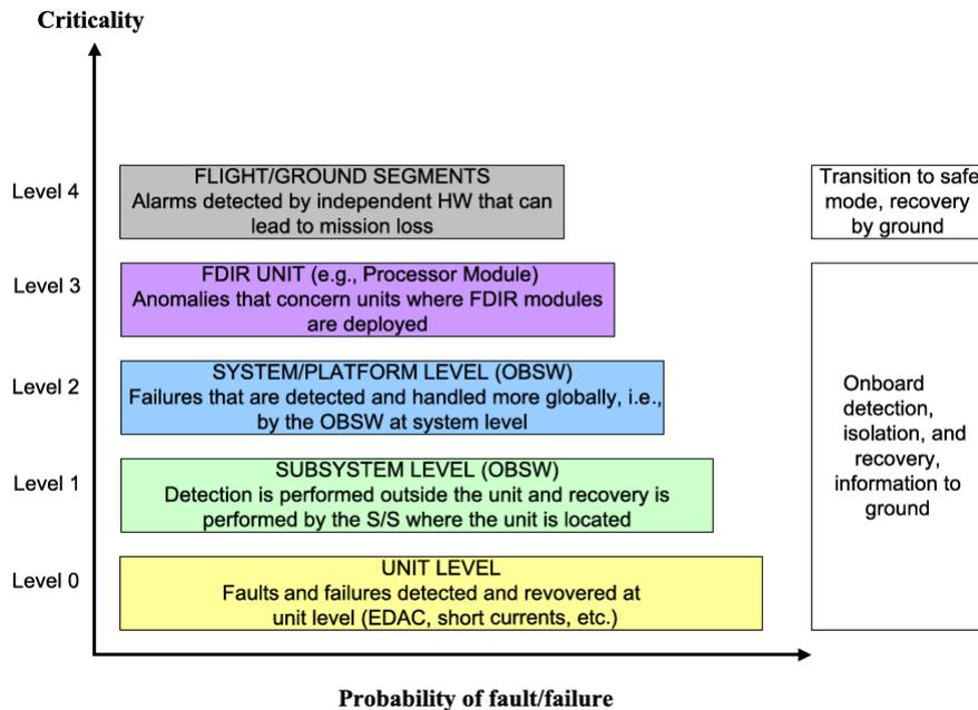
Figure 3.1: Example of spacecraft FDIR hierarchical structure
