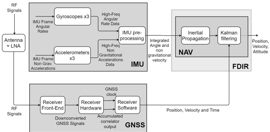
Figure 3.2: Hybrid Navigation Unit functional scheme
