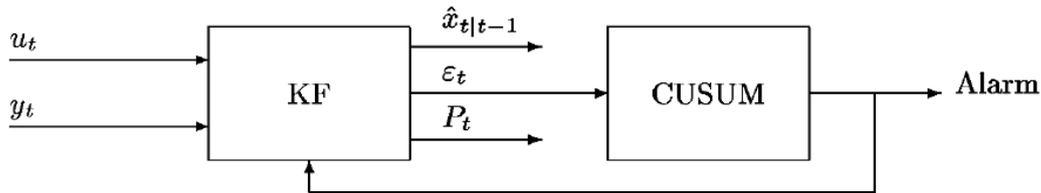
Figure 4.2: Whiteness innovation test for Kalman filter, where  $\epsilon_t$  is the innovation [22]
