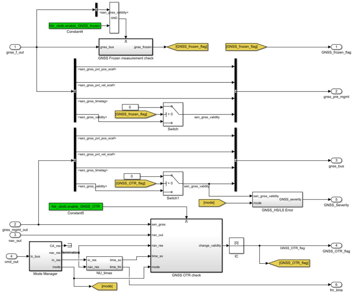
Figure 4.12: GNSS FDIR 1st level model
