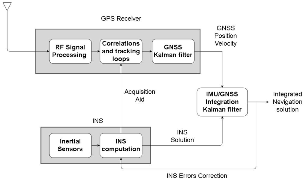
Figure 2.4: Loosely coupled architecture schematic view from [8]
