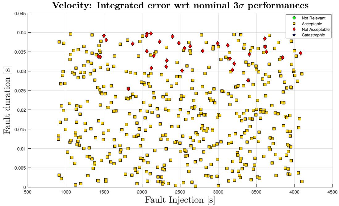
Figure 5.29: IMU FDIR Validation: velocity performances (Simulation FD-15)
