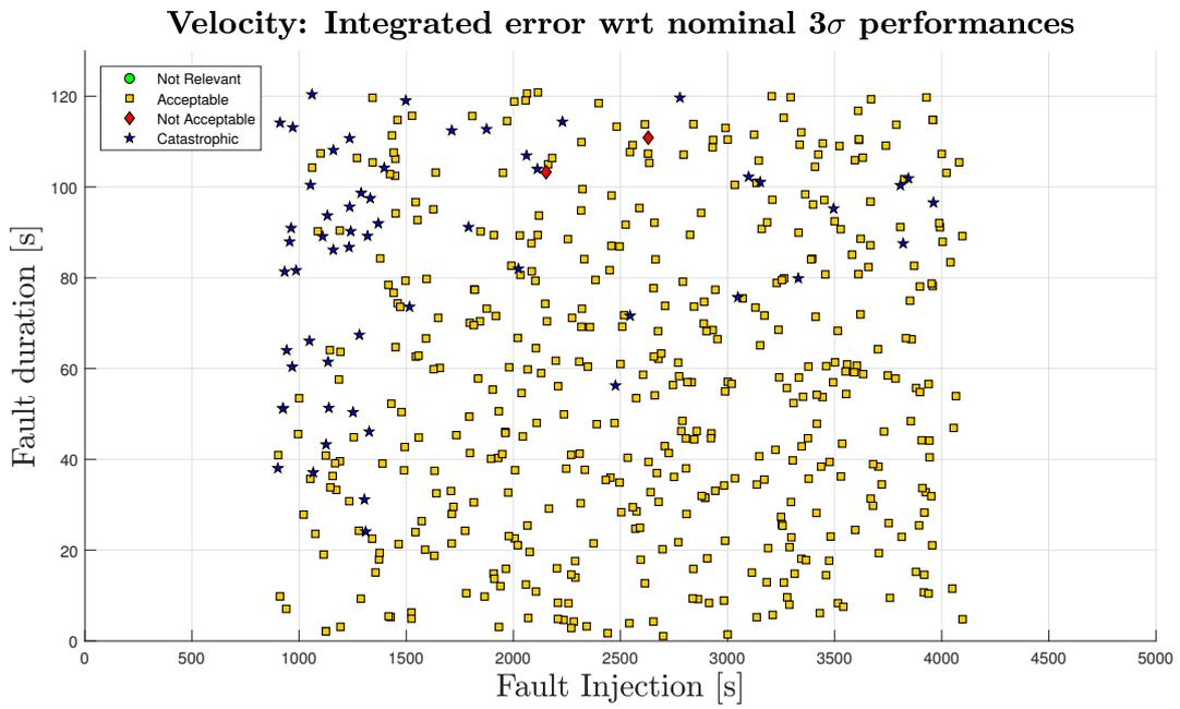
Figure 5.20: GNSS FDIR Validation: velocity performances (Simulation FD-06)
