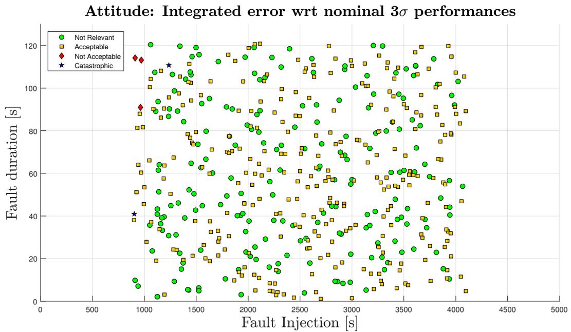
Figure 5.18: GNSS FDIR Validation: attitude performances (Simulation FD-05)
