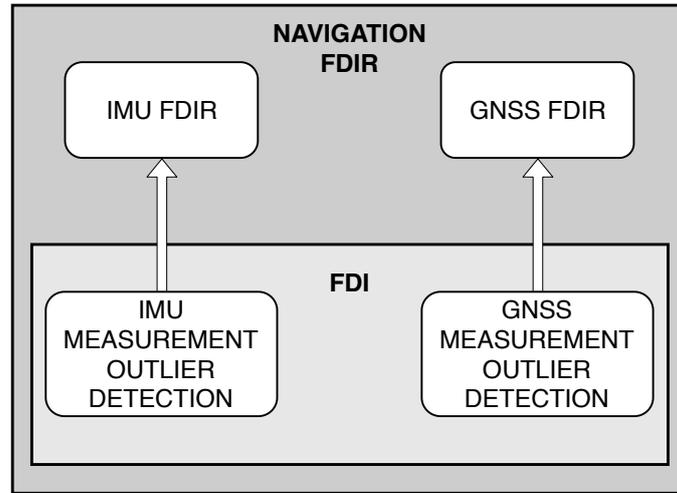
Figure 4.4: Basic FDIR hierarchy and levels
