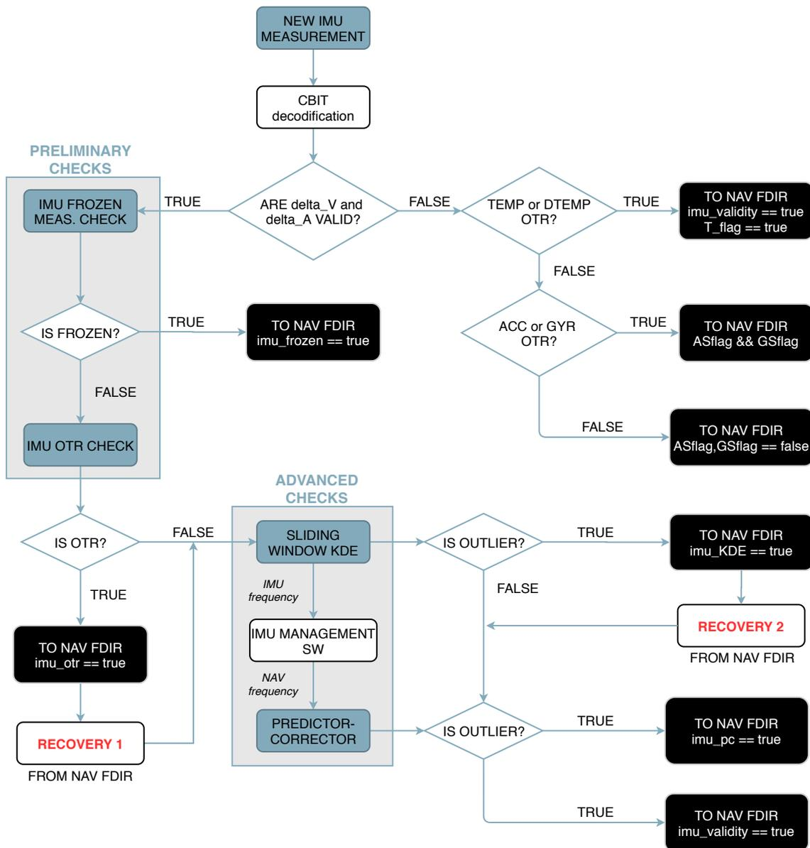
Figure 4.8: IMU FDI (1st level) logic
