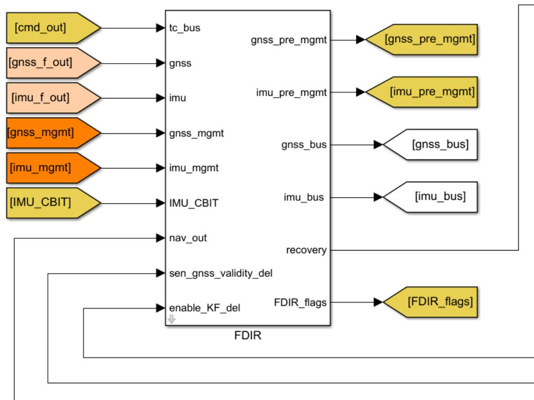
Figure 4.10: FDIR model integrated in SENER Aeroespacial hybrid navigation simulator
