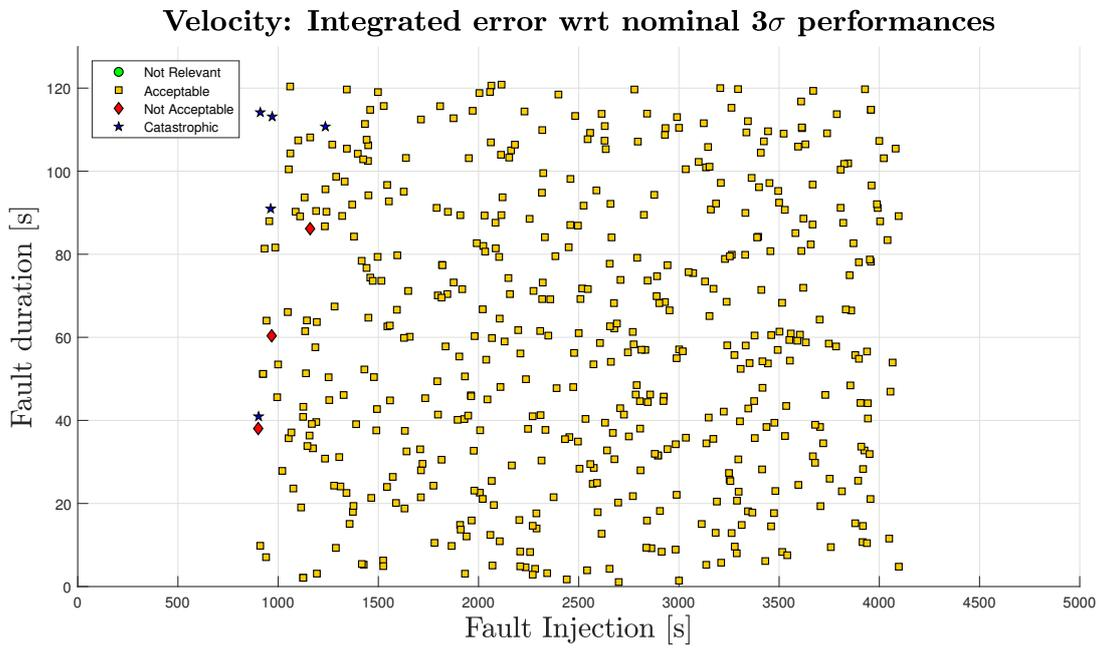
Figure 5.17: GNSS FDIR Validation: velocity performances (Simulation FD-05)
