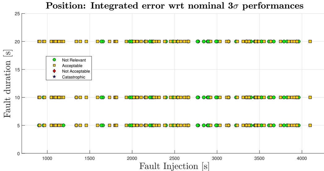
Figure 5.22: Hybrid navigation unit position performances for frozen gyroscopes measurements (Simulations FD-07, FD-08 and FD-09)
