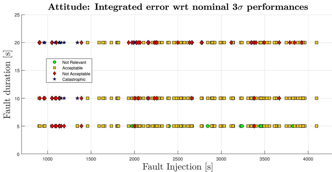
Figure 5.24: Hybrid navigation unit attitude performances for frozen gyroscopes measurements (Simulations FD-07, FD-08 and FD-09)
