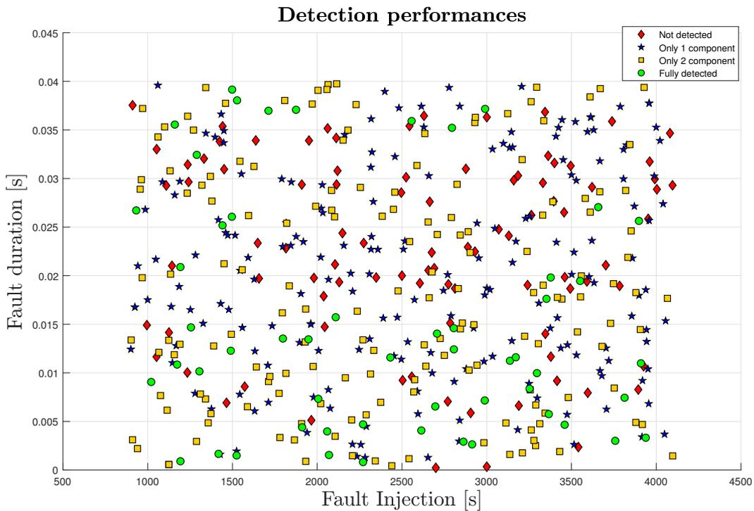
Figure 5.28: IMU FDIR Validation: detection performances (Simulation FD-15)
