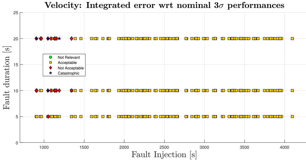
Figure 5.23: Hybrid navigation unit velocity performances for frozen gyroscopes measurements (Simulations FD-07, FD-08 and FD-09)
