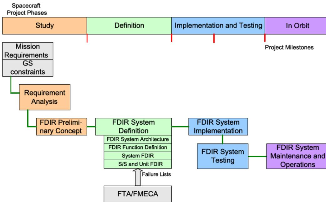
Figure 1.2: FDIR development phases vs project phases [6]
