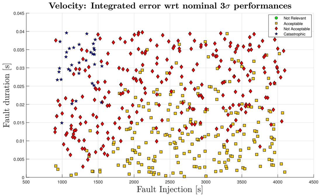
Figure 5.30: IMU FDIR Validation: velocity performances (Simulation FD-16)
