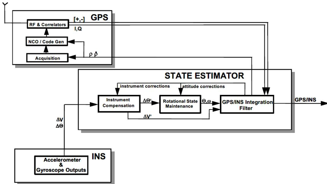
Figure 2.6: Deeply integrated systems schematic view [10]
