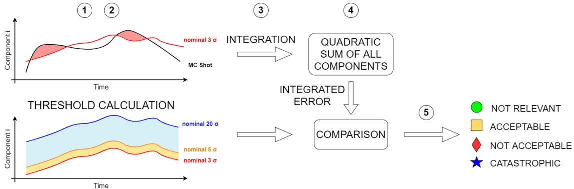
Figure 5.8: Procedure used to interpret FDIR results
