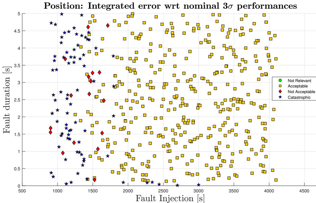
Figure 5.36: IMU FDIR Validation: position performances (Simulation FD-18)
