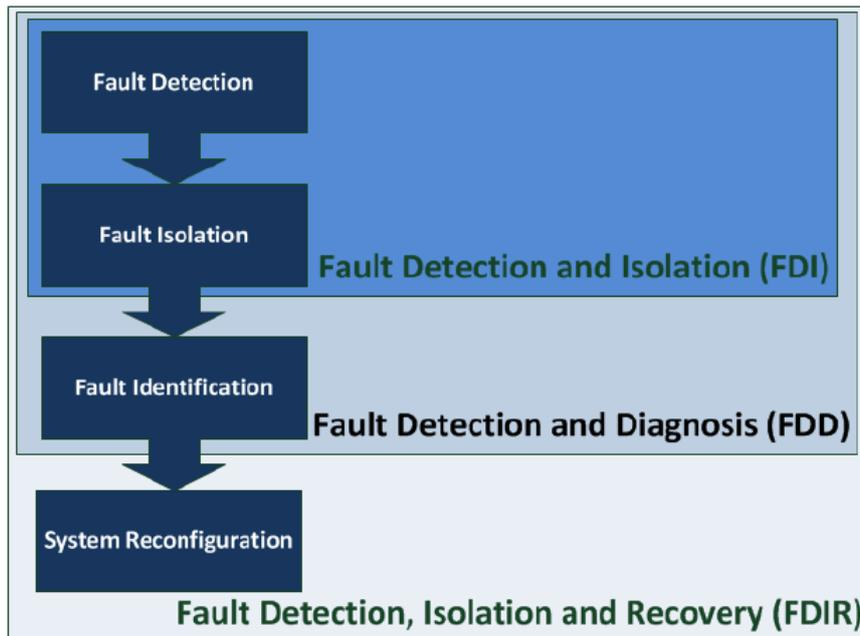
Figure 2.9: Schematic view of Fault Detection, Isolation and Recovery Functions [15]
