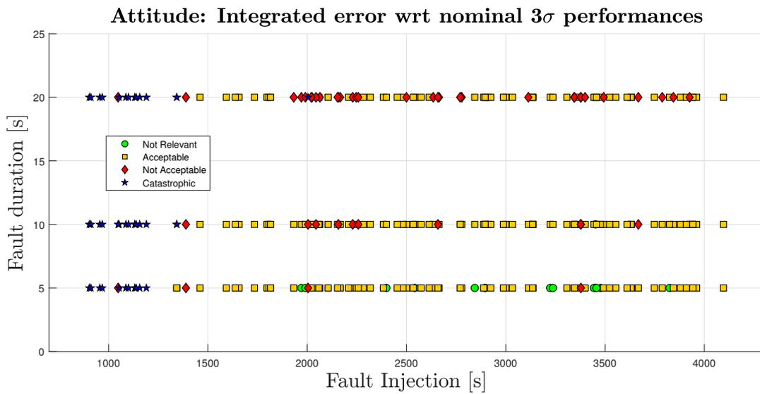
Figure 5.27: Hybrid navigation unit attitude performances for frozen IMU measurements (Simulations FD-10, FD-11 and FD-12)
