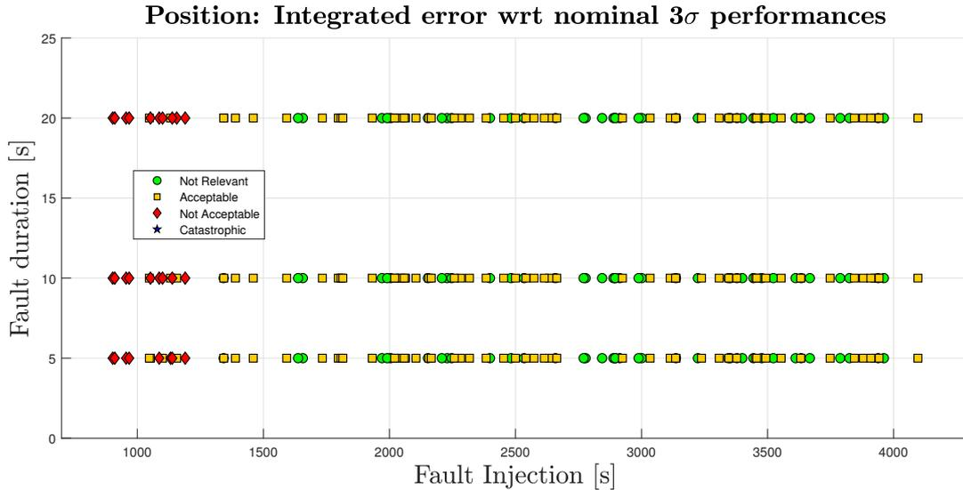
Figure 5.25: Hybrid navigation unit position performances for frozen IMU measurements (Simulations FD-10, FD-11 and FD-12)
