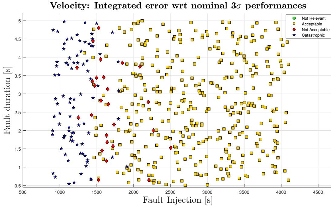
Figure 5.34: IMU FDIR Validation: velocity performances (Simulation FD-17)
