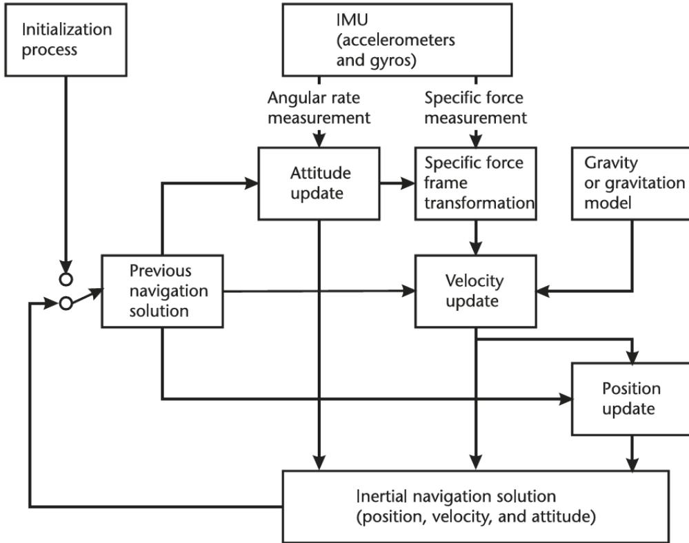
Figure 2.1: Inertial Navigation System operation [2]
