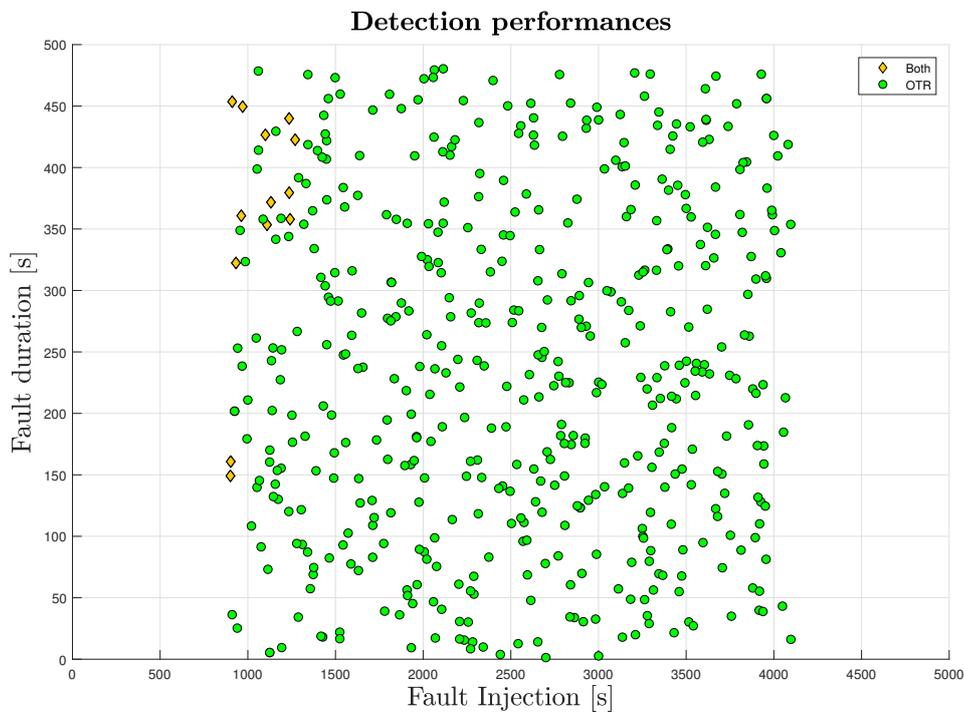
Figure 5.15: GNSS FDIR Validation: detection performances (Simulation FD-04)
