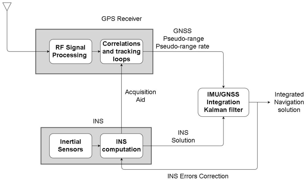
Figure 2.5: Tightly coupled architecture schematic view from [8]
