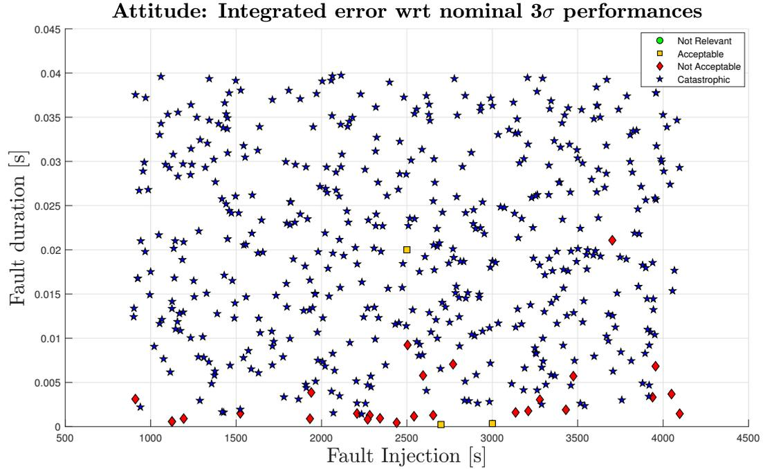
Figure 5.32: IMU FDIR Validation: attitude performances (Simulation FD-16)
