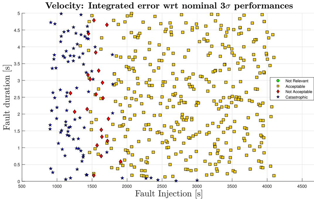
Figure 5.37: IMU FDIR Validation: velocity performances (Simulation FD-18)
