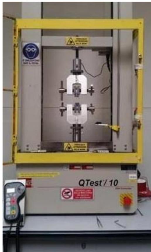
Figura 52: MTS QTest/ 10 Elite Controller.
