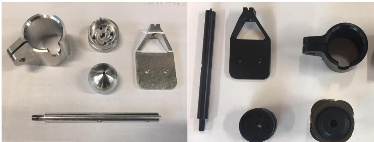
Figure 50: Manufactured parts: before and after anodization.
