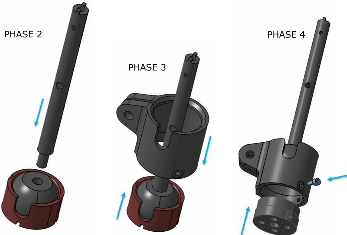
Figure 41: Installation, phase 2, 3 and 4: Completion of the Spherical Joint.
