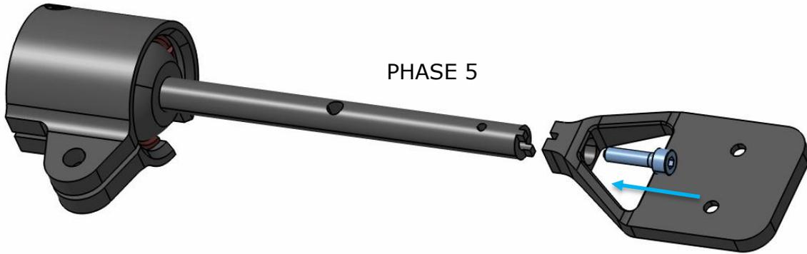
Figure 42: Installation, phase 5: Connection with the Camera Support.
