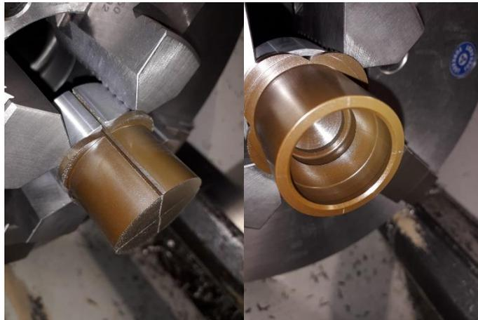
Figure 49: Manufacturing of inner ring.
