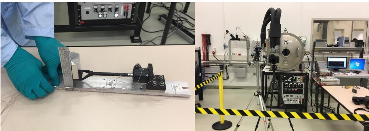
Figure 56: Installation of thermocouples and display of the camera set up.
