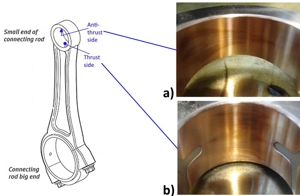
**Figure 49. Darkened surface areas present on the conrod's small eye. a) Thrust side surface. b) Opposite to thrust side surface.**
