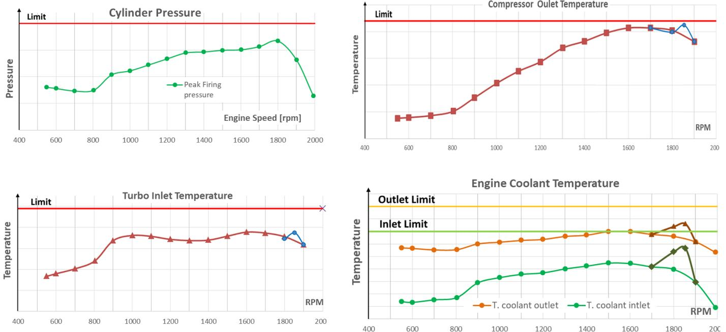
**Figure 42. Cylinder pressure and, compressor outlet, turbo inlet and engine coolant temperatures with limit values.**
