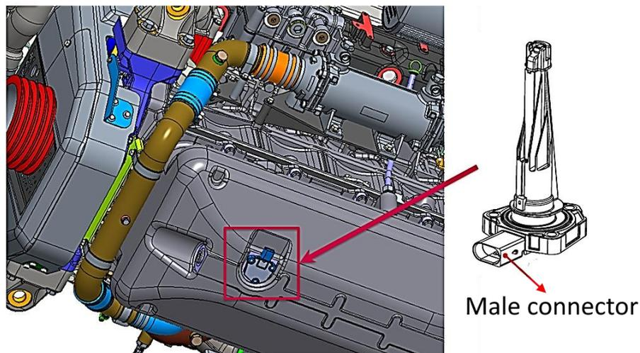
**Figure 16. Oil level sensor located at the bottom of the oil sump.**
