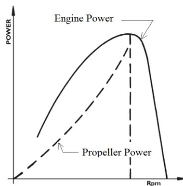
**Figure 8. Engine power and propeller absorption curves.**
