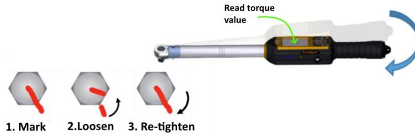
**Figure 48. Marking torque test procedure.**
