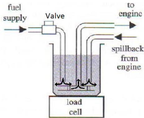
Figure 30. Gravimetric - direct weighing fuel gauge.
