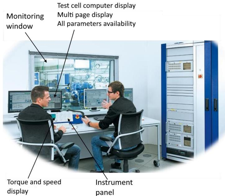
**Figure 33. Powertrain test cell control room.**
