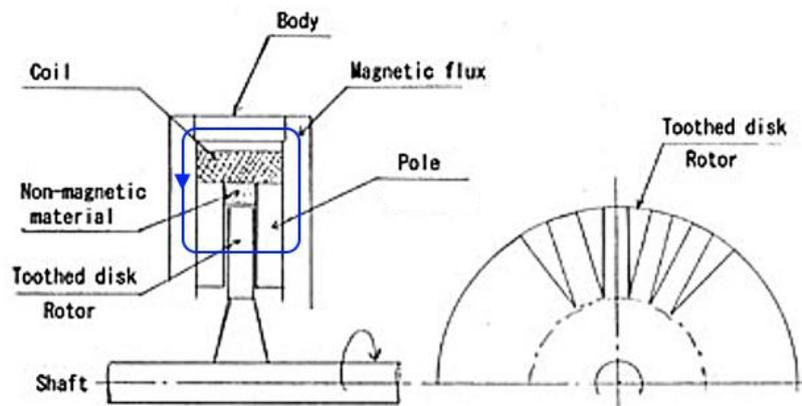
Figure 25. Working principle of the Eddy-current dynamometric brake.
