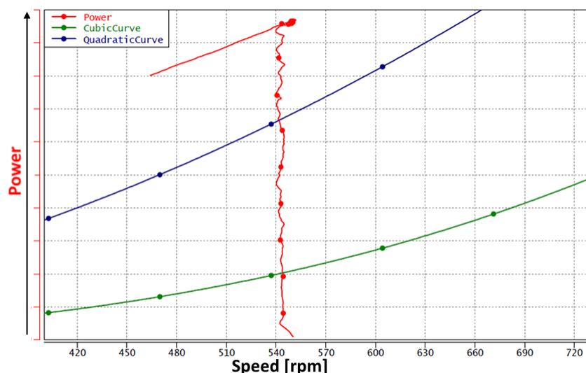
Figure 46. Lowest Propulsion Engine Speed Test Curve
