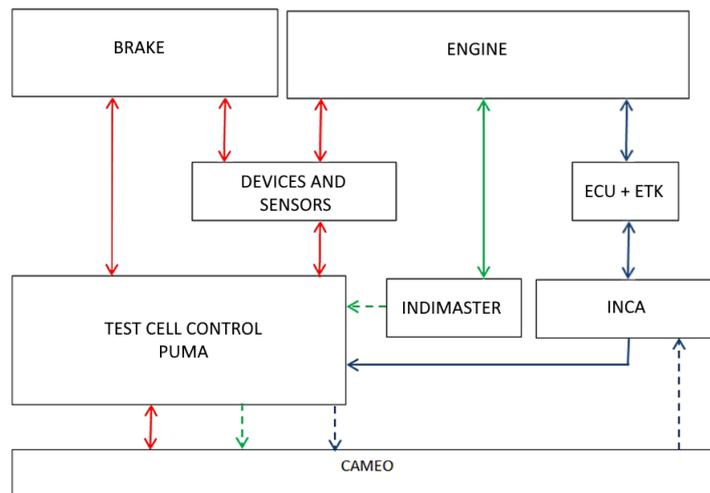
**Figure 36. Test cell management system layout**
