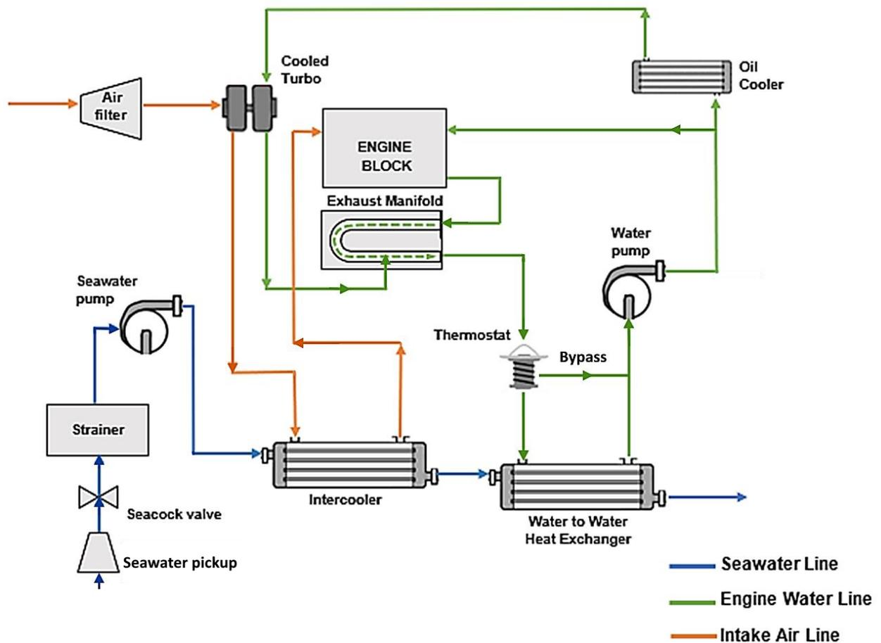
Figure 19. Seawater, engine coolant and intake air circuits.
