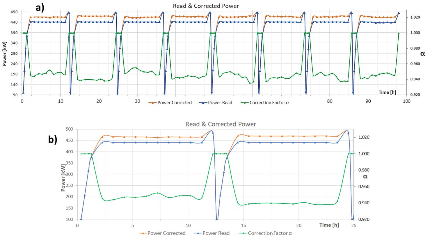
**Figure 43. Read and corrected power for a) the full 98h core tests and b) one cycle**
