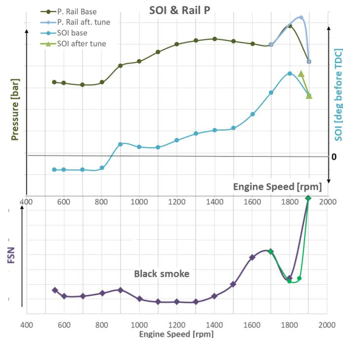
**Figure 41. Development of SOI, Rail pressure and Black Smoke curves related to the full load test.**
