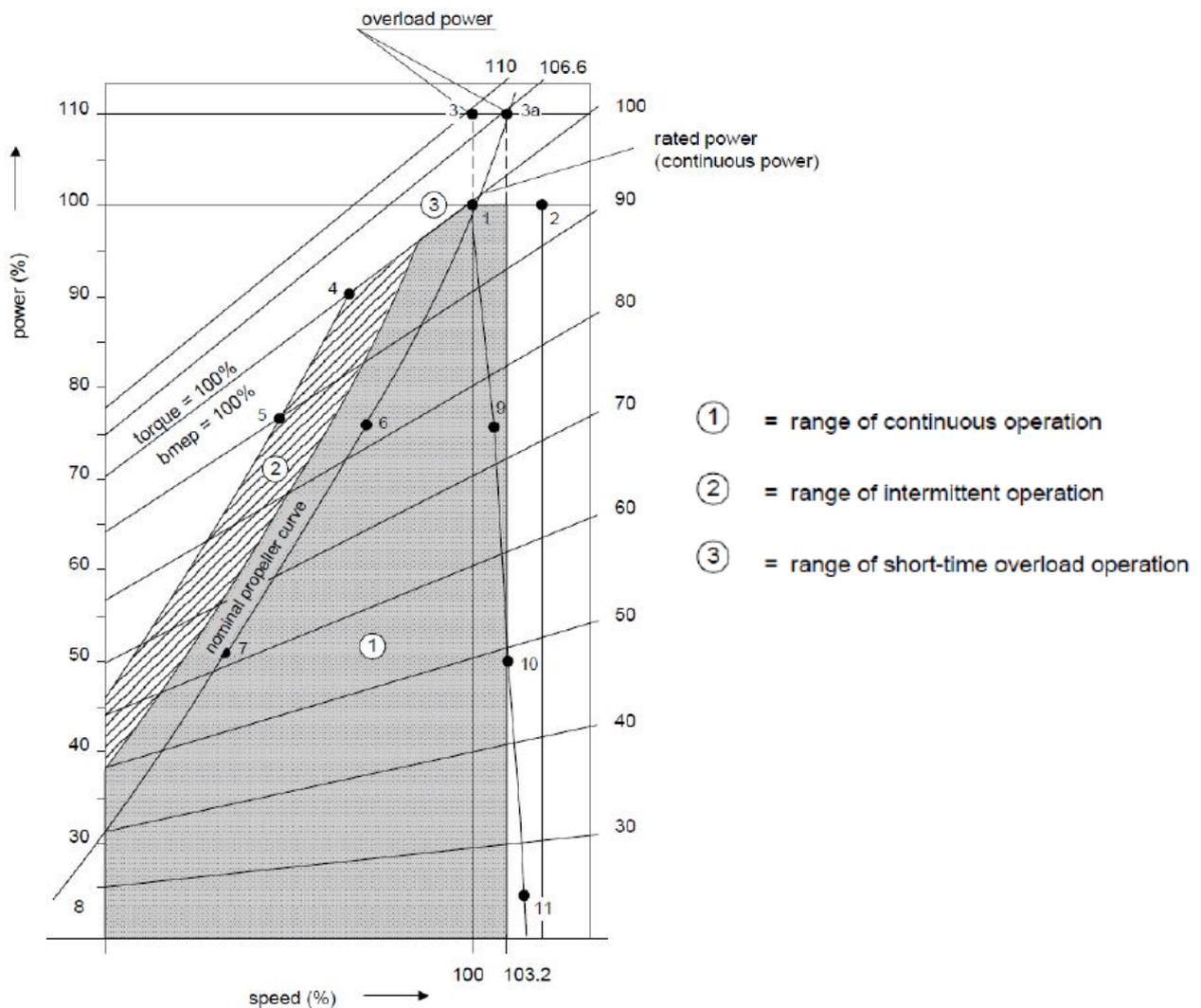
Figure 2. Power – Speed diagram
