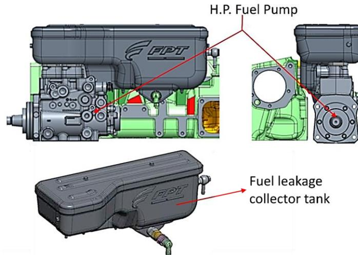
**Figure 12. Fuel leakage collector box.**
