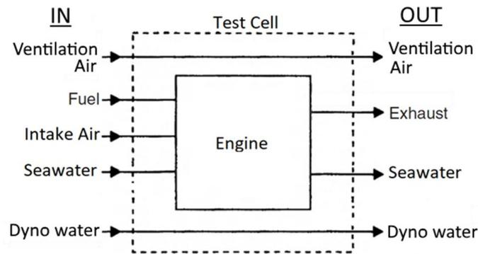
**Figure 23. Fluid flows to and from the test cell.**
