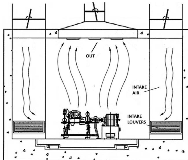
Figure 27. Test cell ventilation system layout. Modified from [12].
