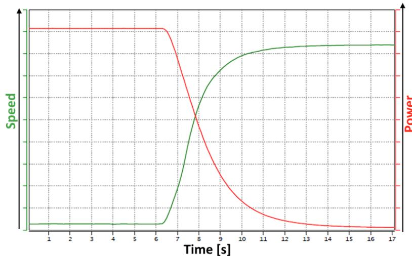
Figure 47. Speed Governor Compliance Test
