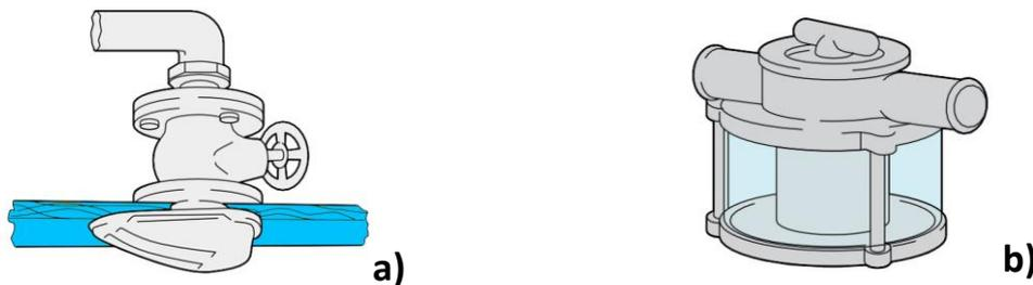
**Figure 18. a) Seacock valve placed under the sea waterline and b) Strainer to filter out smaller debris.**
