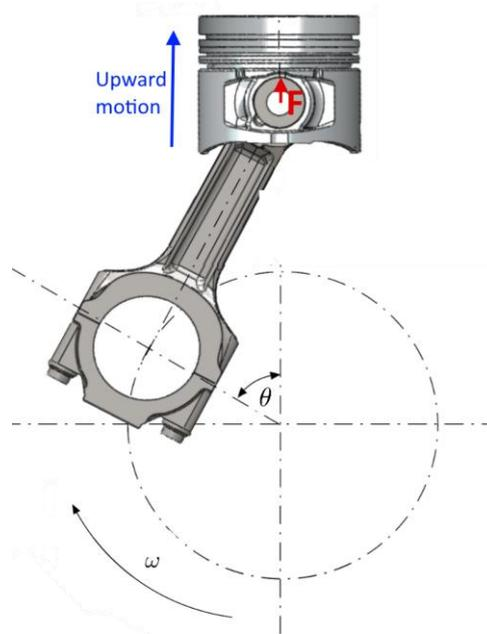
**Figure 50. Force F applied to the anti-thrust side of the conrod's small during piston upward motion.**
