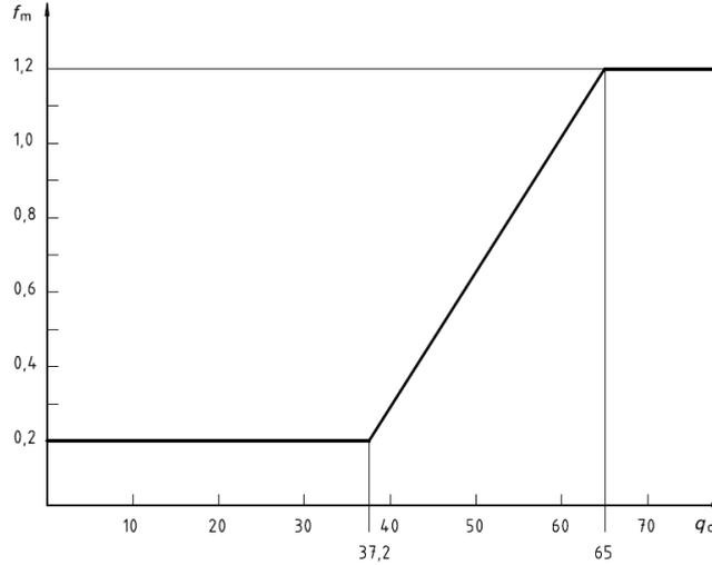
**Figure 1. Engine factor  $f_m$  vs. corrected fuel delivery  $q_c$**
