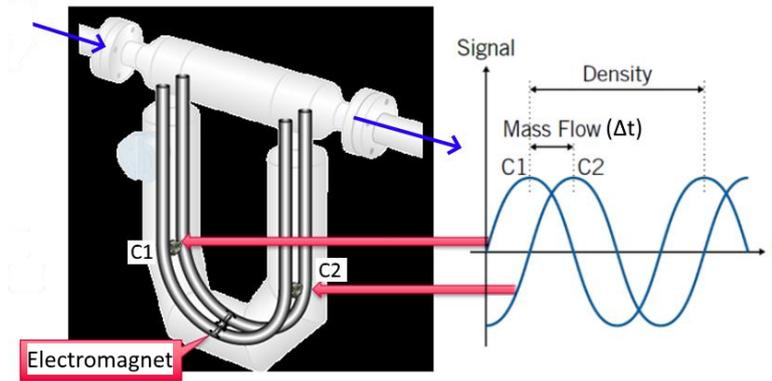
Figure 31. Coriolis effect flowmeter
