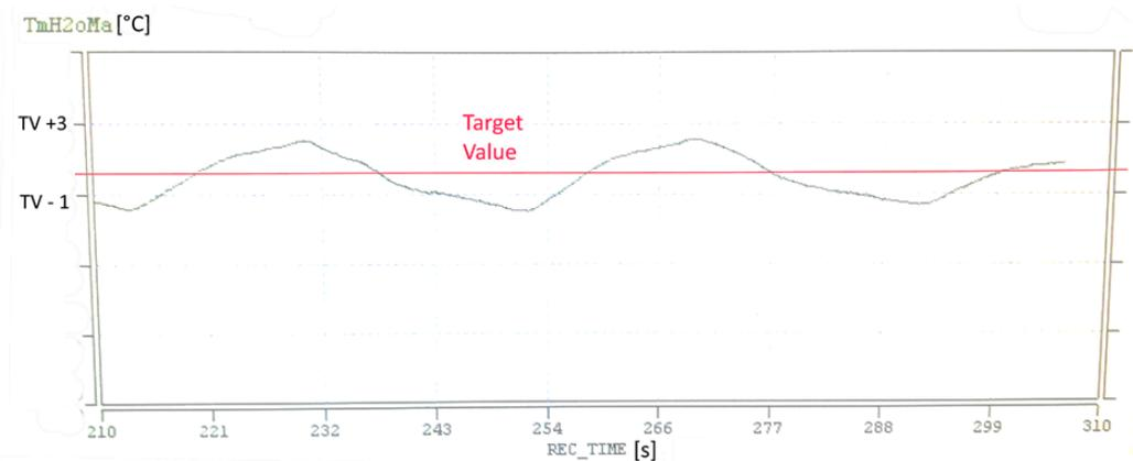
**Figure 29. Recorded seawater temperature at the engine inlet (TmH2oMa) over time. (TV: Target Value)**
