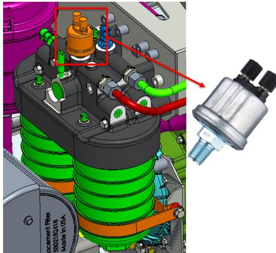
**Figure 17. Fuel pressure sensor location.**
