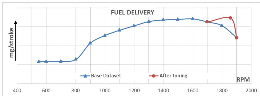
**Figure 38. Fuel delivery before and after tuning tests**
