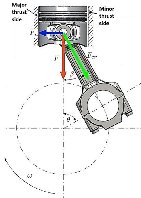
**Figure 55. Forces present on the crank mechanism in the expansion stroke.**
