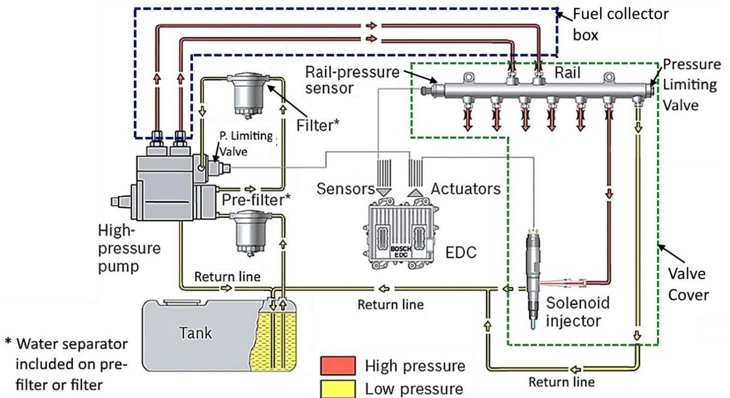
Figure 20. Common-rail diesel fuel injection system. Schematic adapted from Bosch diagram.
