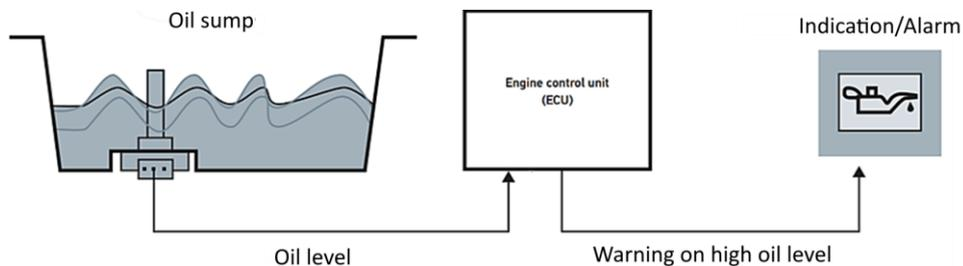
**Figure 15. Oil level sensor alarm working principle. Modified from [11].**
