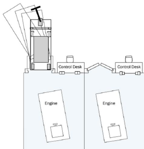
Figure 22. Test benches arrangement with frontal corridor only [12].
