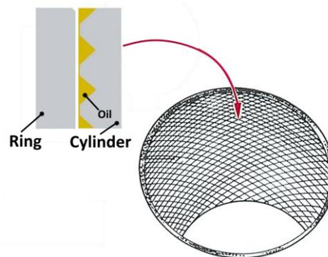
**Figure 54. Lubrication improvement achieved with honing of the cylinder liners.**
