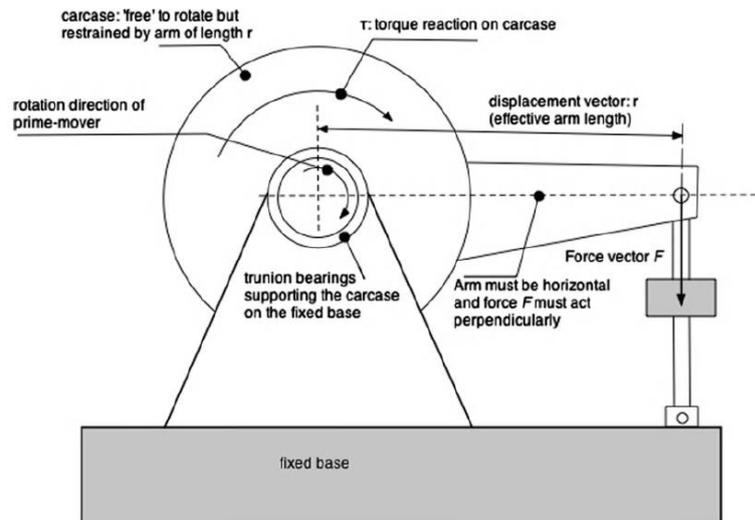
**Figure 26. Schematic of a dynamometer [12].**
