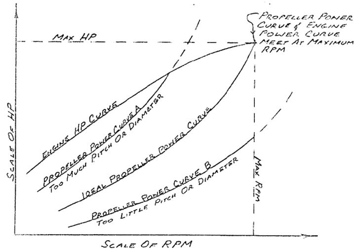
**Figure 9.** Engine and propeller power equilibrium [10].
