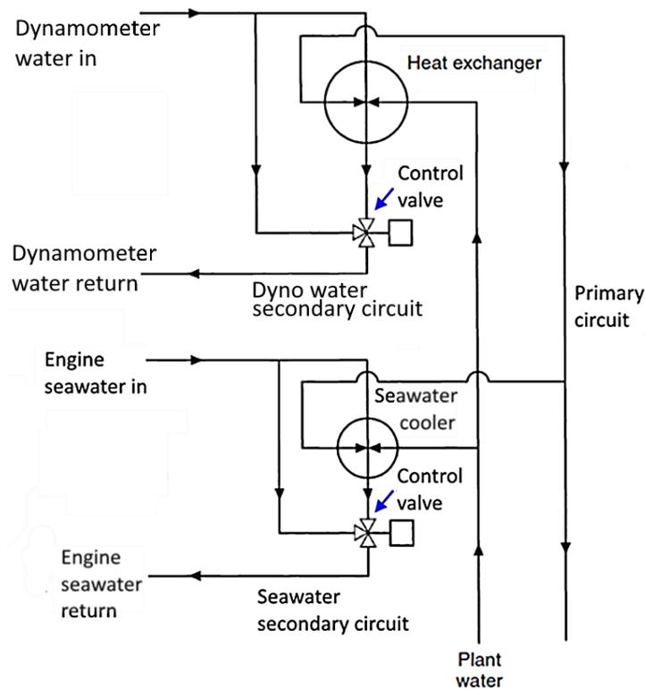
**Figure 28. Test cell and engine primary and secondary cooling circuits layout.**
