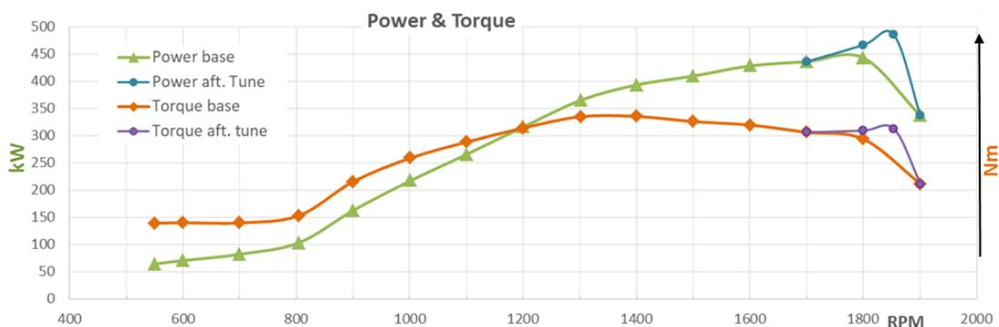
**Figure 39. Power and Torque behavior – Full load**
