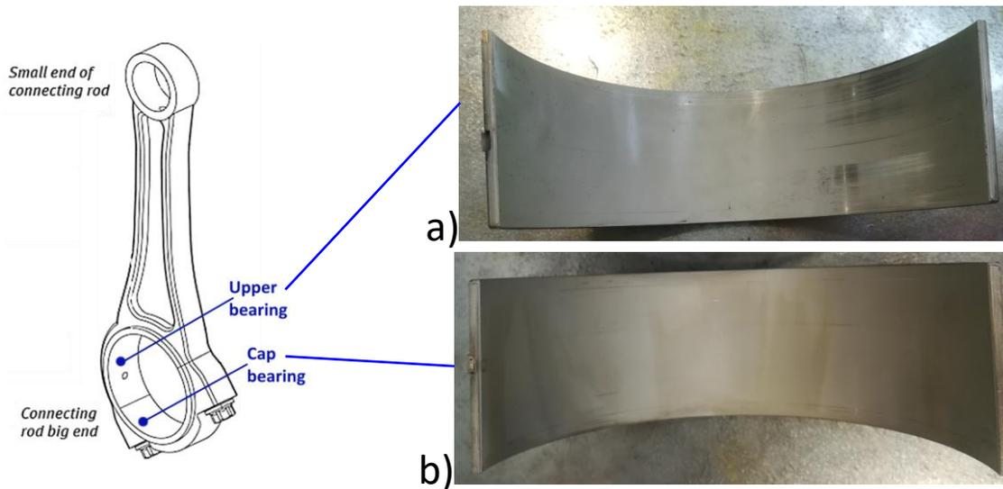
**Figure 51. Crankshaft bearings appearance. a) Upper half (thrust side). b) Lower half (cap side)**
