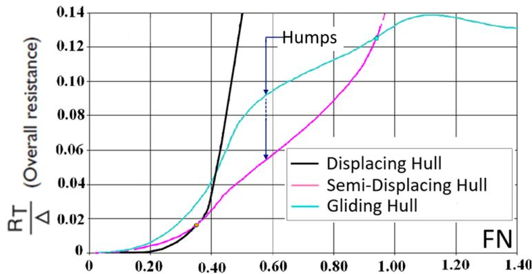
Figure 7. Different types of hull resistance characteristics [9].
