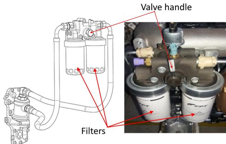
**Figure 11. Duplex type filters for avoiding flow interruption during maintenance operations.**
