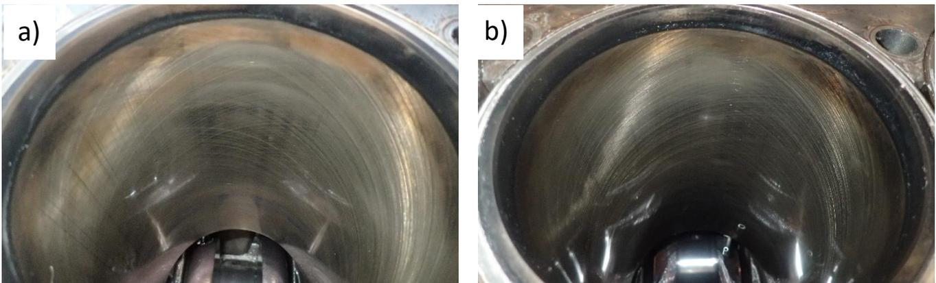
**Figure 53. Cylinder walls visual inspection. a) Major thrust side b) Minor thrust side**
