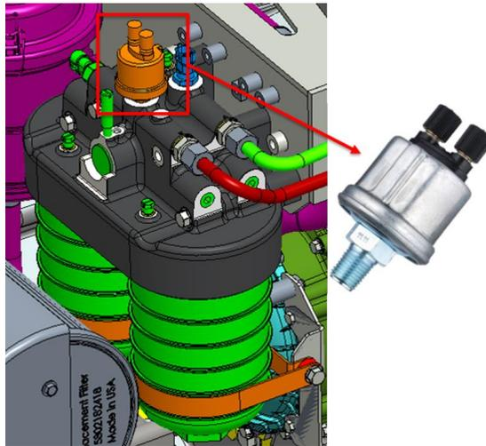
Figure 17. Fuel pressure sensor location.
