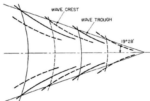
**Figure 5. Single point wave patten.**
