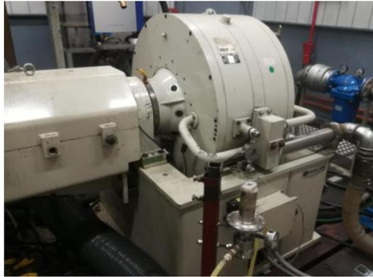
Figure 24. Dynamometric brake used in the tests.
