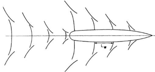
**Figure 6. Schematic diagram of the bow and stern wave systems formed by a travelling vessel [8].**
