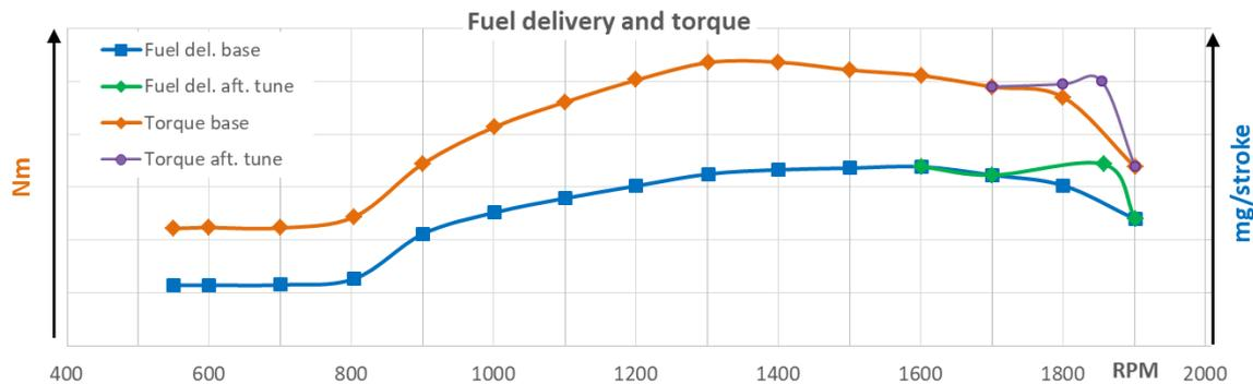
Figure 40. Relation between load and fuel injection
