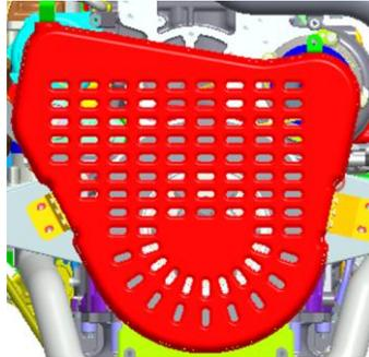
**Figure 13. FEAD cover with openings.**
