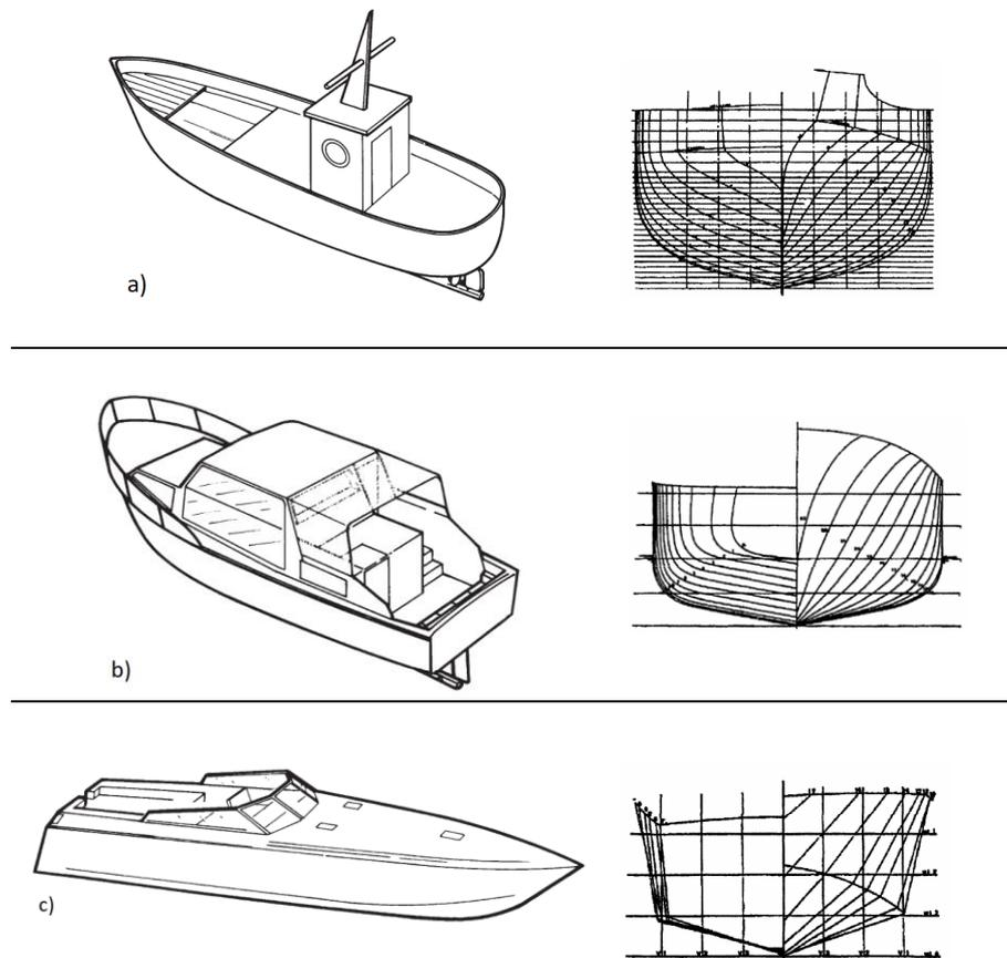
Figure 4. Different hull types. a) Displacing hull. b) Semi-displacing hull. c) Gliding hull. [6].
