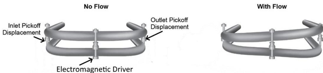
Figure 32. Tubes twisting caused by the Coriolis forces.
