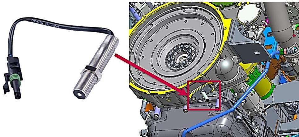
Figure 14. Overspeed sensor located on the flywheel housing
