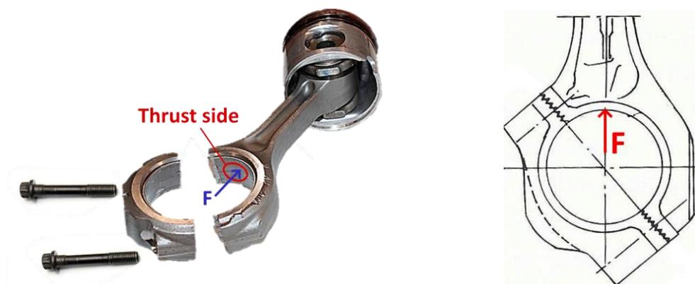
**Figure 52. Maximum force developed on the thrust side of the connective rod's big eye.**
