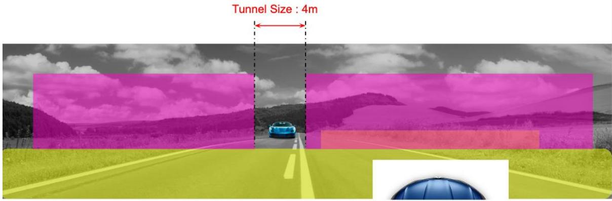
Beam Pattern Incoming Car @ 250 m with aiming tolerance +/-0.7°
