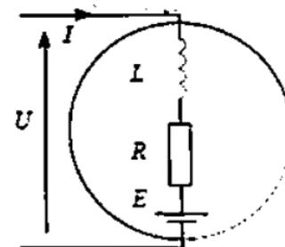
Equivalent electric circuit of the rotor
