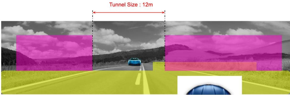
Beam Pattern Incoming Car @ 150 m with aiming tolerance +/-0.1°
