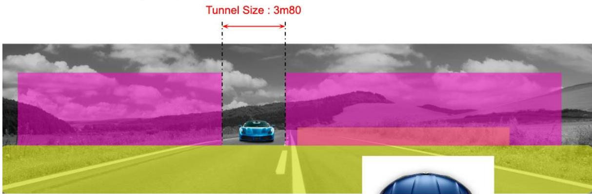
Beam Pattern Incoming Car @ 150 m with aiming tolerance +/-0.7°
