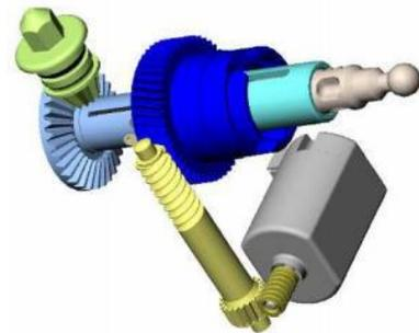
**Figure 5:** Architecture of the geared motor associated to the screw nut system
