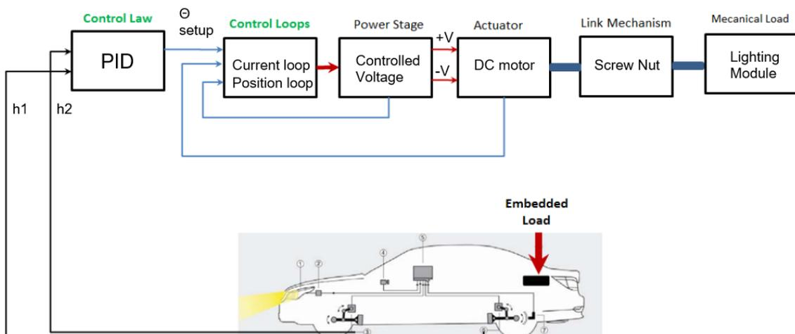
**Figure 7:** Block scheme of the headlight levelling system
