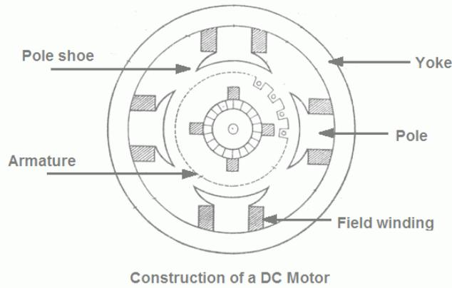
DC machine: operating principle
