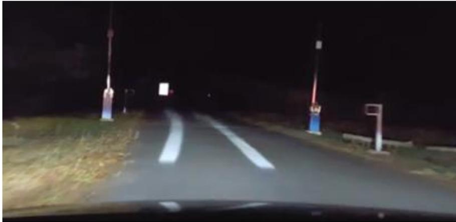
Different shapes are also available, with either stripes reproducing the road marking lines, or a complete “carpet” in front of the vehicle, or even “2D Lanes” with also transversal stripes, for example, to provide distance information.
