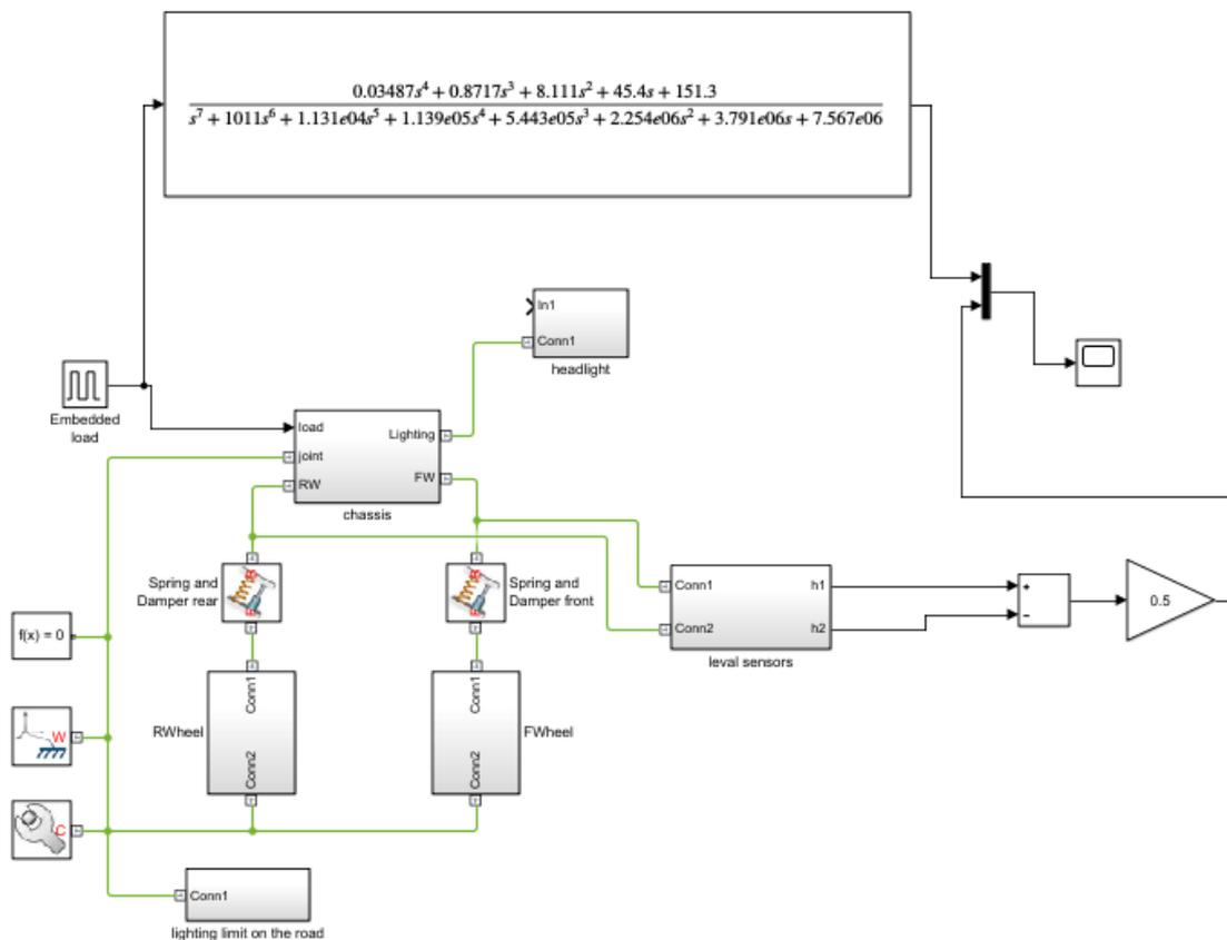
Simulink model with control loop
