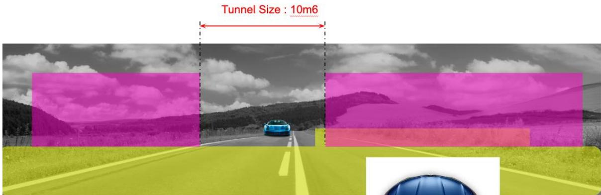
Beam Pattern Incoming Car @ 250 m with aiming tolerance +/-1°
