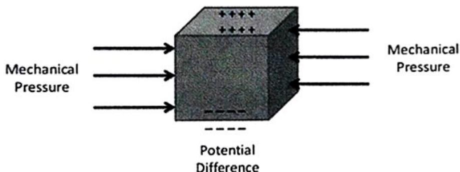
In the piezoelectric motor (USM), the working principle is based on the Converse
