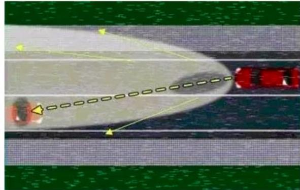
Figure 2 Reflection of AFS Light in Rainy Water (Looking Down)
