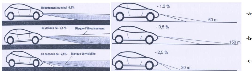
**Figure 2:** Effect of the embedded the load on the light beam
