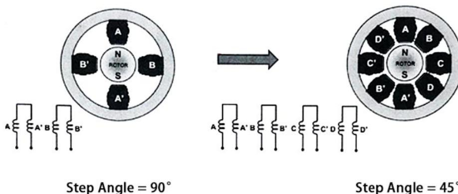
Comment : Micro stepping motors are designed according to case 1 or 2 depending on the desired step angle and the cost
