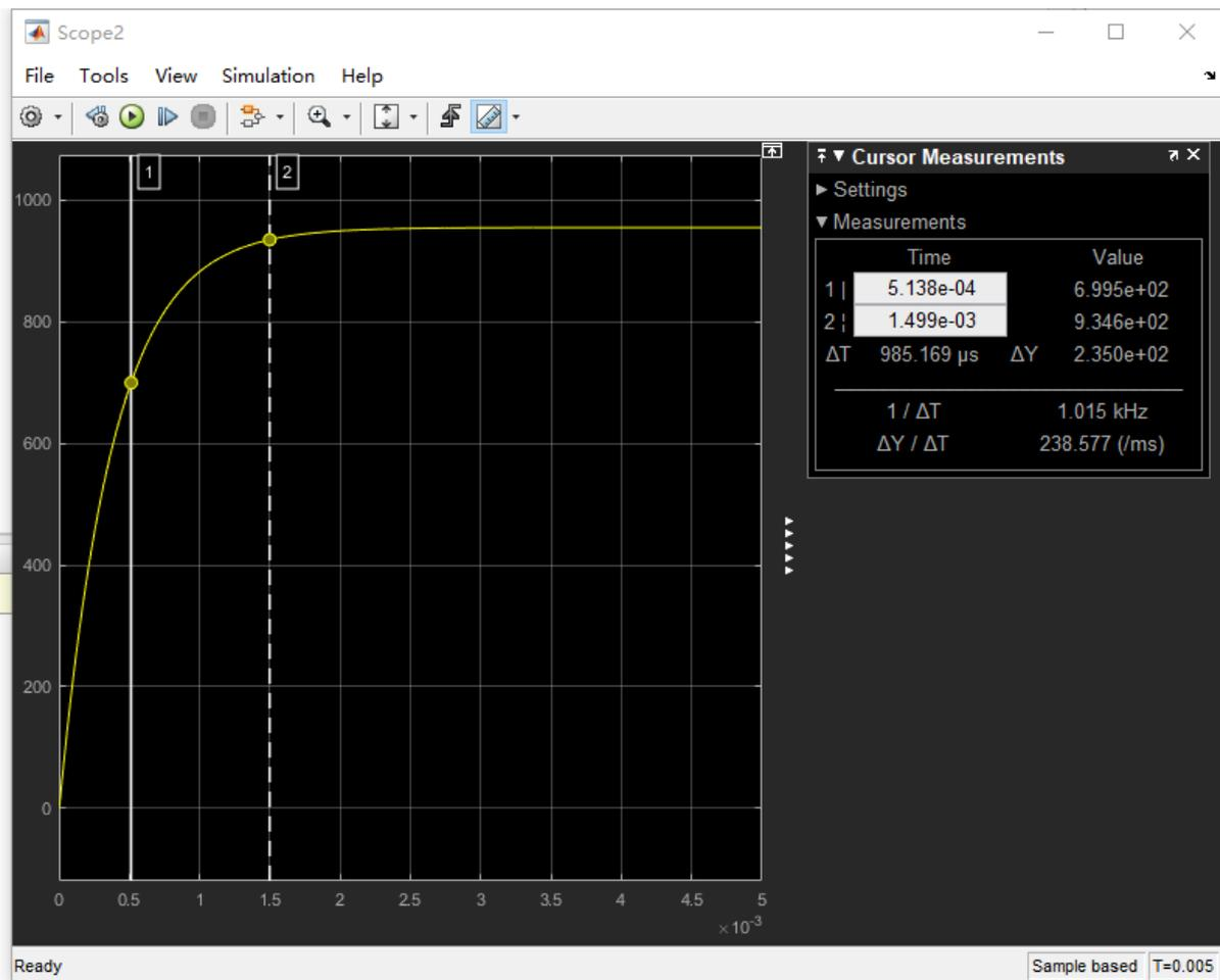
In the simplified model, the moment of inertia of the DC motor is designed to be very small, so the time to reach the target speed after the DC motor is powered on is very short. It means that the response speed approaches zero, and in actual system design, this response time will be much larger than this value.
