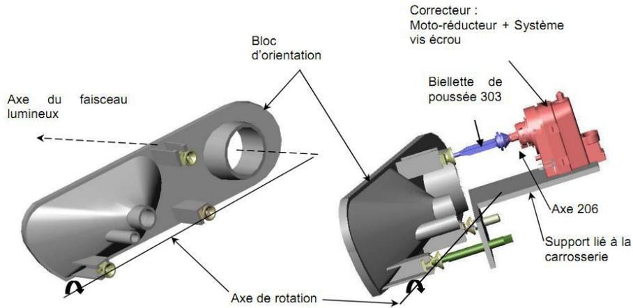
**Figure 4:** Kinematic chain of the headlight levelling system
