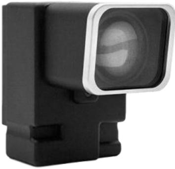
The technology is based on a monolithic LED, developed and produced by CREE, with 3,696 pixels to produce a high definition beam on the whole field. The main purpose of this module is to produce a high definition beam on the whole field. This module also makes it possible to do road marking for ADAS, but from 15 m in front of the car.
