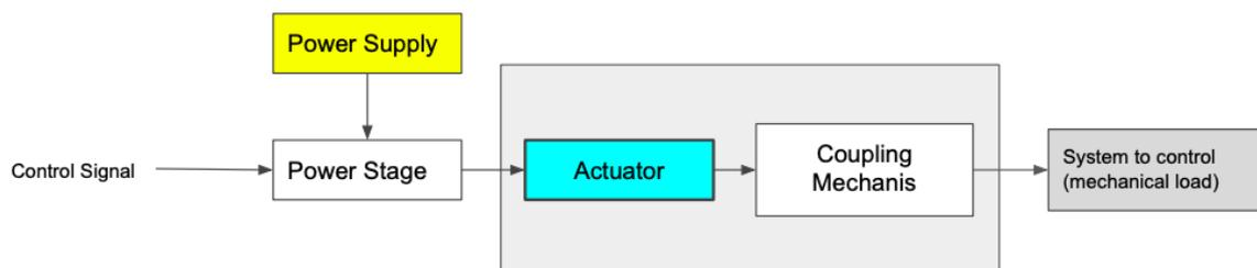
Figure 2 : Actuator in a mechatronic lighting system
