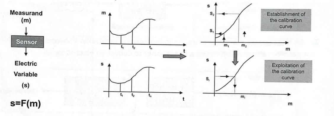
For easy exploitation reasons, we realized sensors or at least we use them in order to establish a linear relationship between the variations of the output signal and the variations of the physical variable to measure. This relationship is given by:
