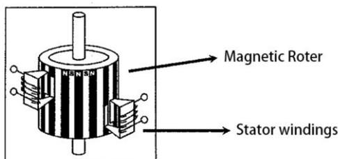
Step angle of a PM stepper motor:  $N_{ph} = \text{Number of equivalent poles per phase} = \text{number of rotor poles}$
