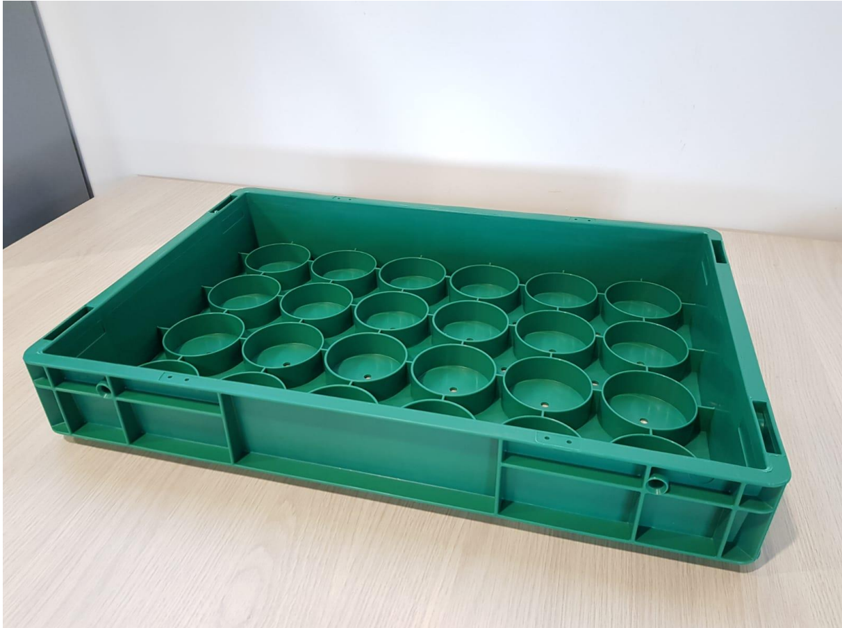
Figure 24 Standard holding box (engine pistons)
