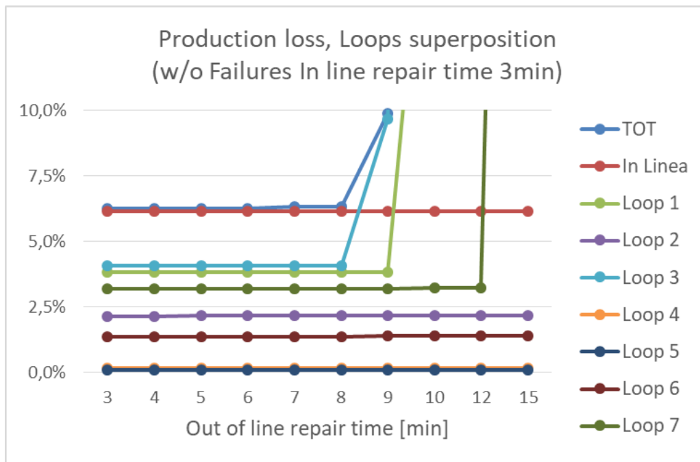
Figure 47 Production loss, loops superposition (Experiment without failures, 3min in line repairing time) ZOOM
