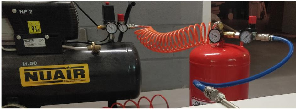
Figure 2.27: Compressor and tank set up for validation tests
