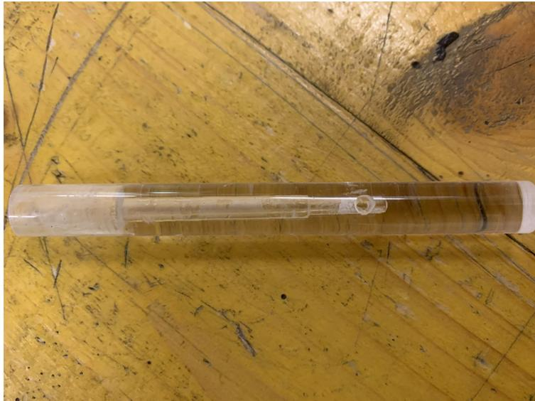
Figure 2.3: PMMA resonator used for validation tests
