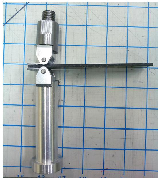
(b) Test fitting of the fixture components and a specimen off the machine
