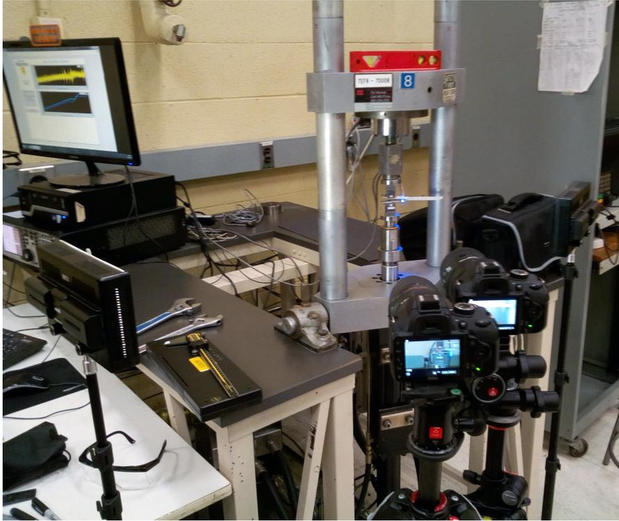
(a) Overview of the Small hydraulic frame setup. The compactness of the DSLR cameras allowed them to be placed side by side.
