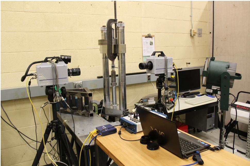
(b) The high-speed cameras were placed on the two sides of the specimen; two LED light fixtures were used to obtain high-contrast imagery.
