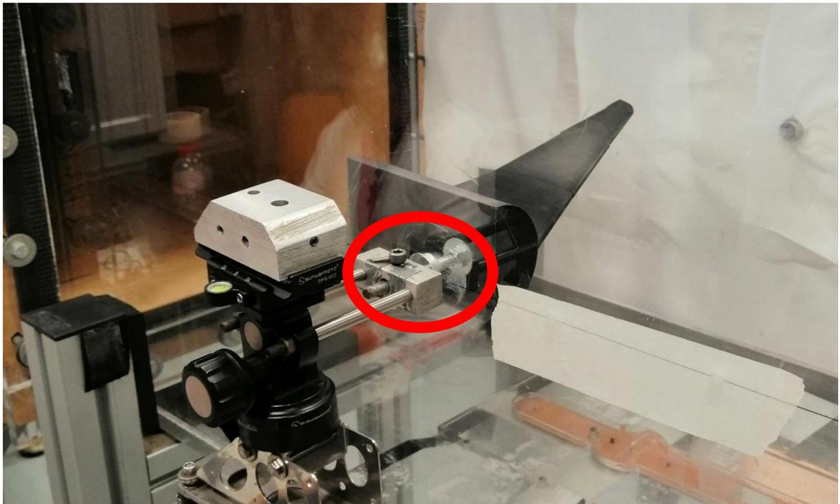
Figure 15 - Particular of the suspension system
