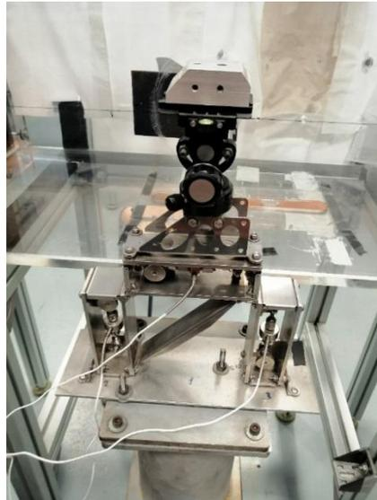
Figure 19 - Balance with gauges
