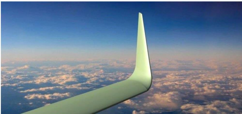
*Figure 7-Blended winglet configuration*
