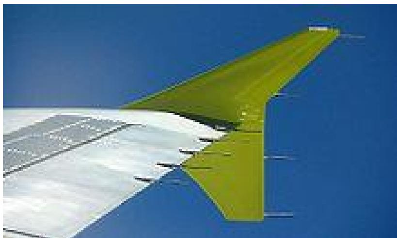
*Figure 9- Endplate winglet configuration*
