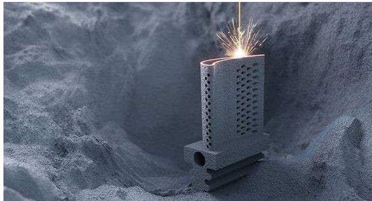
Figura 1: Additive manufacturing: paletta per turbina a gas [2]
