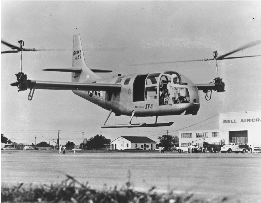
**Figure 1.4:** Photograph of the Bell XV-3 in helicopter mode
