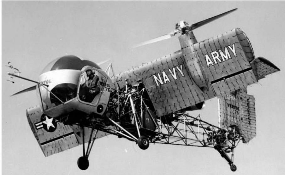
**Figure 1.5:** The Vertol Model 76 tilt-wing aircraft (Reference [12])
