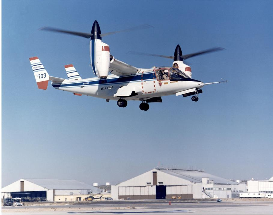
**Figure 1.7:** The XV-15 in helicopter mode during a test flight at the NASA Dryden Flight Research Center in 1980 (Courtesy of NASA)
