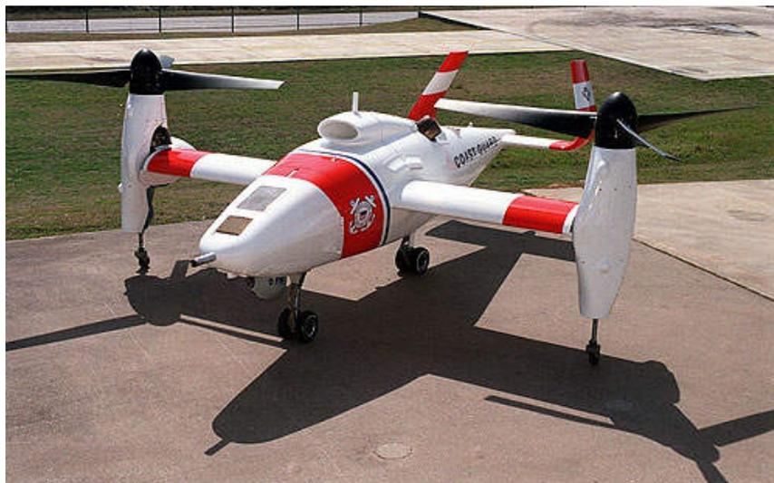
**Figure 1.13:** The Bell Eagle Eye tilt-rotor UAV
