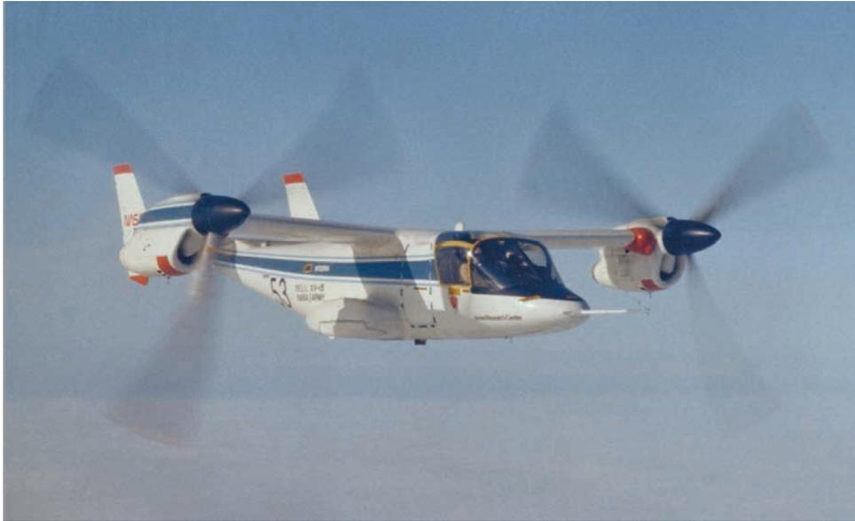
**Figure 2.1:** The XV-15 Tilt Rotor Research Aircraft flying in airplane mode (Reference [12])
