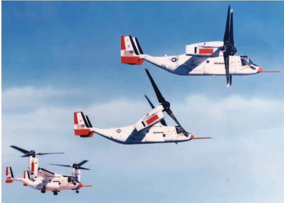
**Figure 1.2:** Collage showing the V-22 Osprey (*left to right*) in helicopter mode, during in-flight conversion and in airplane mode (Reference [12])
