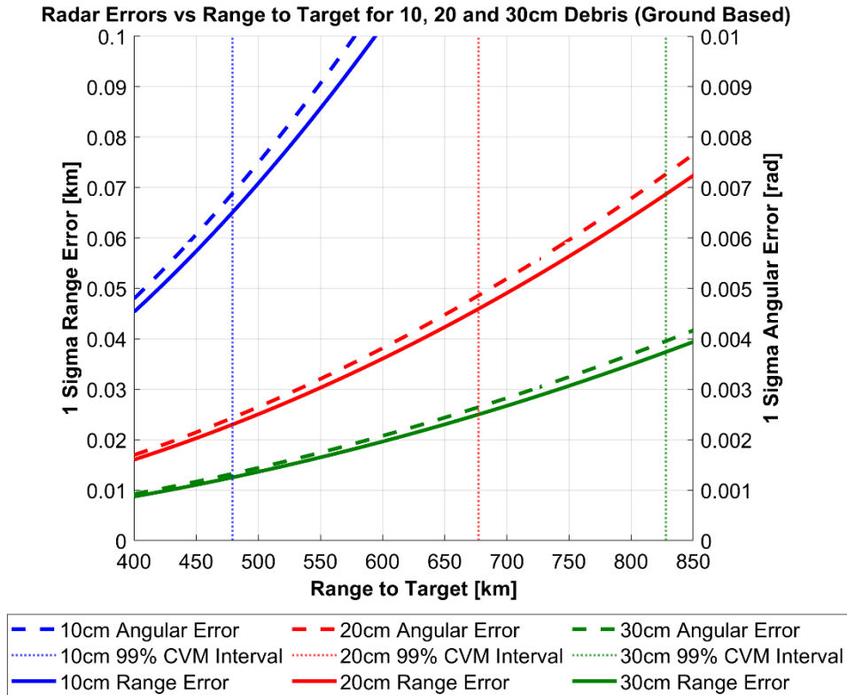
Figure 38. Ground Based Radar range and angular errors as a function of range to target
