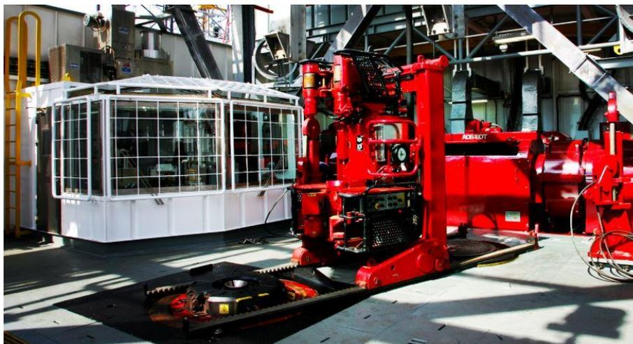
**Figure 10-** shows the iron rough neck device by varco inc
