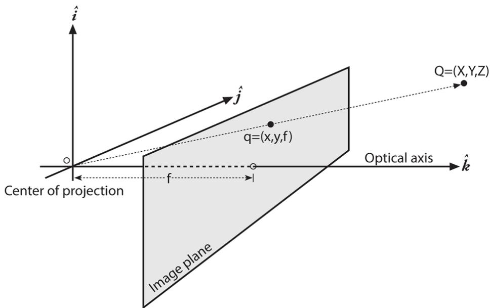
Figure 10: Rearranged pinhole camera model. ©[1]
