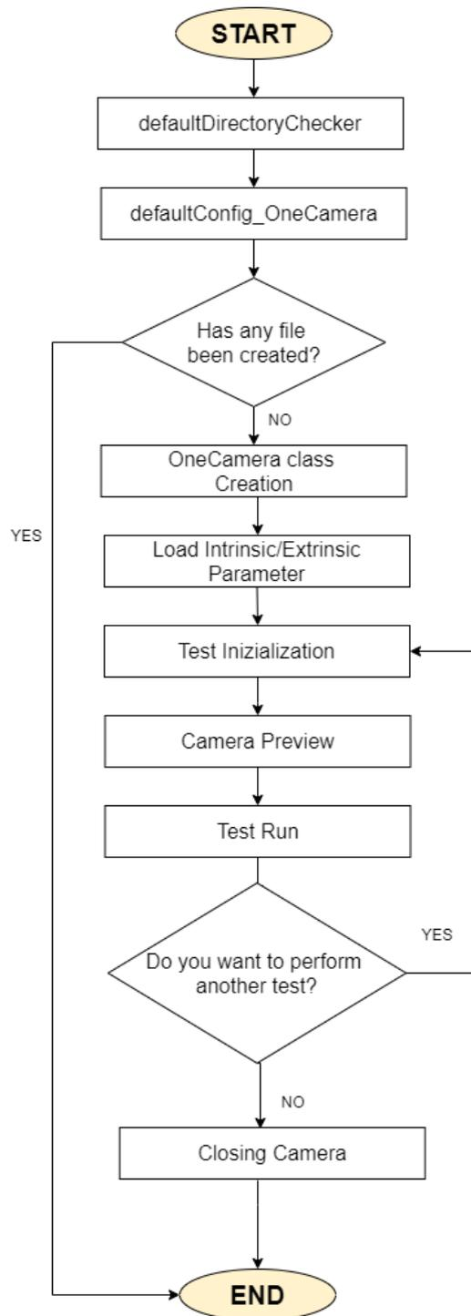
Figure 43: *LocSys\_OneCamera* flowchart
