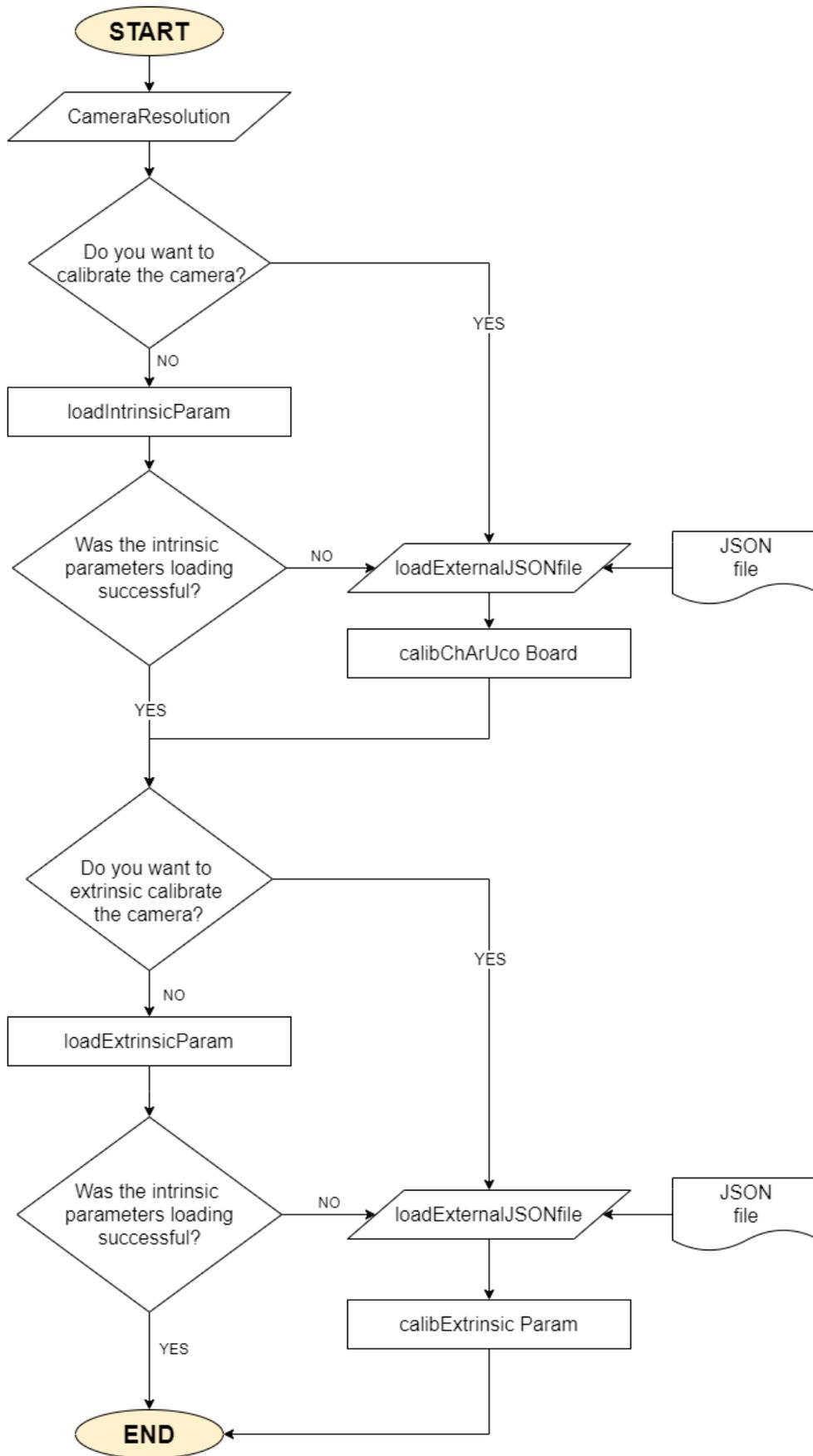
Figure 40: loadCalibParam OneCamera method flowchart
