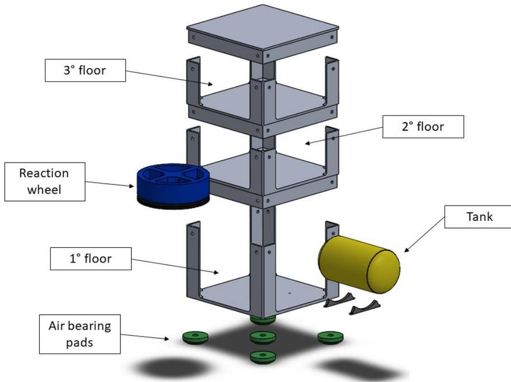
Figure 6: FTS exploded view
