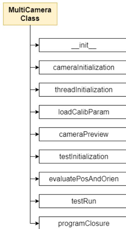
Figure 44: MultiCamera class methods
