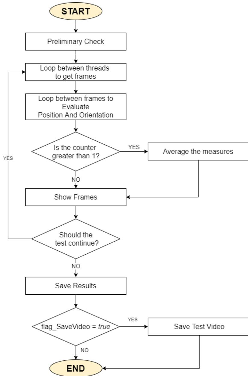
Figure 49: testRun MultiCamera method flowchart
