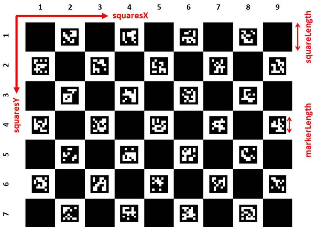
Figure 32: ChArUco board geometry
