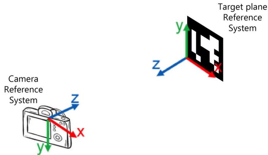
Figure 58: Camera and Marker reference systems
