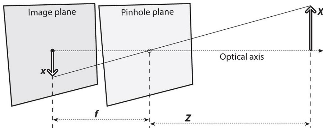
Figure 9: Pinhole camera model. ©[1]
