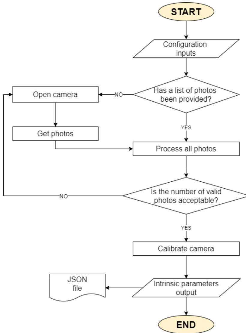
Figure 30: calibChArUcoBoard method flowchart
