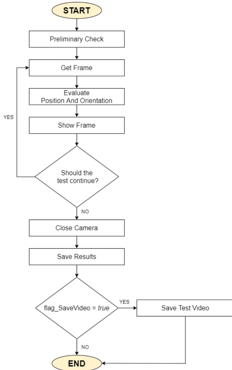
Figure 42: *testRun* method flowchart
