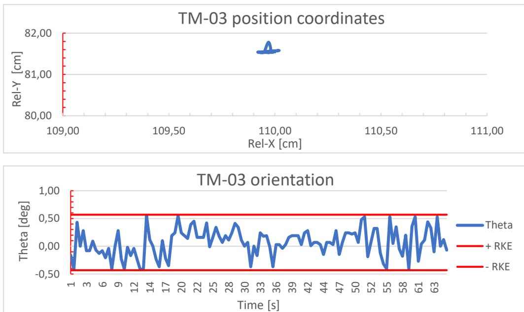
Figure 84: TM-03 position and orientation results
