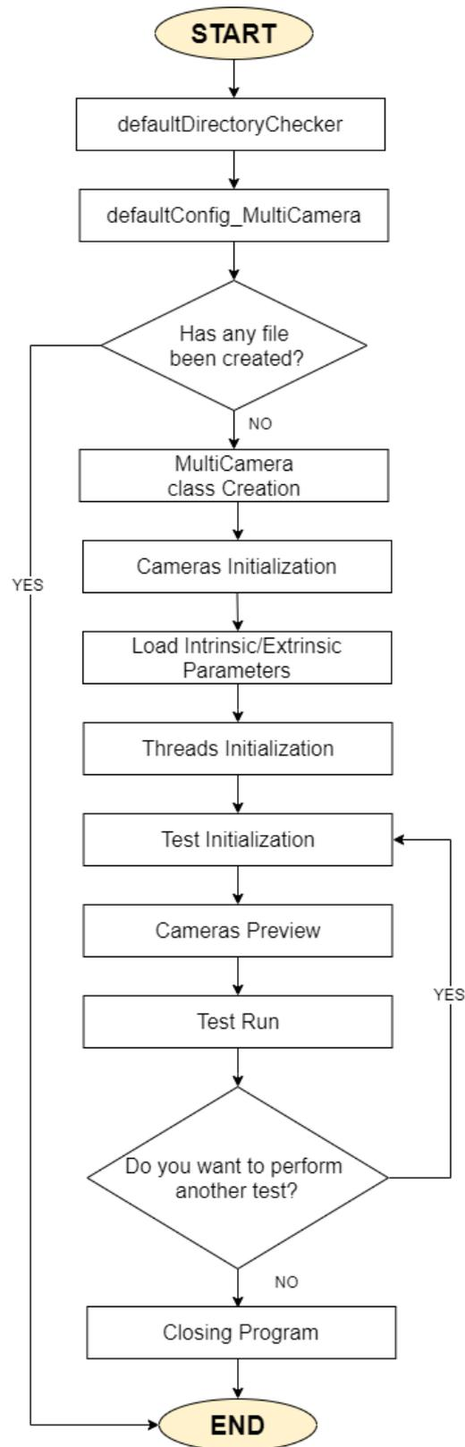
Figure 50: LocSys\_MultiCamera flowchart
