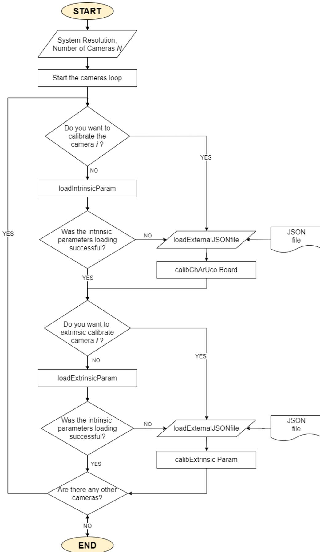
Figure 48: loadCalibParam MultiCamera method flowchart
