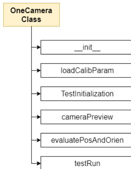
Figure 38: OneCamera class methods
