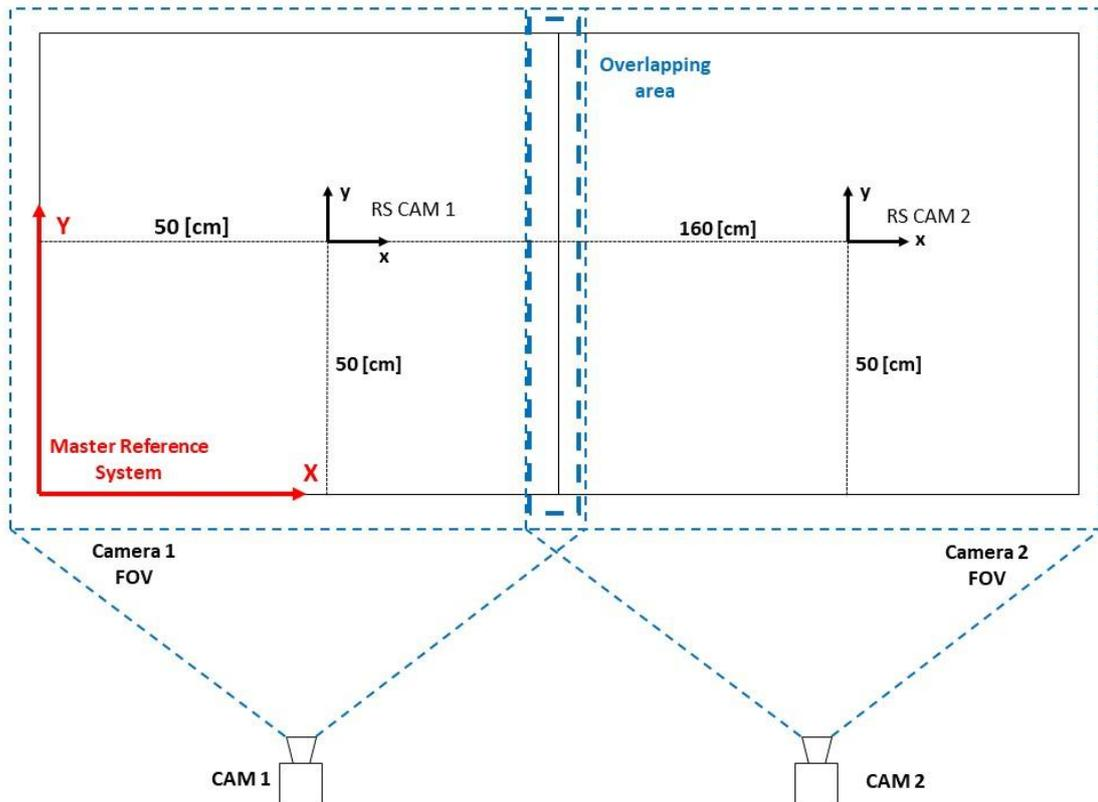
Figure 80: MultiCamera test configuration
