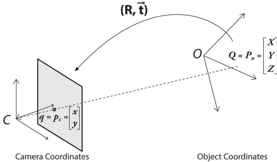
Figure 13: Camera and object coordinate frame relationship. © [1]
