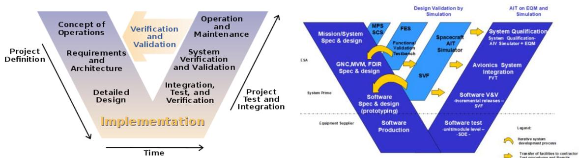
Figure 3: V-model and multiV-model comparison ©ESA
