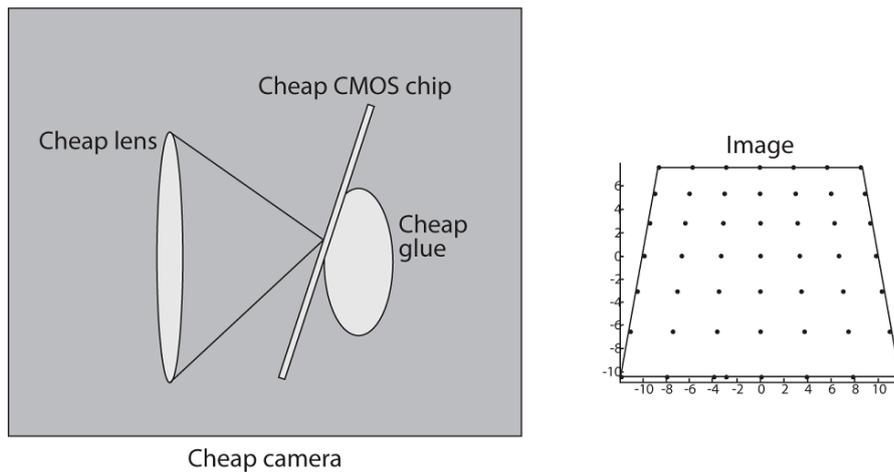
Figure 12: Tangential distortion. ©[6]
