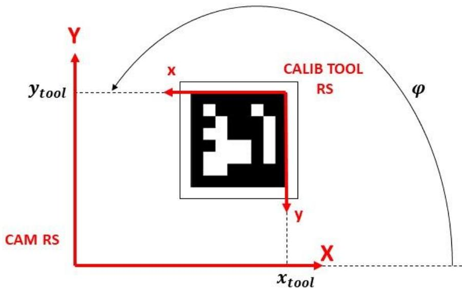
Figure 57: 3D calibration tool RS and camera RS relationship
