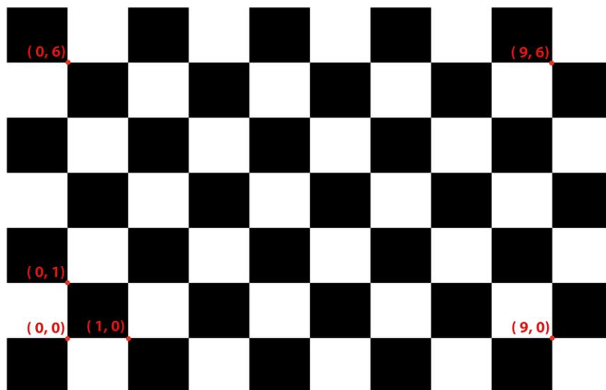
Figure 16: Chessboard calibration pattern
