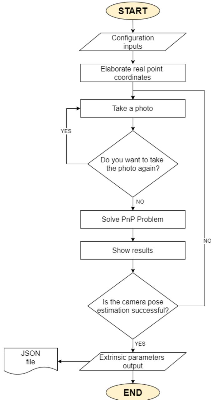
Figure 36: calibrExtrinsicParam method flowchart
