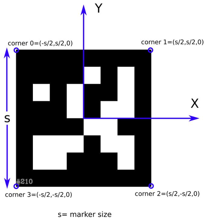
Figure 15: ArUco relative coordinate system. ©[9]
