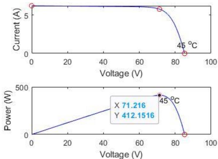
External Temperature has a significant effect on the power production of solar cells. High temperature has a reversal effect on the production of solar panel as we can see the graph, the total power produced is 412.15 watt when the external temperature is 45°C. The total energy production for a single day with external temperature 45°C is calculated as follows if the sunshine for at least 6 hours.
