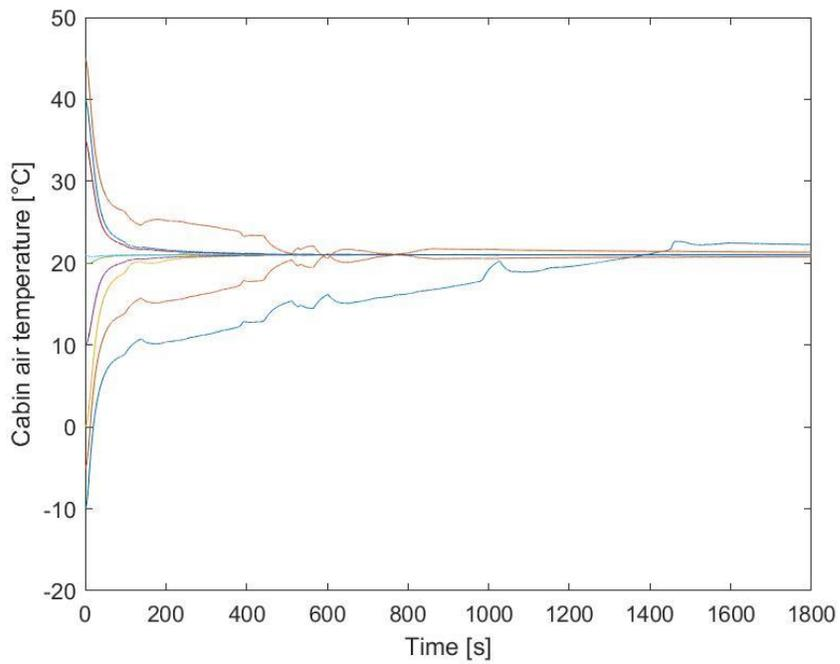
Simulation of cabin temperature for external temperature values equal to [-10 -5 0 10] requires a heating phase of the simulation model, while values [35 40 45] external temperature conditions simulated in this model require the cooling state of the HVAC system. The graph is showing the condition air temperature of the vehicle inside the cabin for the described external temperature values.
