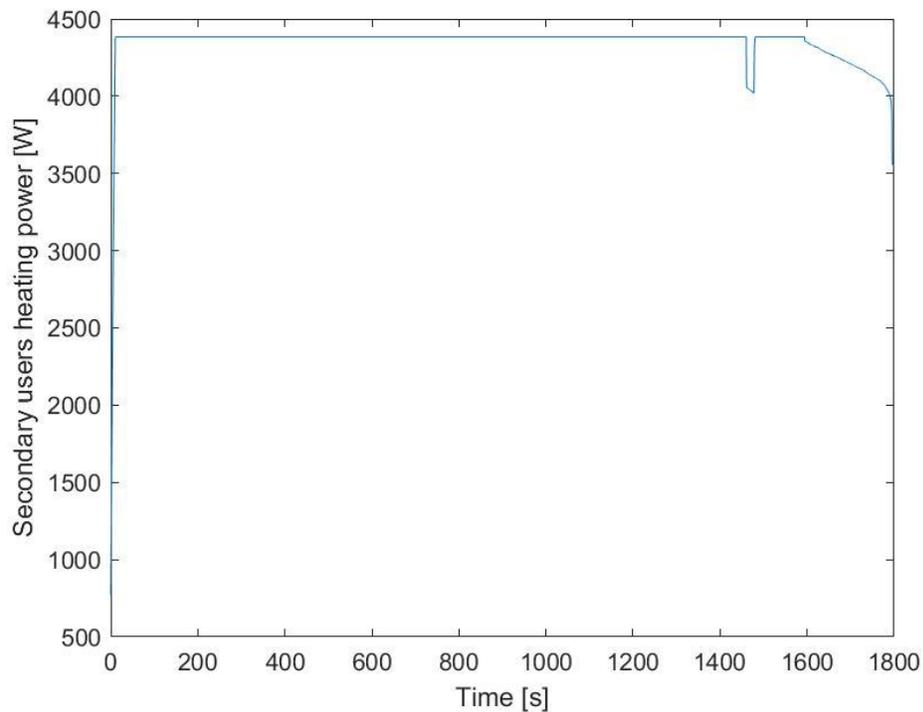
Extreme external weather conditions have a great impact on power consumption; As the graph shows, the PTC heating system uses its total available power to bring the cabin temperature to the desired set value.
