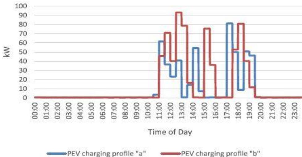
Fig. 2. PEV charging profiles considered in this study.
