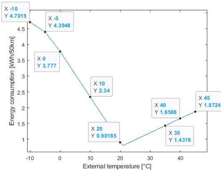
Graphical representation of the amount of energy required for the HVAC system of the car for 50 km drive on cloudy day scenario with respect to different external temperature conditions illustrate that heating vehicle consumes more energy compare to the sunny day scenario, while for cooling the electric vehicle cabin the amount of energy expended on a cloudy day is less than on a sunny day.
