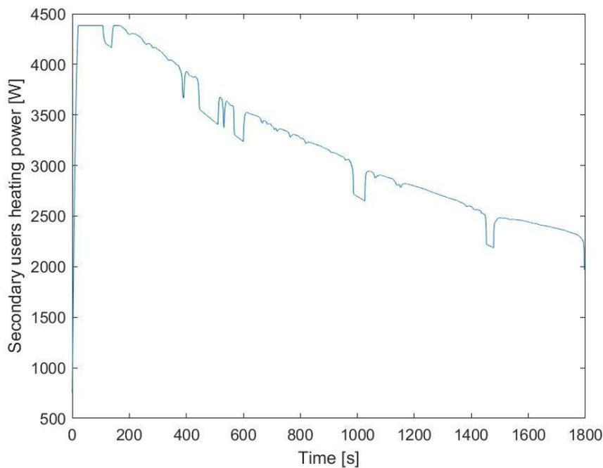
Power demand decreases as the value of external temperature, and the desired value temperature difference decreases. The amount of energy demand is much less as compared to external temperature conditions of -10°C and -5°C.
