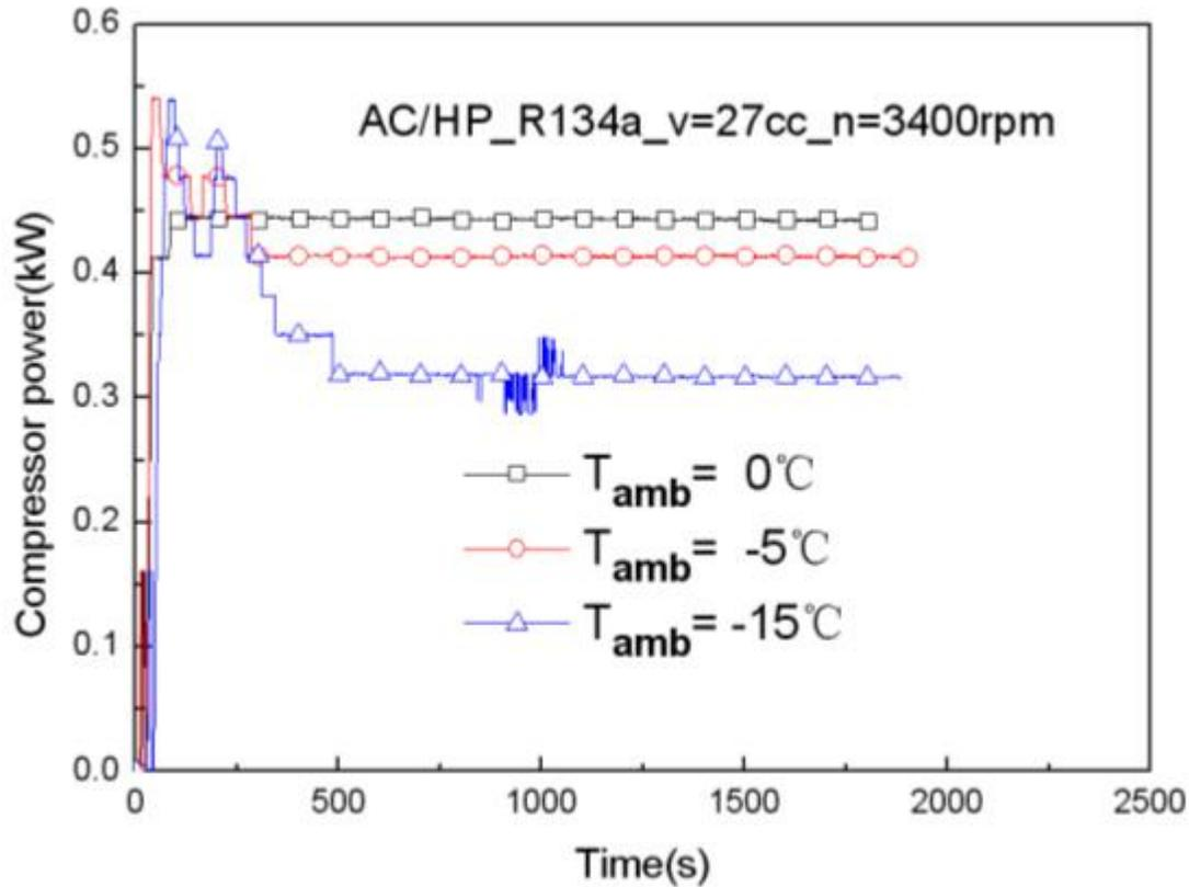
Figure 10 Variation of the compressor power consumption
