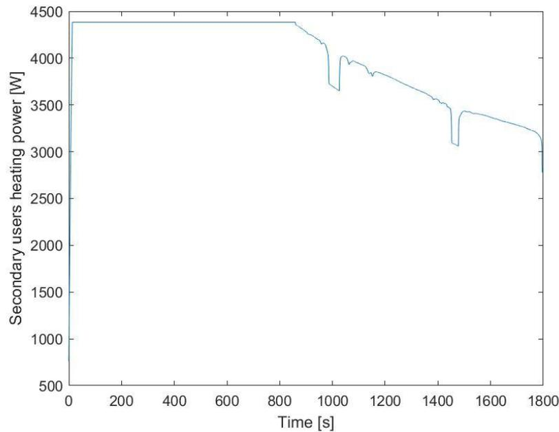
The power requirement for external temperature conditions at -5°C decreases after 700 seconds of a simulation showing that the cabin temperature nearly reaches its desired value.
