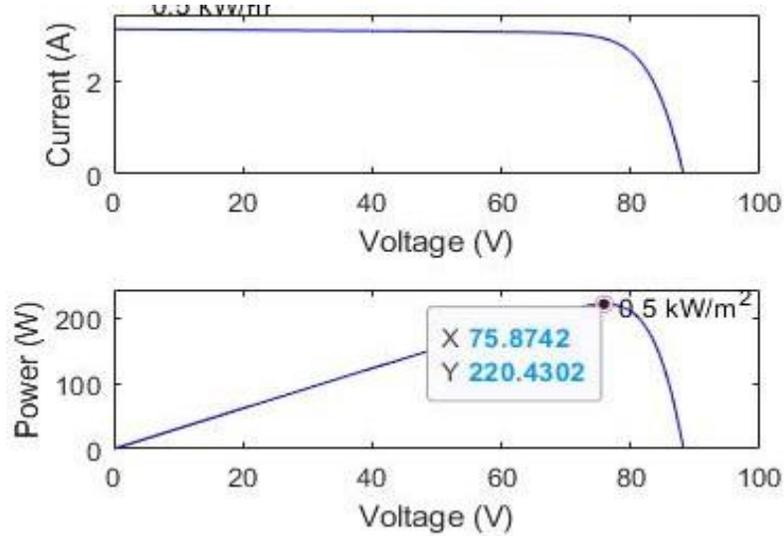
From the results, it is clearly shown that 220 watts are the maximum power we get on the output. If the sun shines for 6 hours a day, the Energy we can get Mathematically,
