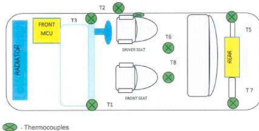
Figure 3 Thermocouples representation [35]
