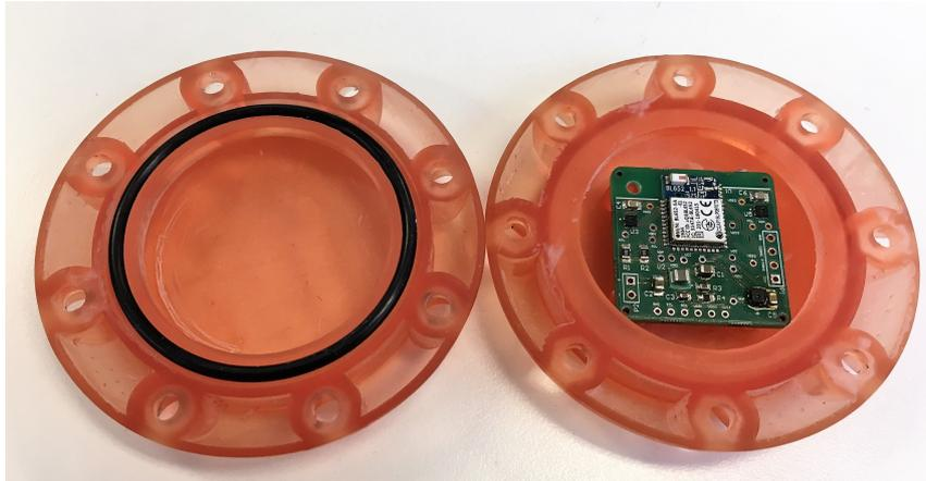
Figure 5.4: Photograph of package internal parts with PCB and o-ring.
