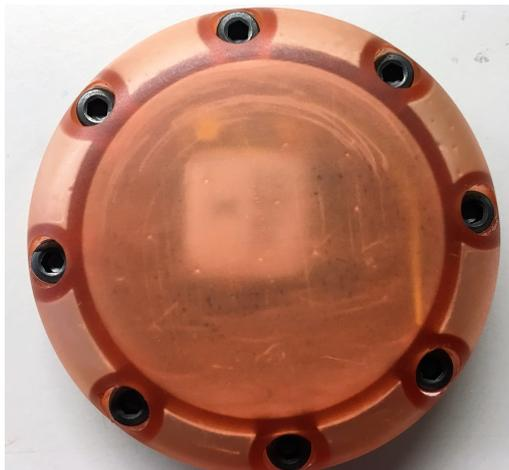
Figure 5.5: Photograph of the final sealed package with PCB and battery inside
