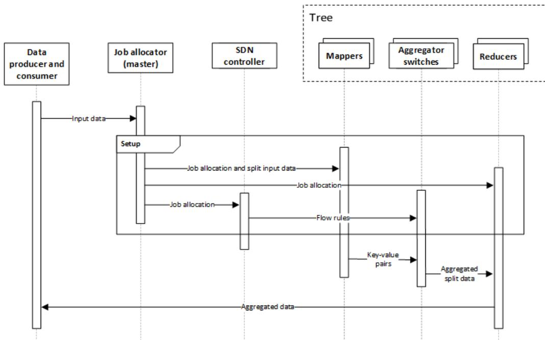
Figure 3.5. Messages exchanged during a Daiet [25] instance execution
