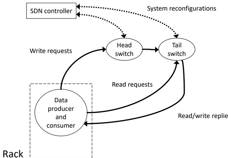
Figure 3.6. NetChain’s [13] basic topology and entities
