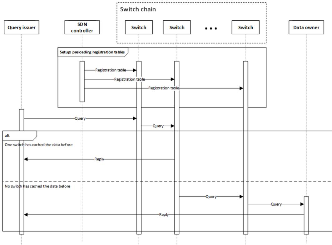
Figure 3.12. Messages exchanged during an IncBricks [17] instance execution
