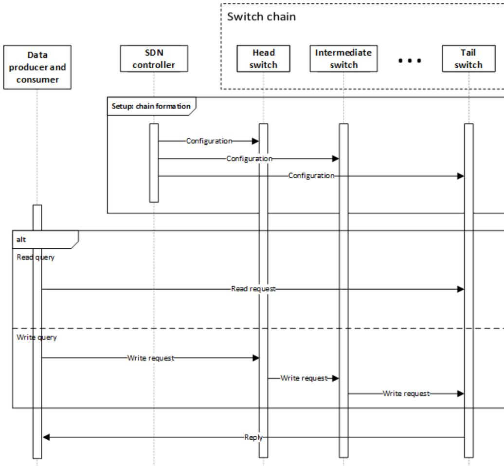
Figure 3.7. Messages exchanged during a NetChain [13] instance execution
