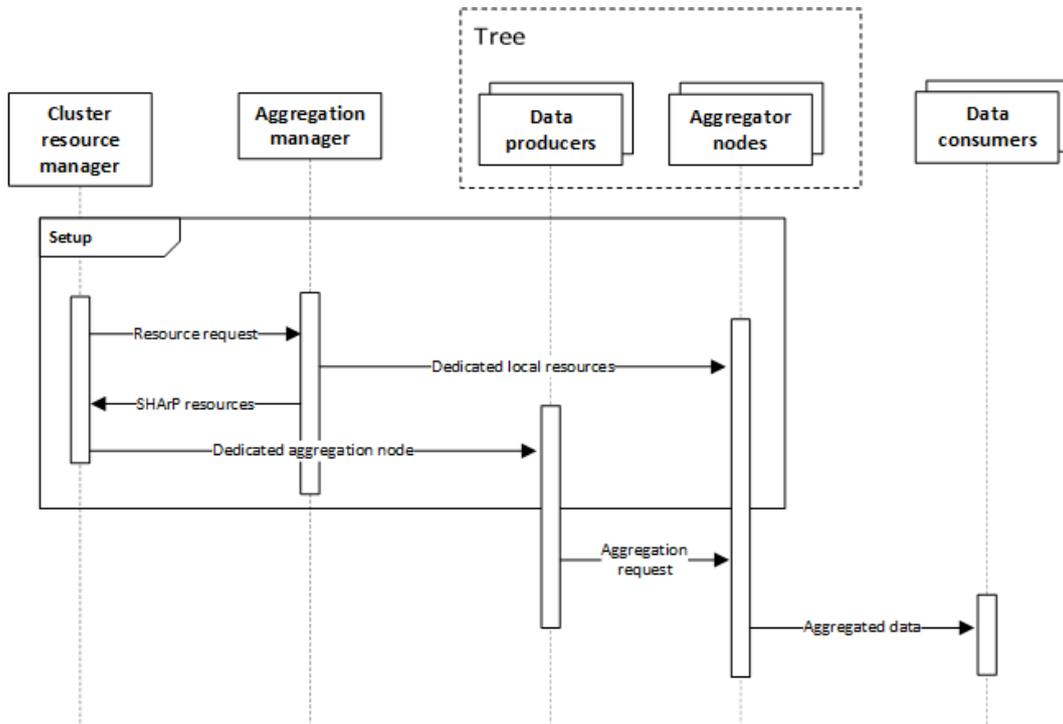
Figure 3.17. Messages exchanged during a SHArP [10] instance execution
