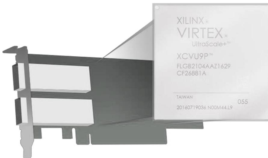
**Figure 4.2:** View of a PCIe development board based on a Xilinx Virtex Ultra-scale+ FPGA (Adapted from [31])
