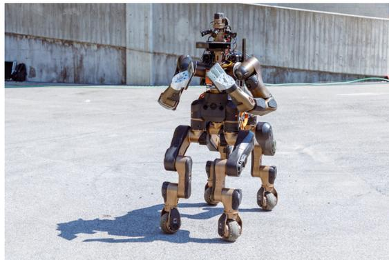
Figure 1.1: Centauro is a robot designed at the Italian Institute of Technology (IIT) that makes use of RGB-D sensors. Image from [52].
