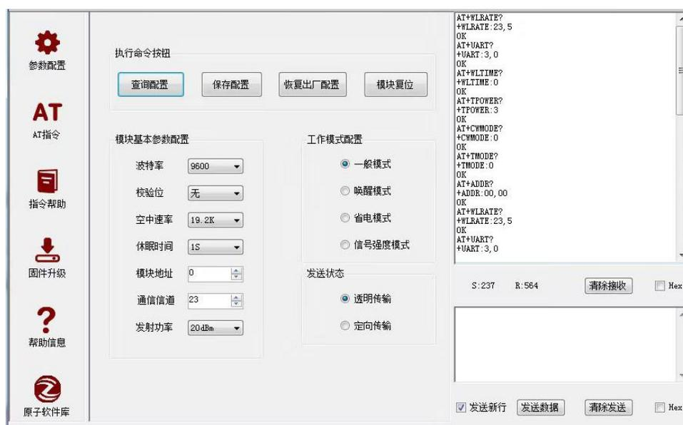
Figure 3.2.6.4 The configuration parameters of LoRa module
