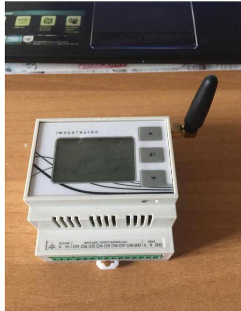
Figure 3.2.5.3 The final combination of D21G controller and LoRa module
