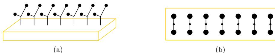
**Figure 1.11:** Molecular wire implementation: (a) a substrate, for example a gold nanowire, onto which molecules are placed, (b) top view.
