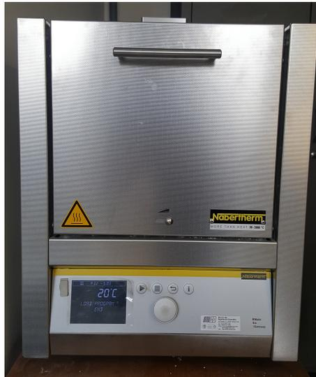
Figure 2.12: Sintering oven
