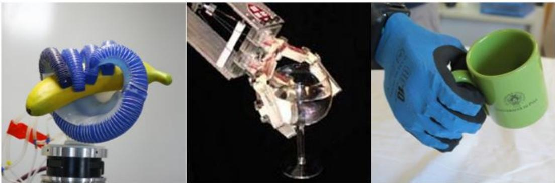
**Figure 2.2:** From the left: RBO Hand 2, SDM Hand, Pisa/IIT Soft Hand
