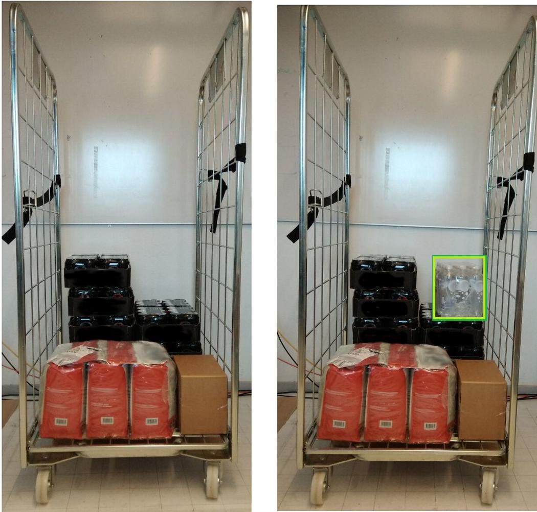
(a) A partially filled roller container with common goods: cans, a bag of pet food, and a box. (b) A new object (water bottles package) is placed automatically in the roller container.
