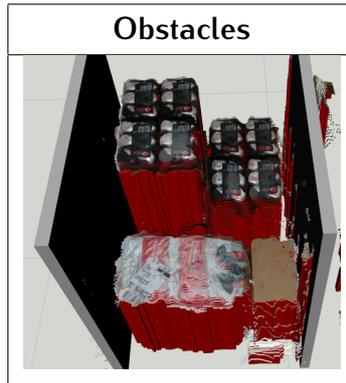
**Table 4.19:** Obstacle estimation (in red). In grey the obstacle volume of the roller container, its pose and volume is known.
