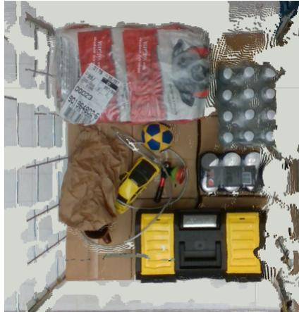
**Figure 3.8:** Point cloud acquired from the RGB-D camera showing the view of the robot over the placement volume.
