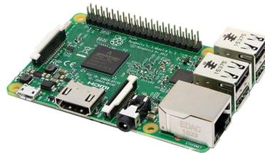
**Figure 3.6:** Raspberry Pi 3 Model B
