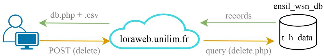
**Figure 5.5:** .csv file download and record removal: download.php, delete.php
