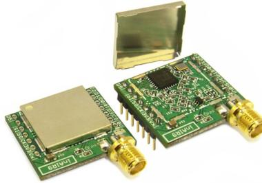
**Figure 3.5:** Wireless SX1276 LoRa module
