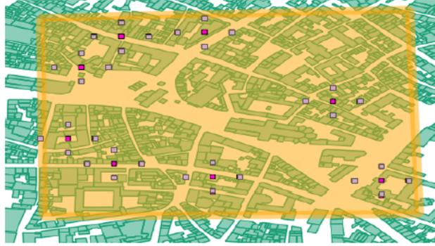
Figure 3.2: The considered suburban area of 0.3 km<sup>2</sup> (orange box) of the city center of Ghent, in Belgium, with macrocell Base Stations (purple points) and microcell Base Stations (pink points)
