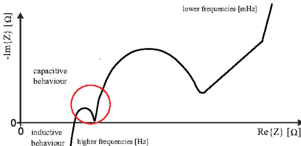
Figure 7 The behaviour of the battery's impedance with different frequencies.
