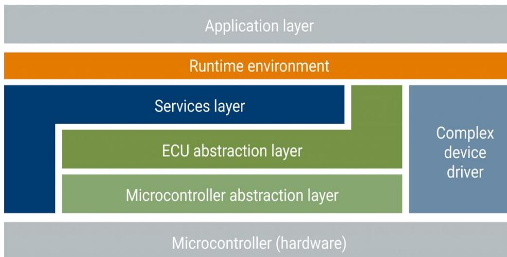
*Figure 14 AutoSAR layered architecture.*
