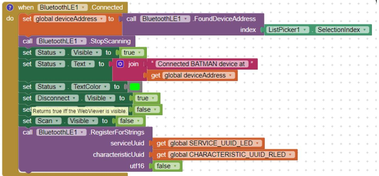
Figure 25 Bluetooth Low Energy block in the mobile application.
