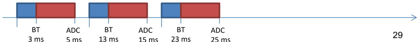
Figure 19 Scheduling of Adc thread (Red) and Bluetooth thread (blue)
