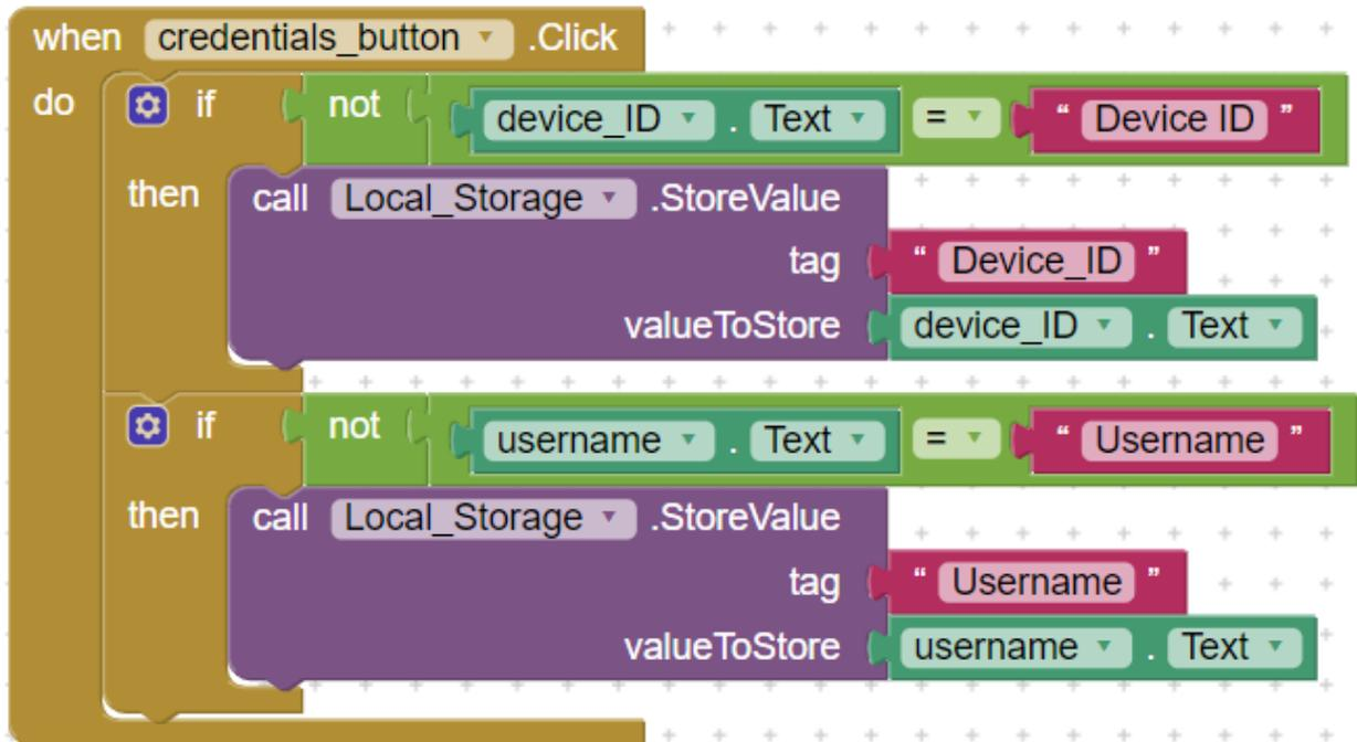
Figure 22 Credentials acquiring block in the mobile application.
