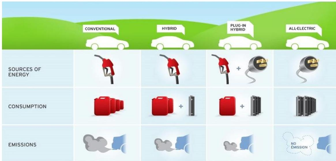
Figure 3 Comparison of the different types of electrical Vehicles.
