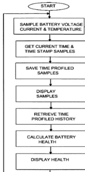
Figure 5 Flow chart of the processes performed by the patented device.
