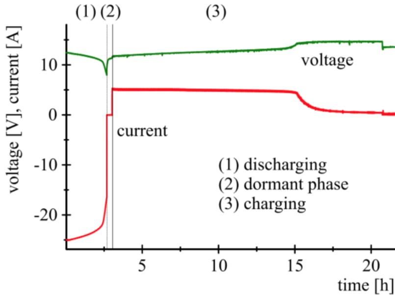
Figure 9 The three main intervals of analysis for the charging and discharging of the battery.
