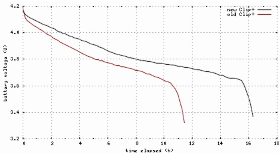
Figure 2 Battery voltage (V) discharge with time (hours).
