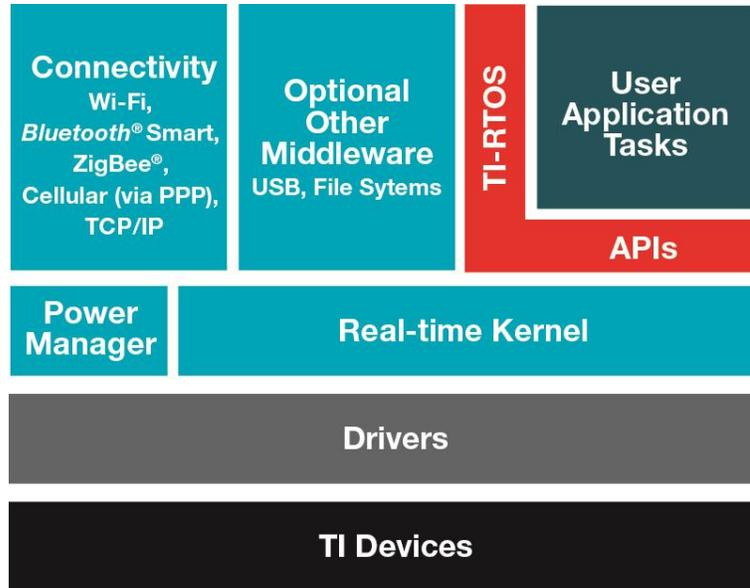
Figure 16. TI RTOS Components Layers
