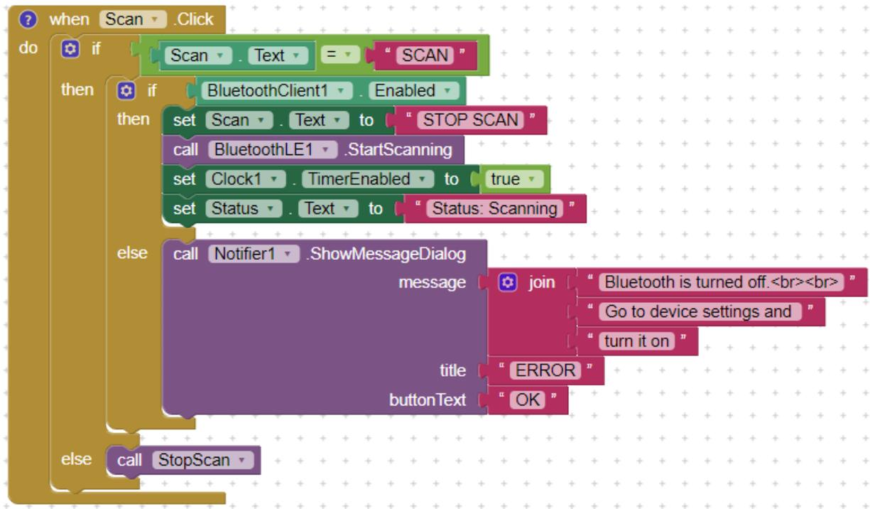
Figure 24 Scan block in the mobile application.
