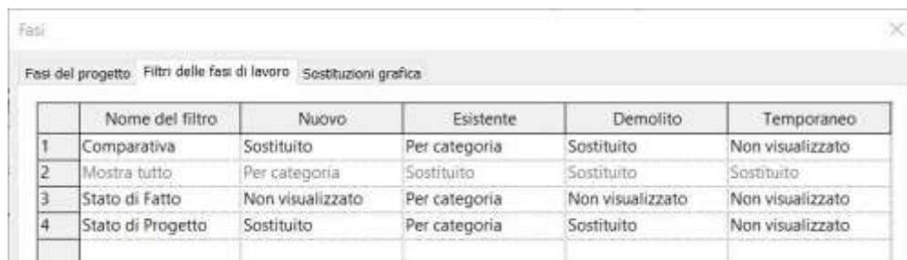
FIGURE 51: FILTRI DELLE FASI DI LAVORO - REVIT 2019
