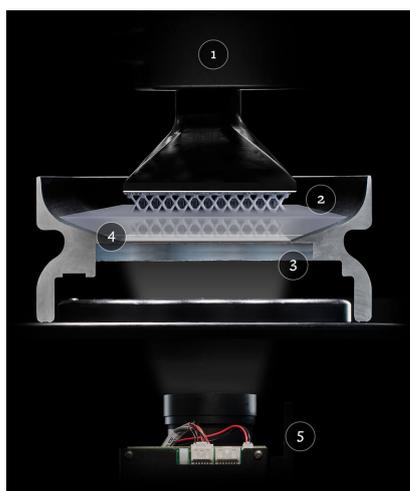
**Figura 2.3:** *Continuous Liquid Interface Production CLIP*
