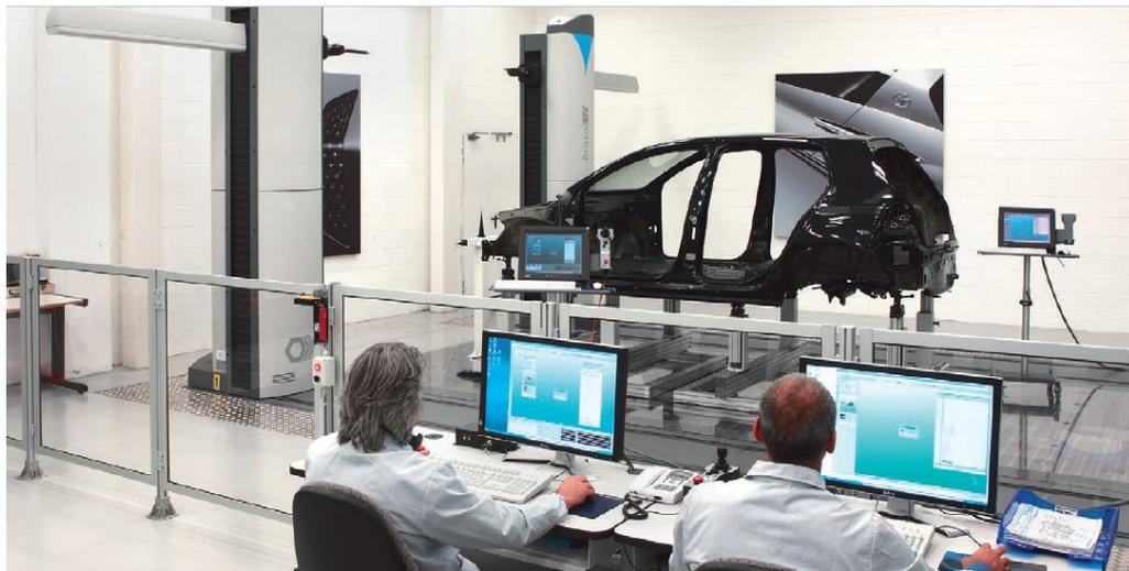
**Figure 6: Application of horizontal-arm machines**
