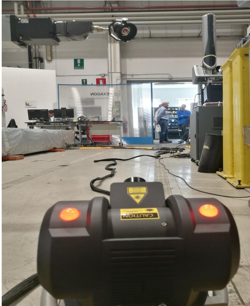
**Figure 18: LT locked-in to the reflector**
