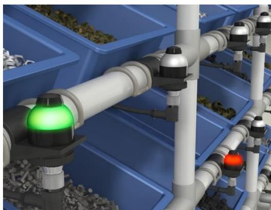
Figura 50 - Sistema logistico "pick to light"
