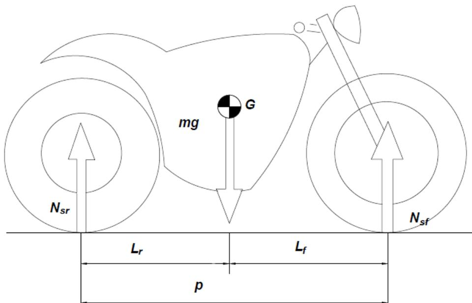
**Figure 1.7:** center of gravity longitudinal position
