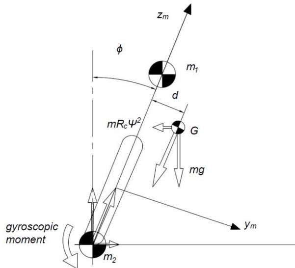
**Figure 1.18:** gyroscopic moment generated by the wheel rotational speed  $\omega_f$  and the yaw motion  $\psi$
