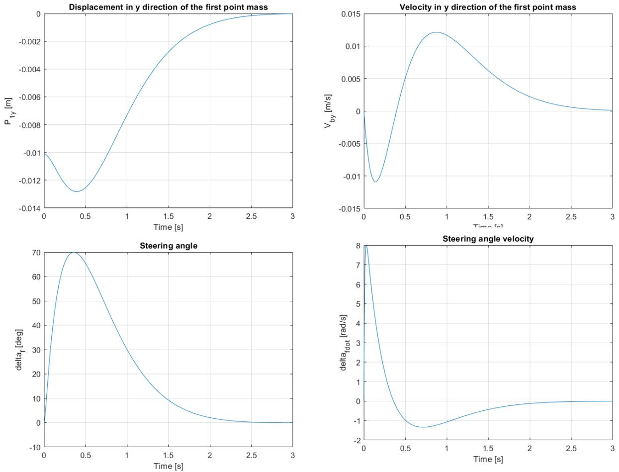
**Figure 3.17:** Results of the simulation with  $d = 0 [m]$  and  $t = 0.1621 [m]$  with the LQR control
