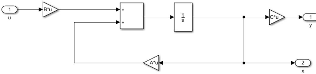
**Figure 3.5:** Simulink model representing the State-space system
