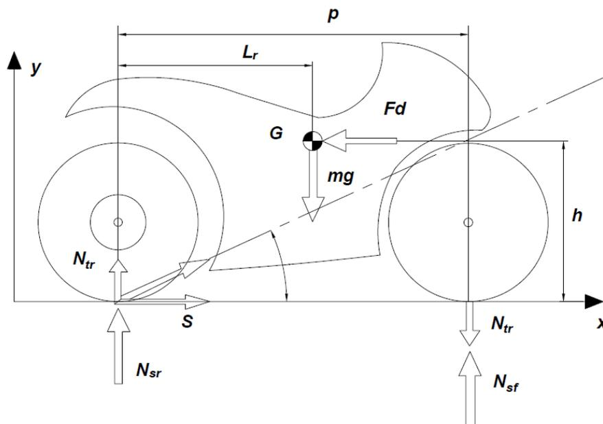
**Figure 1.10:** Load transfer angle
