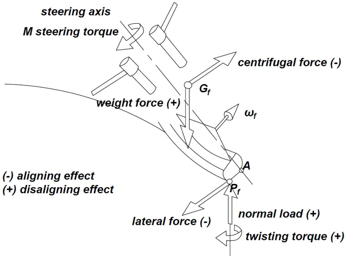
Figure 1.13: steering torque components
