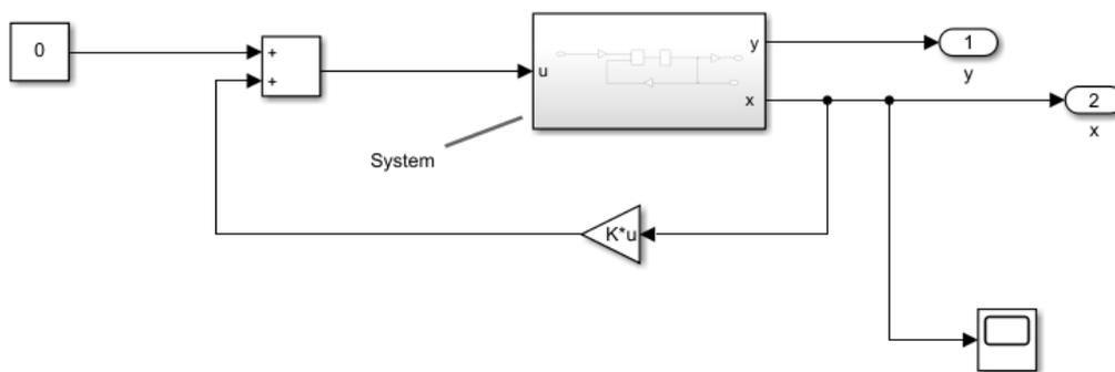
**Figure 3.7:** Simulink model of the system with a controller
