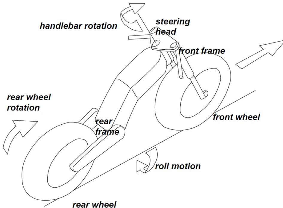
**Figure 1.1:** kinematic structure of a motorcycle
