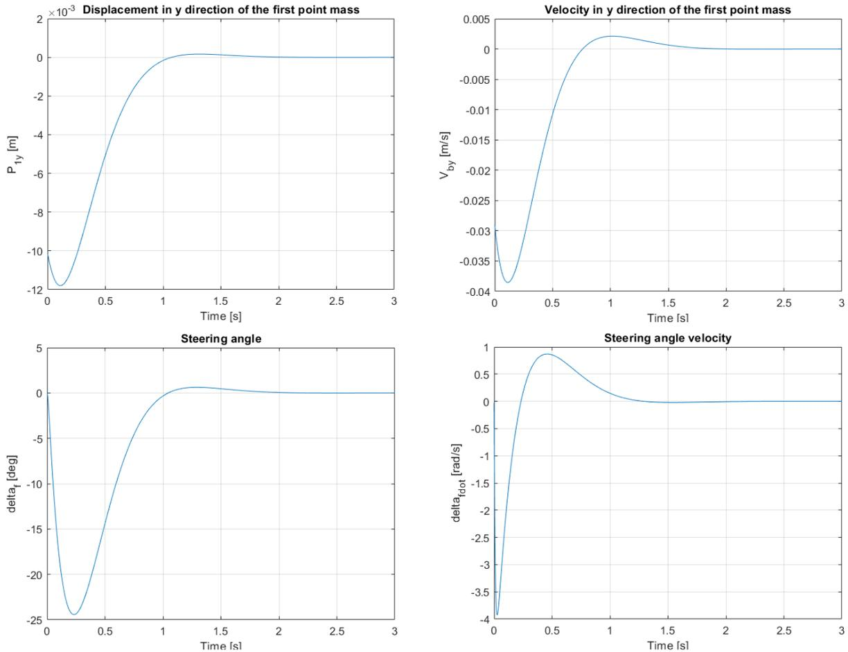
**Figure 3.25:** Results of the simulation with the roll gyroscopic effects generated at  $V_{ox} = 1 \left[ \frac{Km}{h} \right]$
