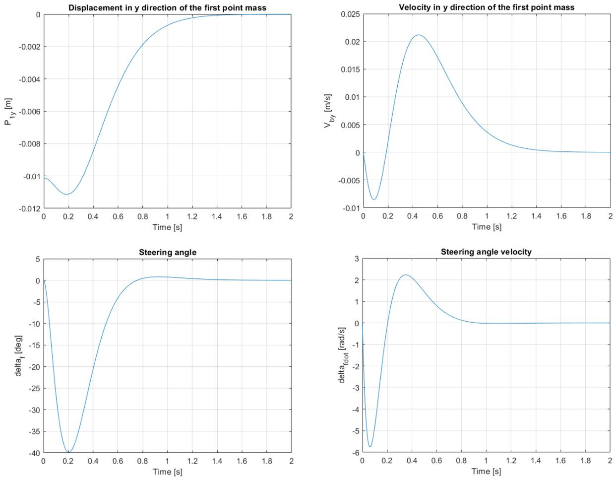
**Figure 3.13:** Results of the simulation with offset  $d = 0.1973 [m]$  and  $t = -0.060 [m]$ .
