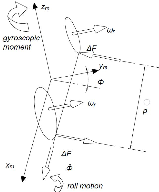
**Figure 1.23:** gyroscopic moment generated by the both wheels rotational speed  $\omega_f$  and  $\omega_r$  and the roll rate  $\dot{\phi}$  with the steering head locked
