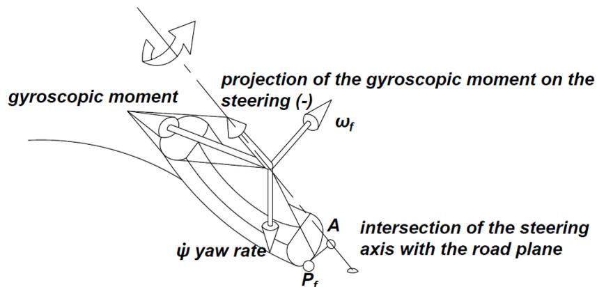
Figure 1.14: gyroscopic component of the steering torque
