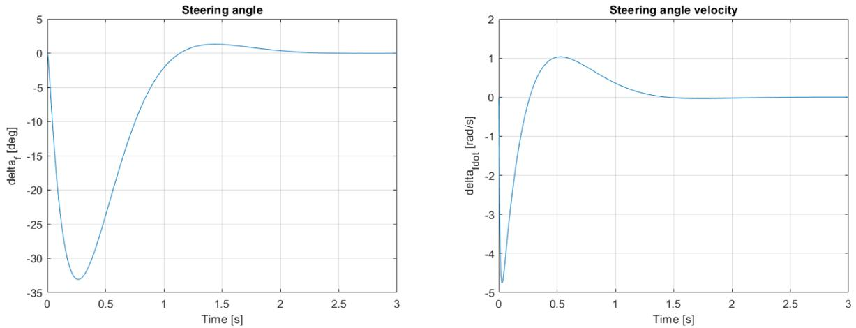
**Figure 3.18:** Results of the simulation with  $d = 0.1973$  [m] and  $t = -0.060$  [m] with the LQR control
