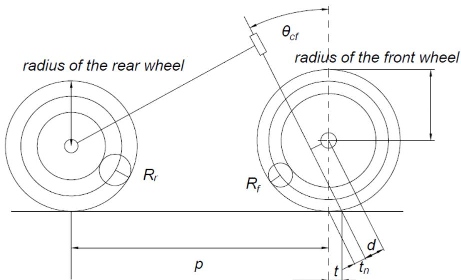
**Figure 1.2:** model of the geometry of a motorcycle
