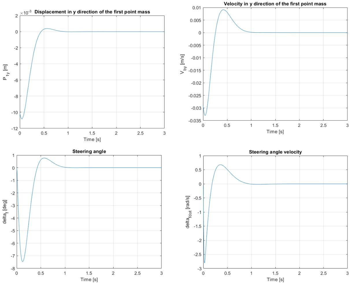
**Figure 3.27:** Results of the simulation with the roll gyroscopic effects generated at  $V_{ox} = 4 \left[ \frac{Km}{h} \right]$
