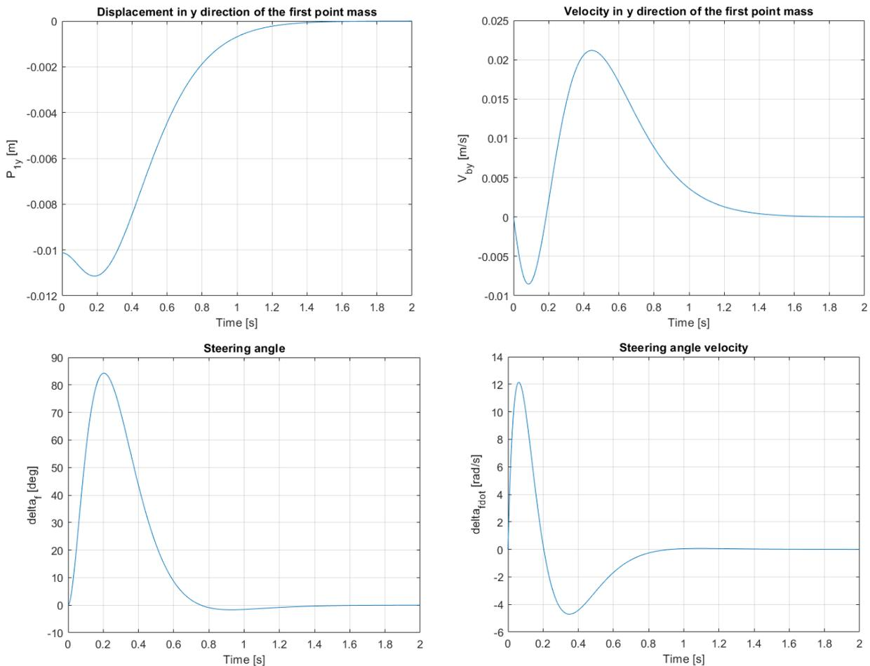
**Figure 3.9:** Results of the simulation with offset  $d = 0[m]$  and  $t = 0.1621 [m]$
