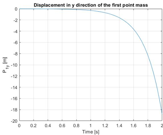
**Figure 3.6(a):** displacement of the first point mass in y direction, result of the simulation performed without a controller
