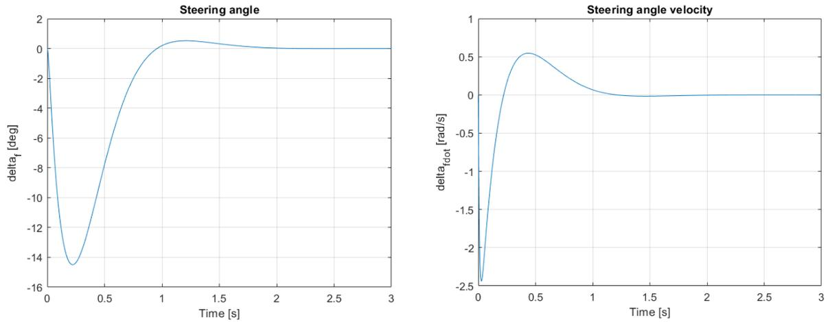
**Figure 3.19:** Results of the simulation with  $d = 0.1973 [m]$  and  $t = -0.060 [m]$  and  $V_{ox} = 1 [\frac{Km}{h}]$
