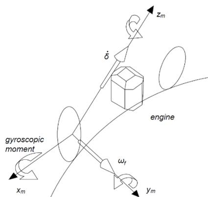
**Figure 1.24:** gyroscopic moment generated by the front wheel rotational speed  $\omega_f$  and the steering rate  $\dot{\delta}$
