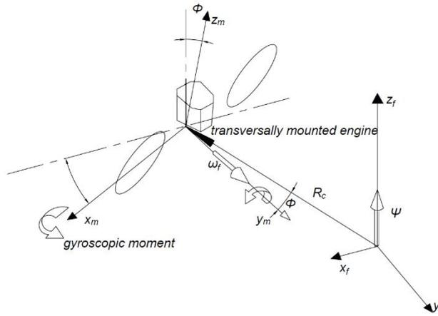
**Figure 1.20:** gyroscopic moment generated by the transversal engine rotational speed  $\omega_m$  and the yaw motion  $\psi$
