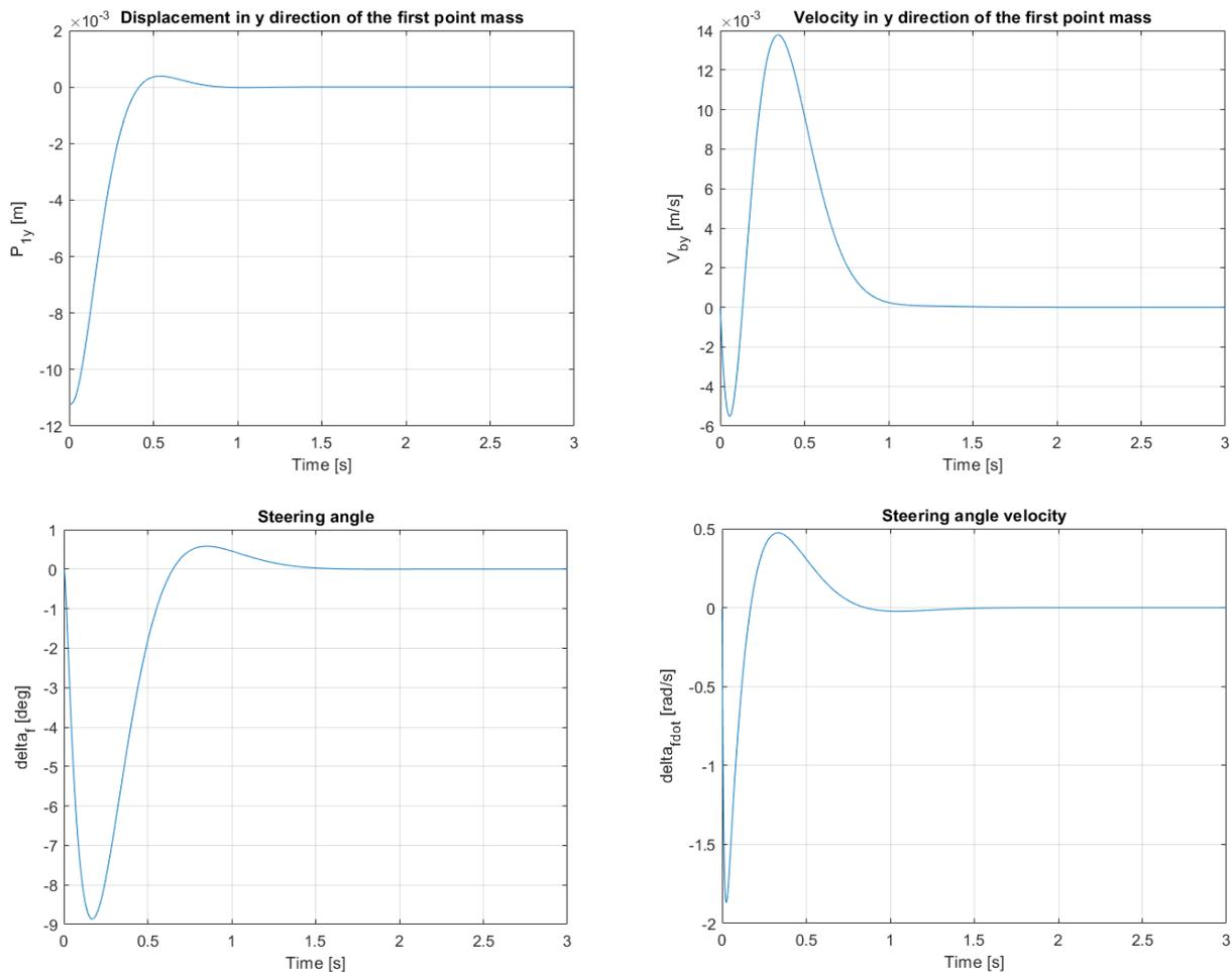
**Figure 3.24:** Results of the simulation with the yaw gyroscopic effects generated at  $V_{ox} = 4 \left[ \frac{Km}{h} \right]$
