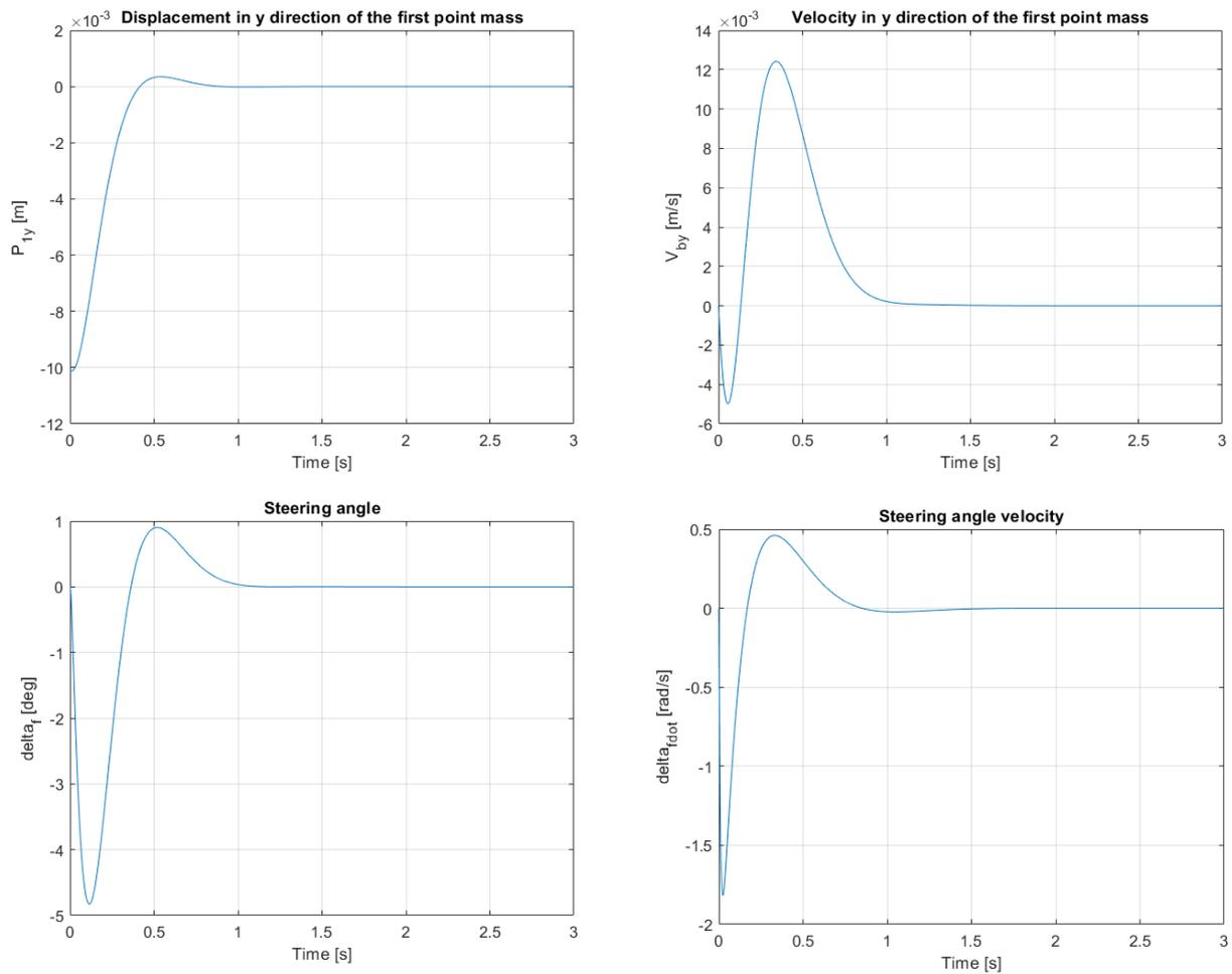
**Figure 3.21:** Results of the simulation with  $d = 0.1973 [m]$  and  $t = -0.060 [m]$  and  $V_{ox} = 4 [\frac{Km}{h}]$
