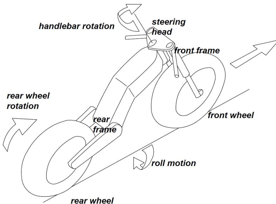
**Figure 1.1:** kinematic structure of a motorcycle
