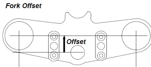
**Figure 3.12:** Typical triple clamp of a front fork with positive offset
