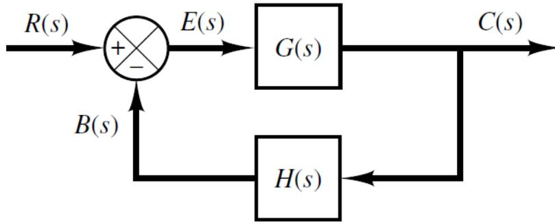
**Figure 2.3:** block diagram of a closed-loop system
