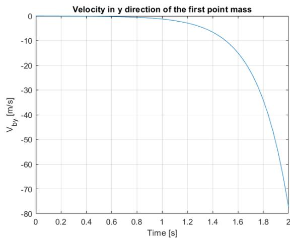
**Figure 3.6(b):** velocity of the first point mass in y direction, result of the simulation performed without a controller
