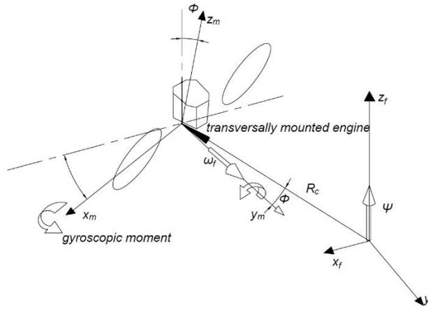
**Figure 1.20:** gyroscopic moment generated by the transversal engine rotational speed  $\omega_m$  and the yaw motion  $\psi$
