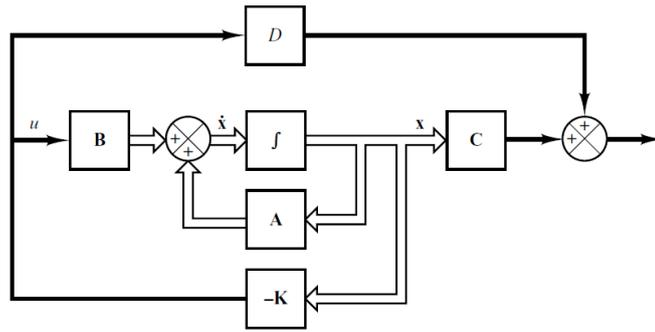
**Figure 2.4:** closed-loop control system with  $u = -Kx$
