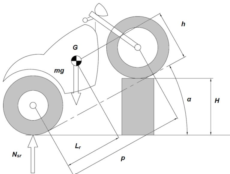
**Figure 1.8:** center of gravity height estimation
