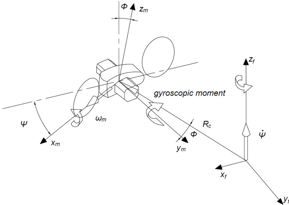
**Figure 1.21:** gyroscopic moment generated by the longitudinal engine rotational speed  $\omega_m$  and the yaw
