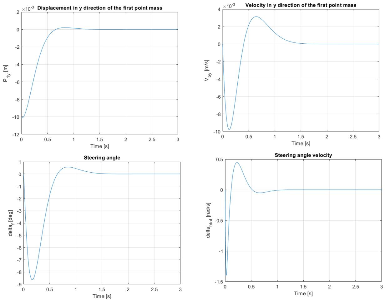
**Figure 3.20:** Results of the simulation with  $d = 0.1973 [m]$  and  $t = -0.060 [m]$  and  $V_{ox} = 2 [\frac{Km}{h}]$
