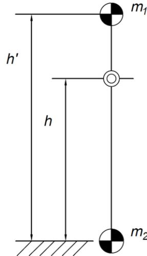
**Figure 3.2:** Approximate dynamics model of an equivalent two point mass system
