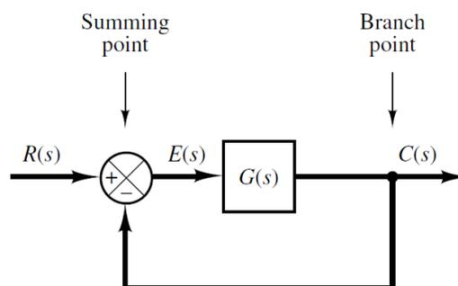
**Figure 2.2:** block diagram of a closed-loop system
