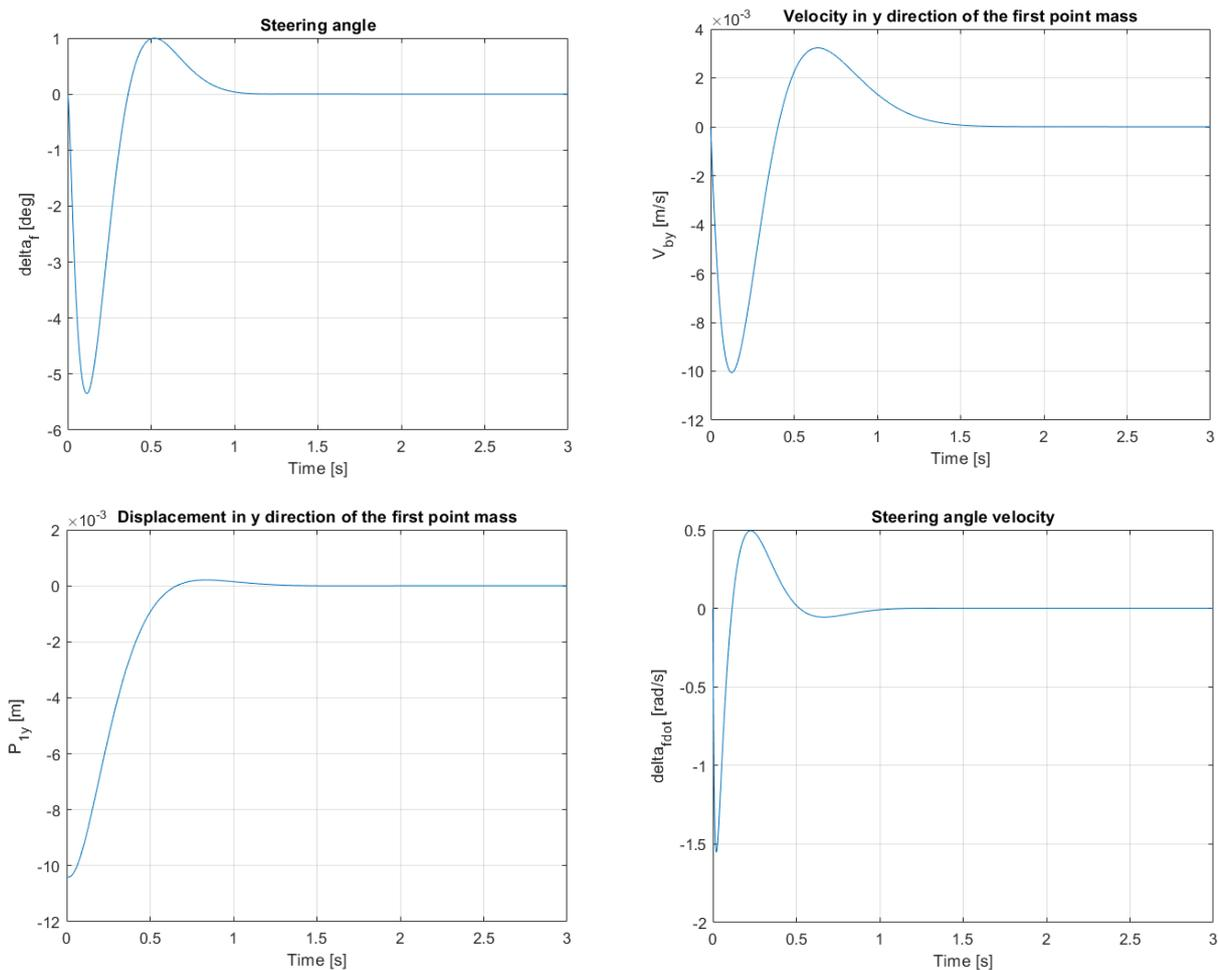
**Figure 3.23:** Results of the simulation with the yaw gyroscopic effects generated at  $V_{ox} = 2 \left[ \frac{Km}{h} \right]$
