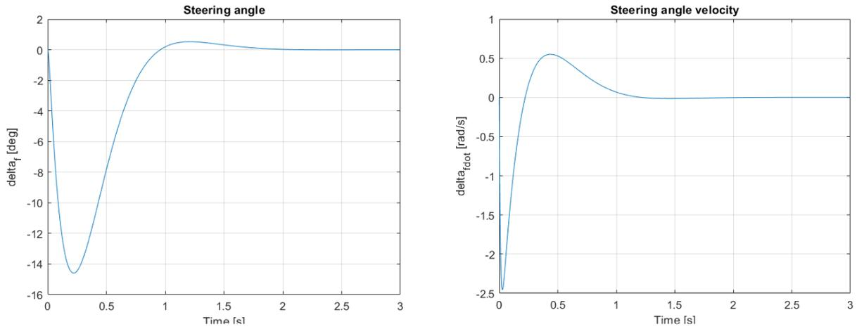
**Figure 3.22:** Results of the simulation with the yaw gyroscopic effects generated at  $V_{ox} = 1 \left[ \frac{Km}{h} \right]$
