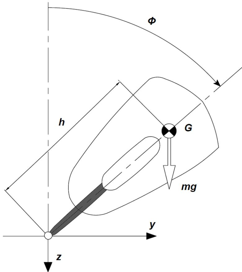
**Figure 1.15:** capsizes model of the motorcycle with thin disk wheels
