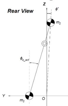
**Figure 3.4:** Roll angle of the first point mass in the approximate dynamics model of the equivalent two point masses system
