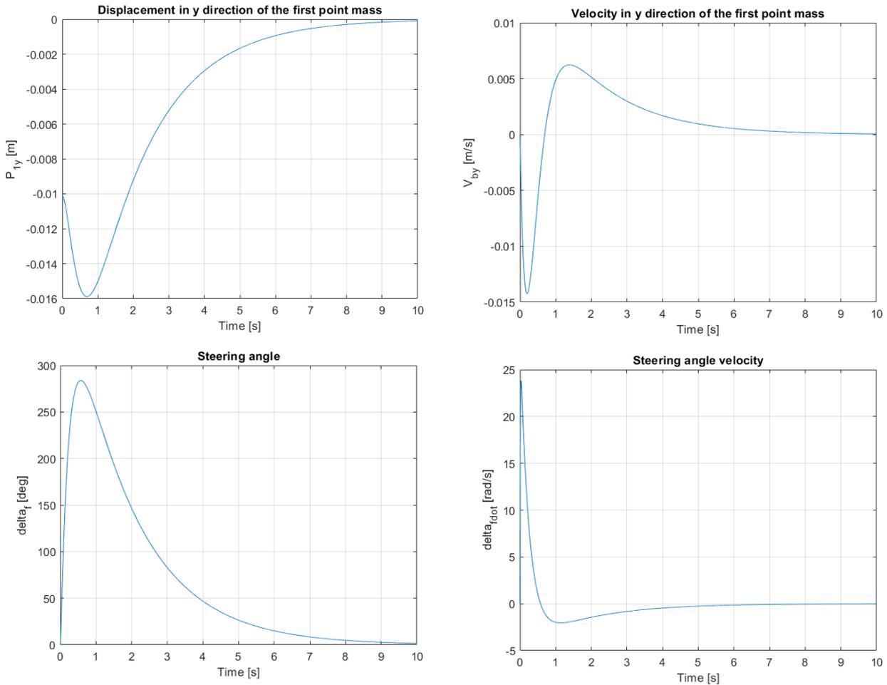
**Figure 3.16:** Results of the simulation with  $d = 0.0463 [m]$  and  $t = 0.110 [m]$  with the LQR control
