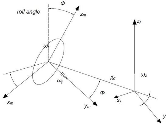
**Figure 1.17:** gyroscopic moment generated by the wheel rotational speed  $\omega_f$  and the yaw motion  $\psi$
