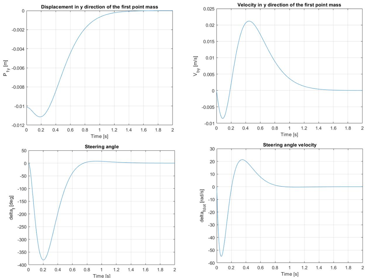
**Figure 3.10:** Results of the simulation with offset  $d = 0.0774 [m]$  and  $t = 0.075 [m]$ .
