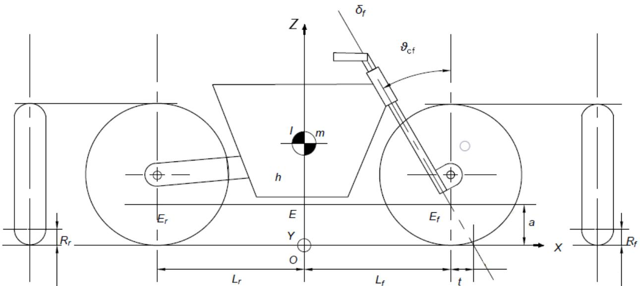
**Figure 3.1:** Dynamics model of a motorcycle
