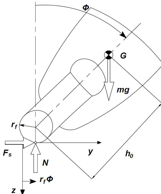
**Figure 1.16:** capsize model of the motorcycle with lateral rolling of the tire
