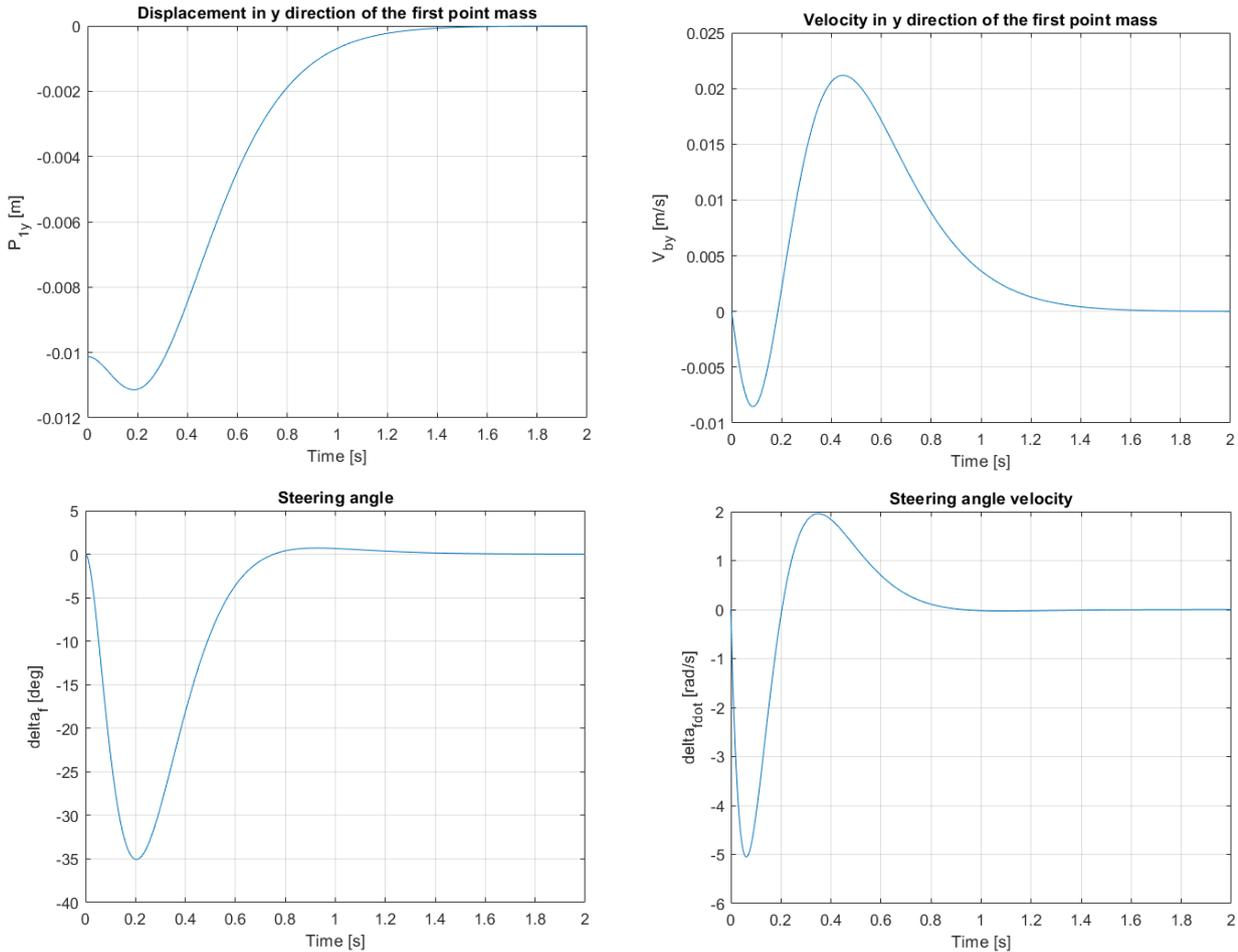
**Figure 3.15:** Results of the simulation with offset  $d = 0.1973 [m]$  and  $t = -0.060 [m]$  and the modified wheelbase with  $L_f = 0.665 [m]$
