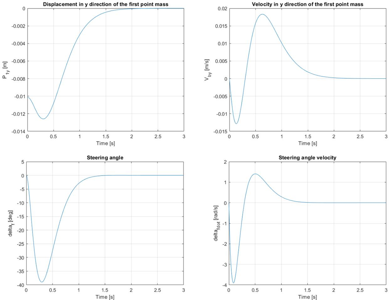
**Figure 3.14:** Results of the simulation with offset  $d = 0.1973 [m]$  and  $t = -0.060 [m]$  and the poles set at  $[-6, -6, -6, -6]$
