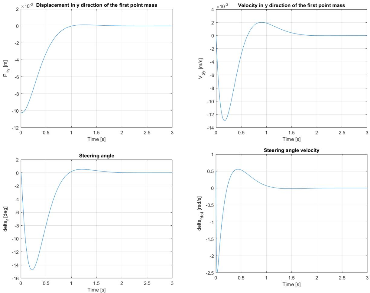
**Figure 3.28:** Results of the simulation with the steering gyroscopic effects generated at  $V_{ox} = 1 \left[ \frac{Km}{h} \right]$
