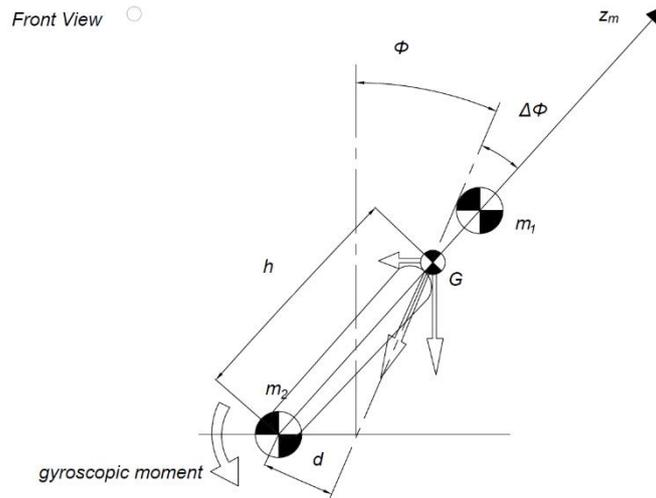
**Figure 1.19:** Increase in the roll angle  $\phi$  caused by yaw gyroscopic effect
