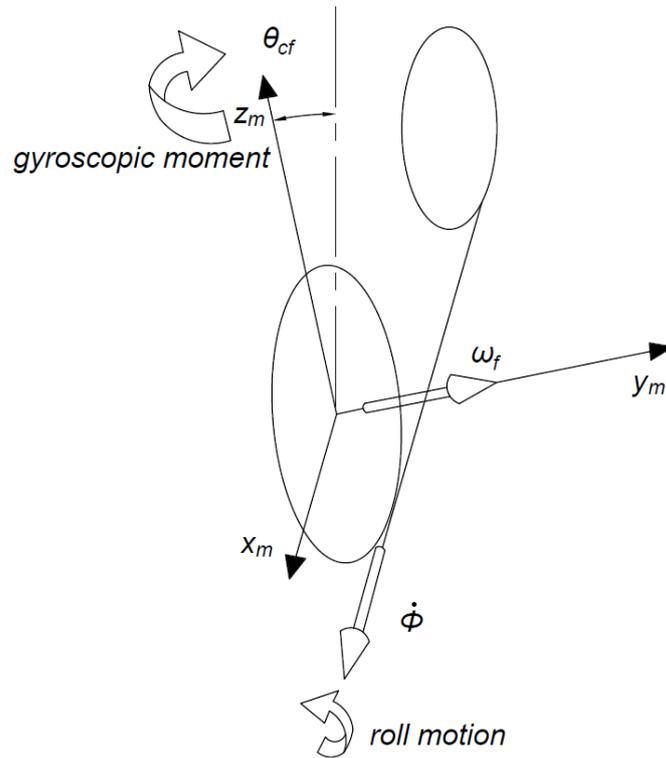
**Figure 1.22:** gyroscopic moment generated by the front wheel rotational speed  $\omega_f$  and the roll rate  $\dot{\phi}$
