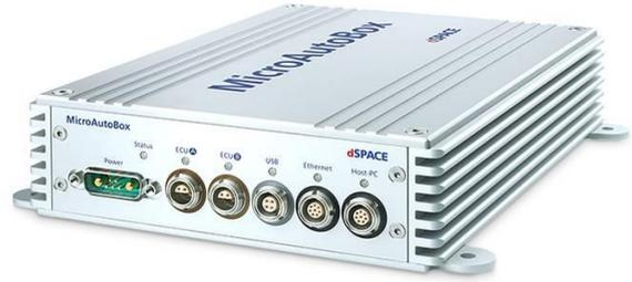
As can be seen from the scheme above, the ECU is the most important electronic component in the vehicle: its main function is to acquire sensor and auxiliary board signals, utilize them in its control logic to determine various outputs. The main output of the control system is the torque request, determined
