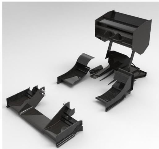
mounted on a slanted surface. However, the increased downforce was found to be worth the 5mm estimated increase in CoG height after simulation and analysis. The overall  $C_x$  and  $C_d$ , obtained through CFD simulation, resulted to be 1.03 and 3.7 respectively, giving an efficiency of 3.6.
