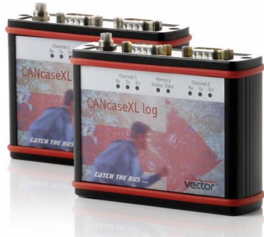
The datalogger utilized in the vehicle was a Vector CANcaseXL connected to the vehicle CAN line. The relevant signals, defined in a .dbc file, are logged on an SD card or alternatively monitored live by connecting a PC through USB for static tests. The software used to read the data logs is Vector CANalyzer, with the possibility to export data in various formats for post processing.
