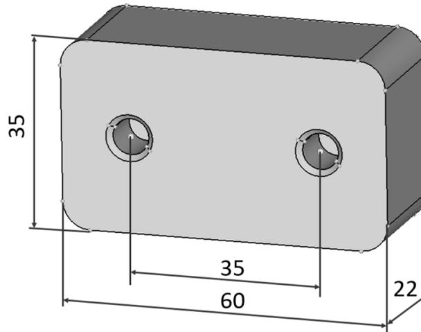
Figure 13: Suspension insert dimensions
