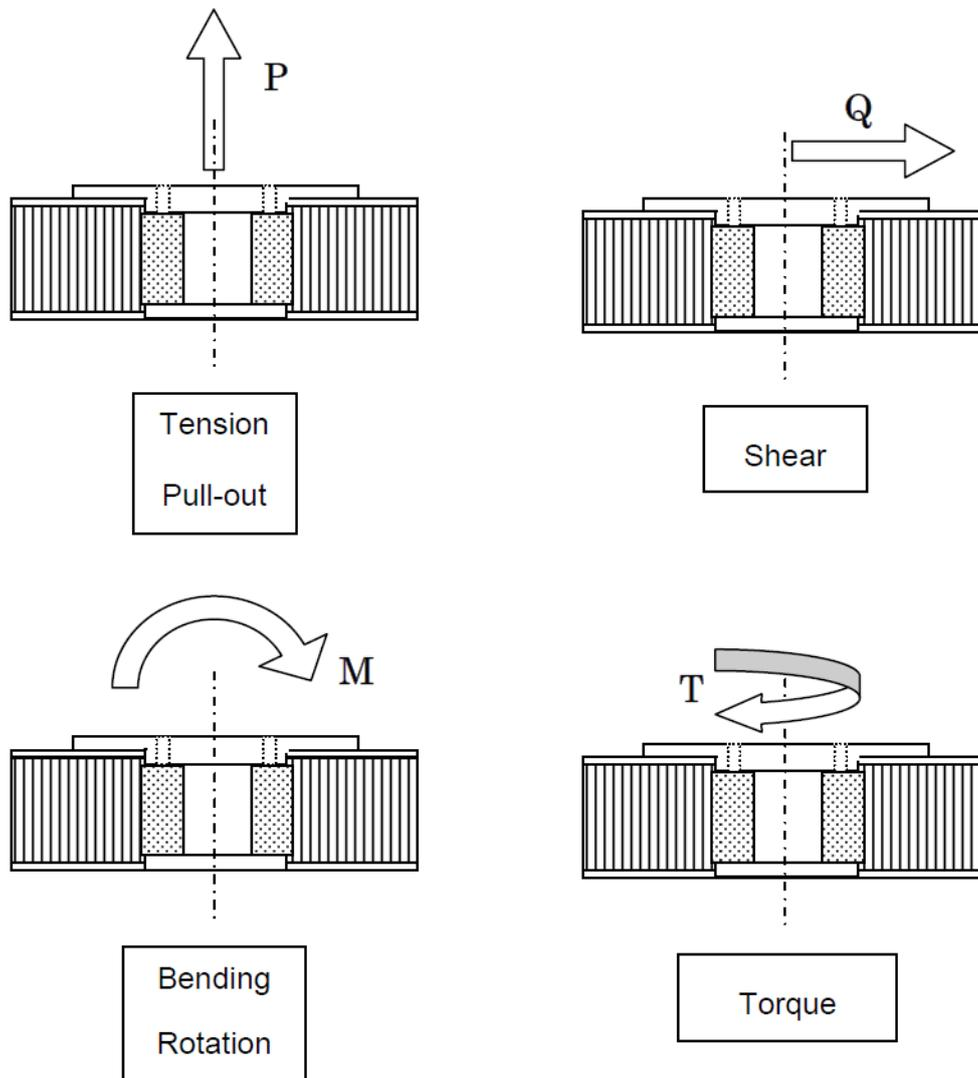
Figure 6: Insert Loadings mode
