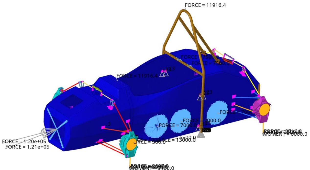
Figure 11: SCXV full vehicle model for general lay-up design
