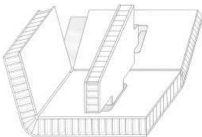
In racing application where weight and stiffness are the main drivers, the extended use of composite materials has been used starting from 1960's by Cooper Formula 1 cars. The structure consisted of a hand worked aluminum outer skin, an aluminum honeycomb core and a GRP inner skin.
