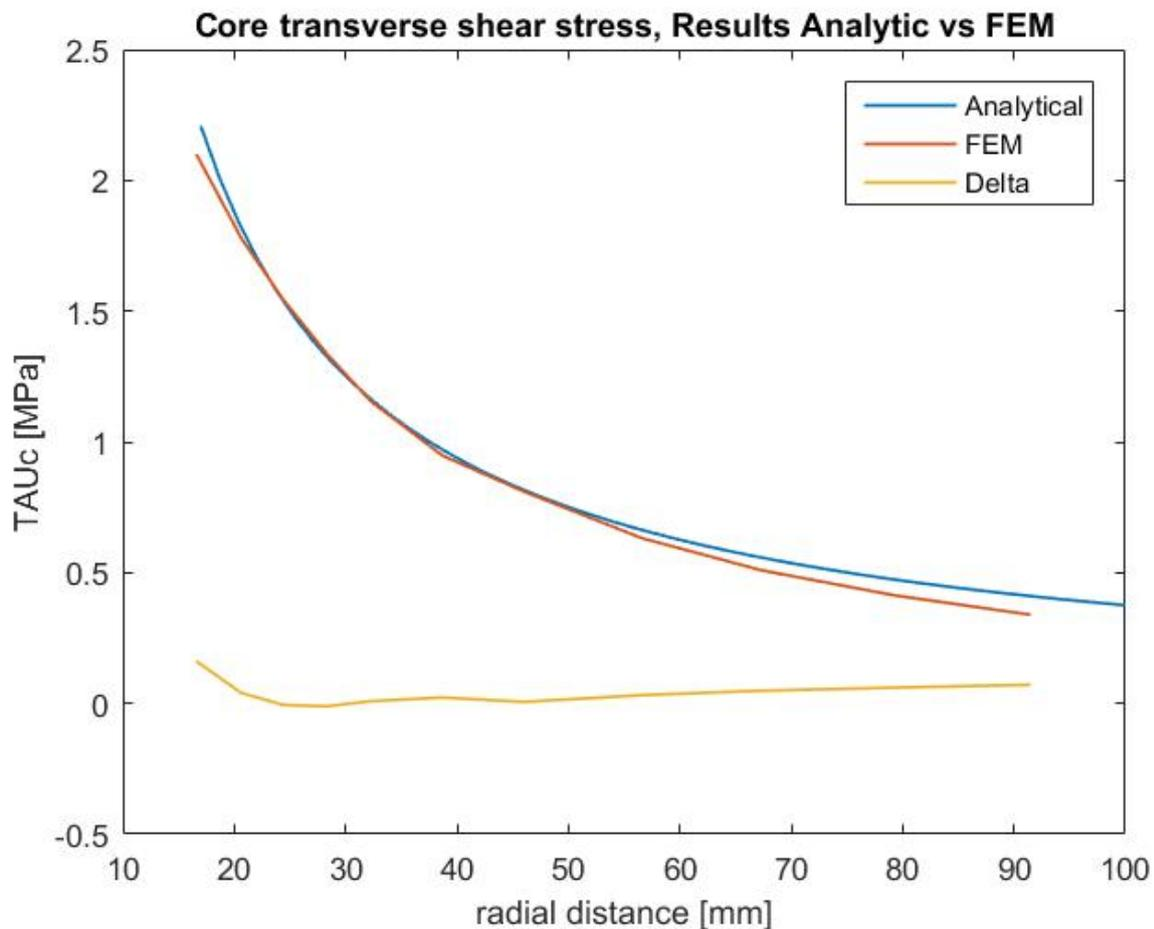
**Fourth** hypothesis, the failure point. The FEM model used for the simulation is a Linear Elastic and its not possible to simulate the failure of the insert assembly, but its possible to understand the model behavior and find the weak point by comparing the Elements status with respect to the material limits. By checking the margin value of the core materiale in the TAU field the following table it's in line with the last hypothesis:
