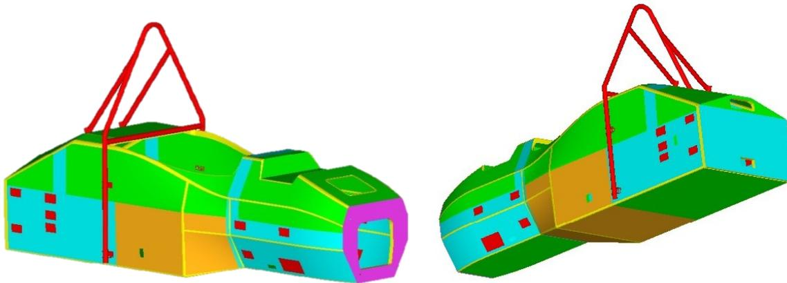
*Figure 8: SCXV FEM preliminary FEM Model*
