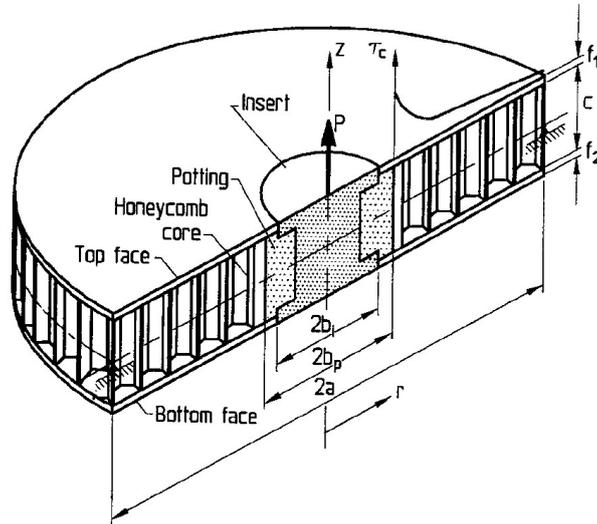
Figure 16: ECSS Anti-plane theory cylindrical coordinate system
