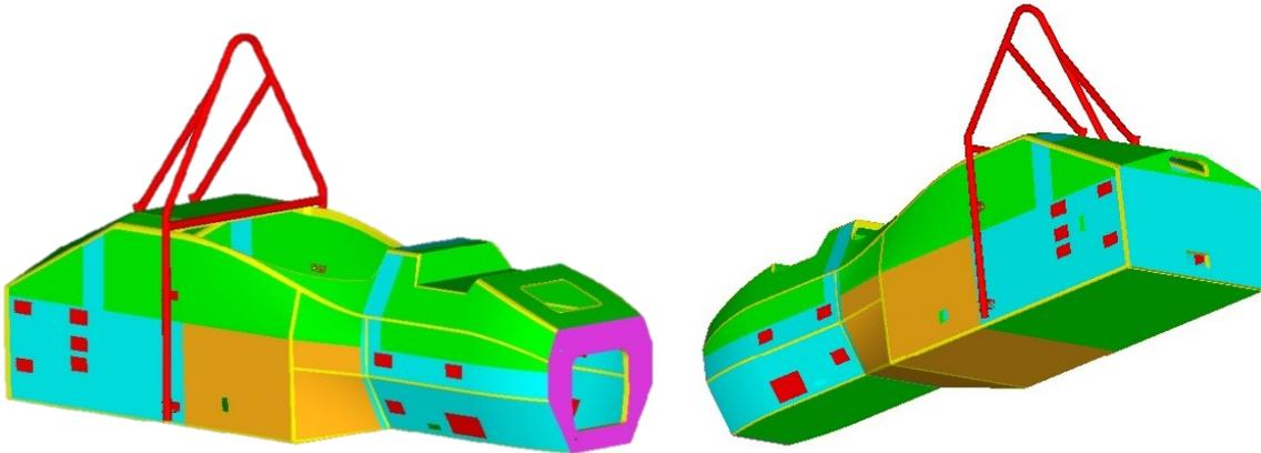
*Figure 8: SCXV FEM preliminary FEM Model*
