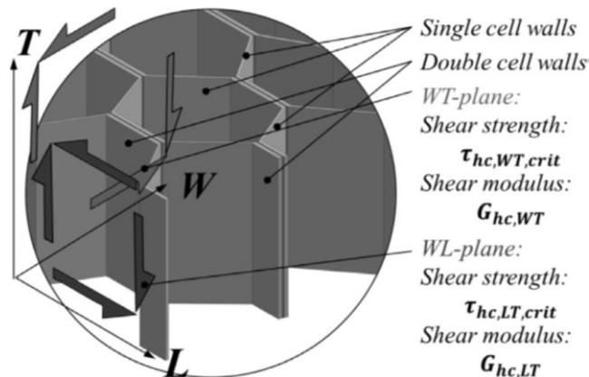
Figure 17: Effects of W and L direction in the honeycomb morphology
