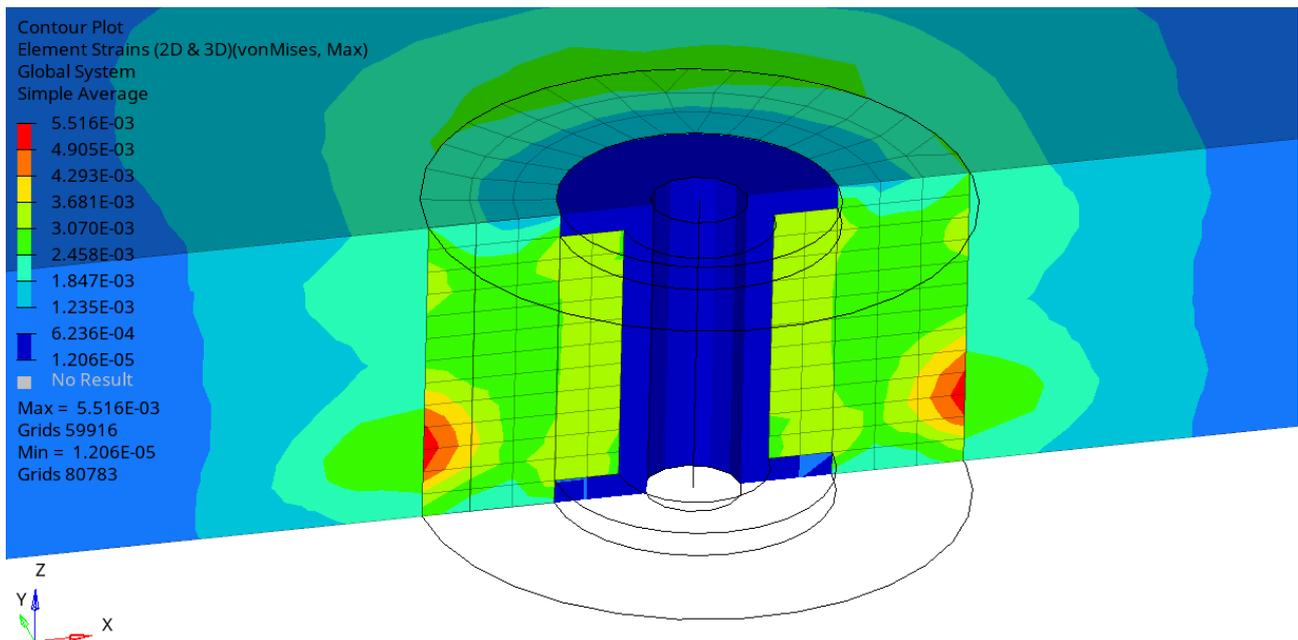
**Second** hypothesis, the plot shows the Shear stress of the honeycomb material along its thickness and distance from the insert axis. The stress is constant over the core thickness.
