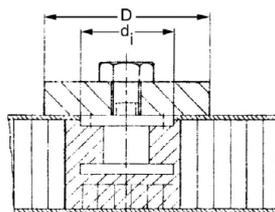
Figure 15: Example of proper overlap between Insert radius and backplate
