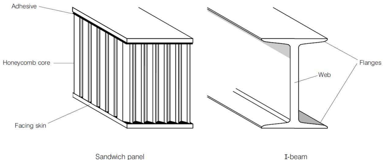
*Figure 1: Construction of a sandwich panel compared to an I beam*
