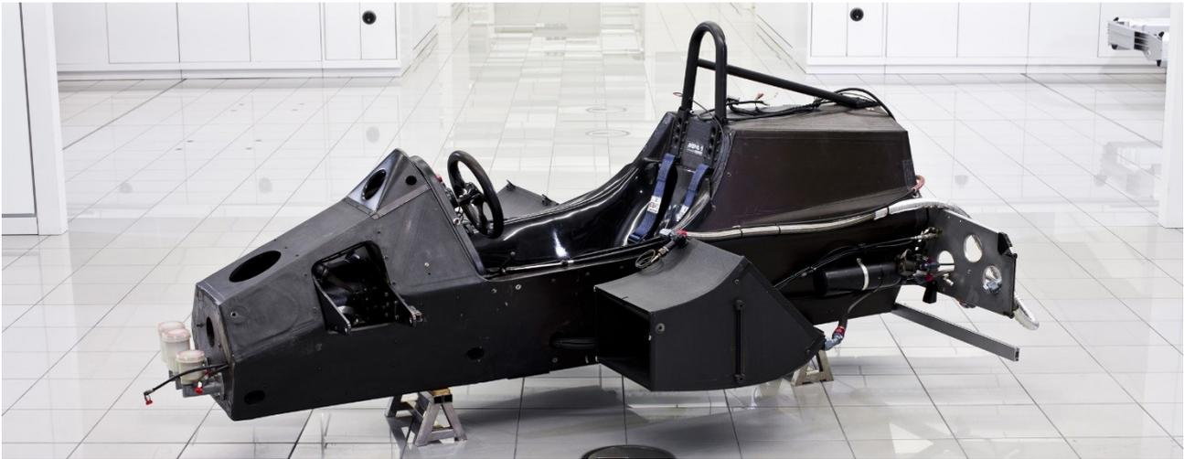
*Figure 4: McLaren MP4/1 Carbon Monocoque*
