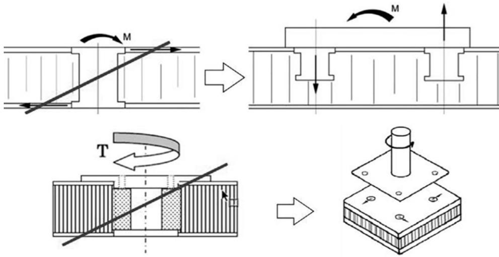
*Figure 7: Constructive measures to avoid bending and torque loads on insert load introductions*
