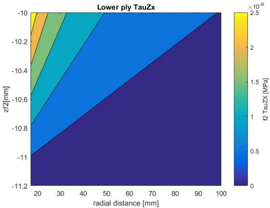
As seen in the radial transverse shear stress resultant  $Q_r(r)$ , also the core, f1 and f2 plies have a hyperbolic shear stress trend. The value of the shear stress over the thickness  $c$  is constant,
