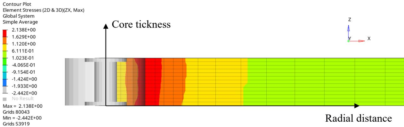
**Third** hypothesis, Hyperbolic trend of the honeycomb shear stress in the radial direction (for the FEM model this corresponds to the 31 direction of the core material). In this case it's possible to make a 1:1 comparison between Analytical and Finite Element Method results. The Fem result is a good representation within ad error of less than 5%.
