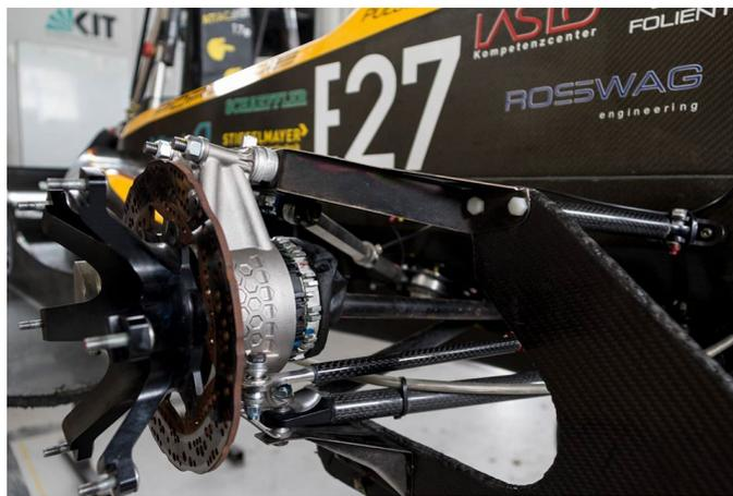
Figure 2.9. KA-RaceIng wheel assembly
