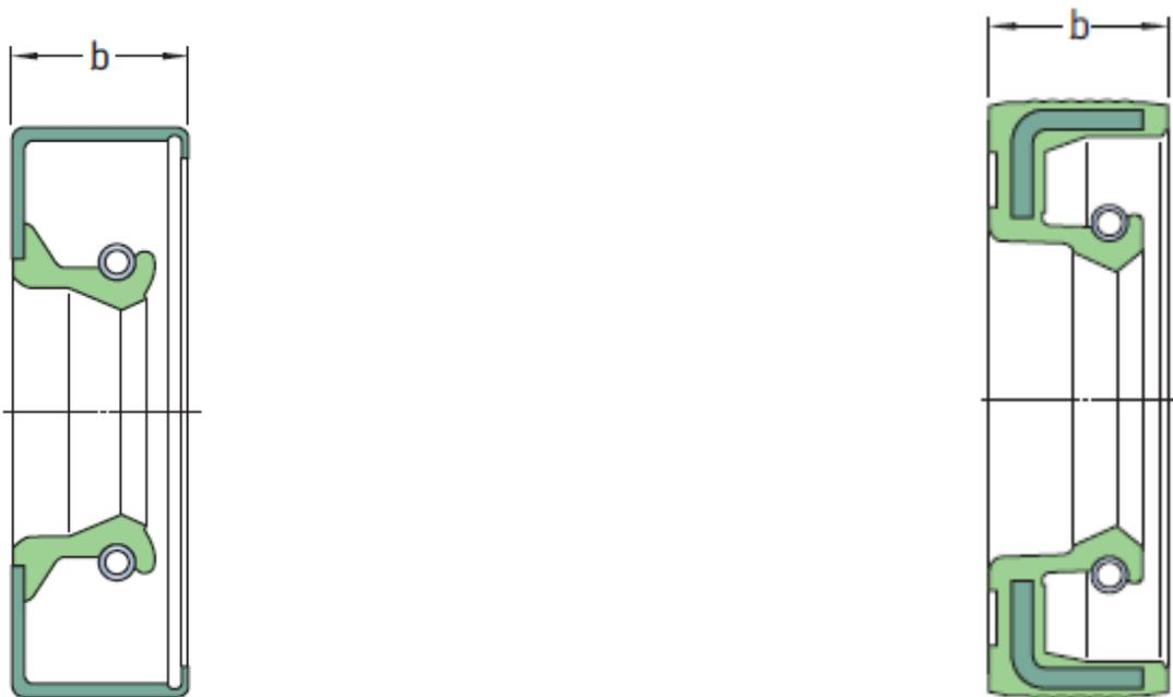
Figure 9.2. CRW1 type seal (left and HMS5 type seal (right) [13]
