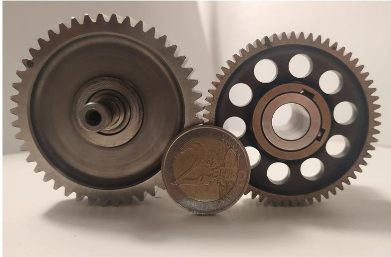
Figure 13.2. Comparison between the SCdiciassette planet gears assembly (left) and the SC18integrale one (right)
