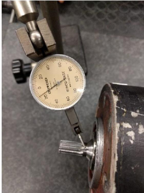
Figure 7.9. Maximum oscillation of the motor output shaft non-splined section
