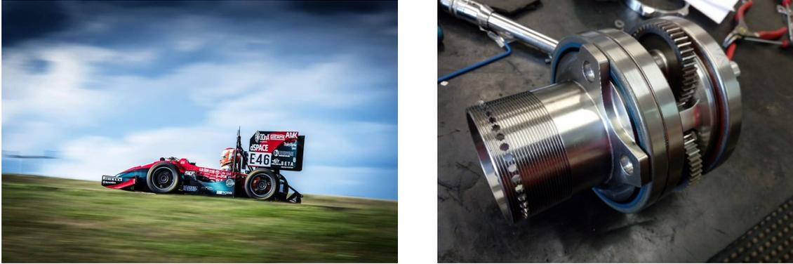
Figure 2.4. SCdiciassette with its gear train
