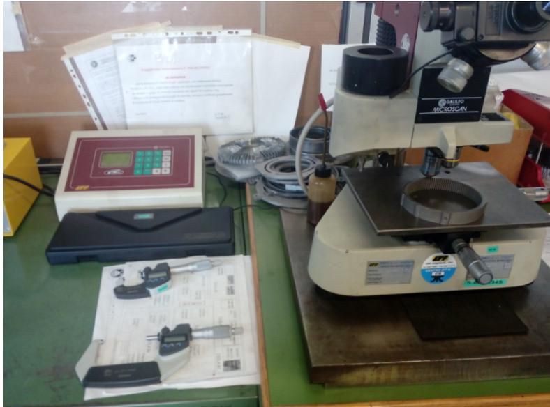
Figure 13.4. Hardness check on the ring gear
