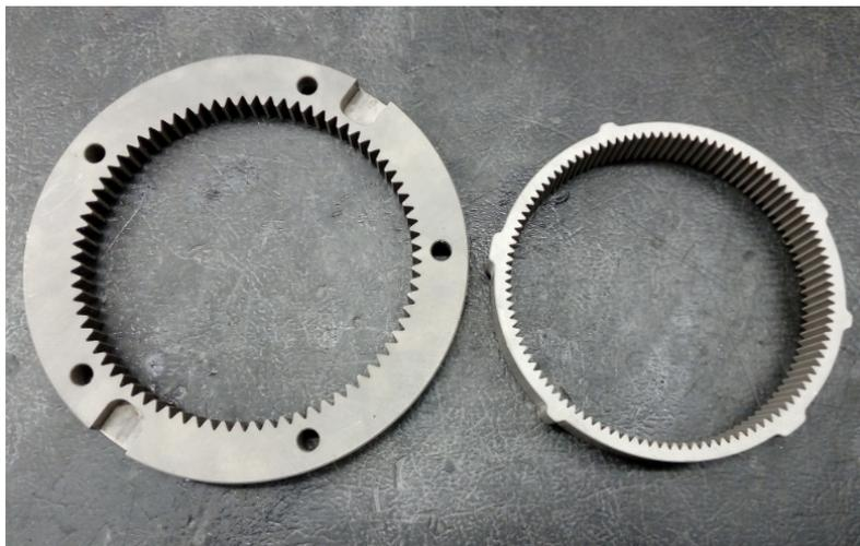
Figure 13.1. Comparison between the SCdiciassette ring gear (left) and the SC18integrale one (right)
