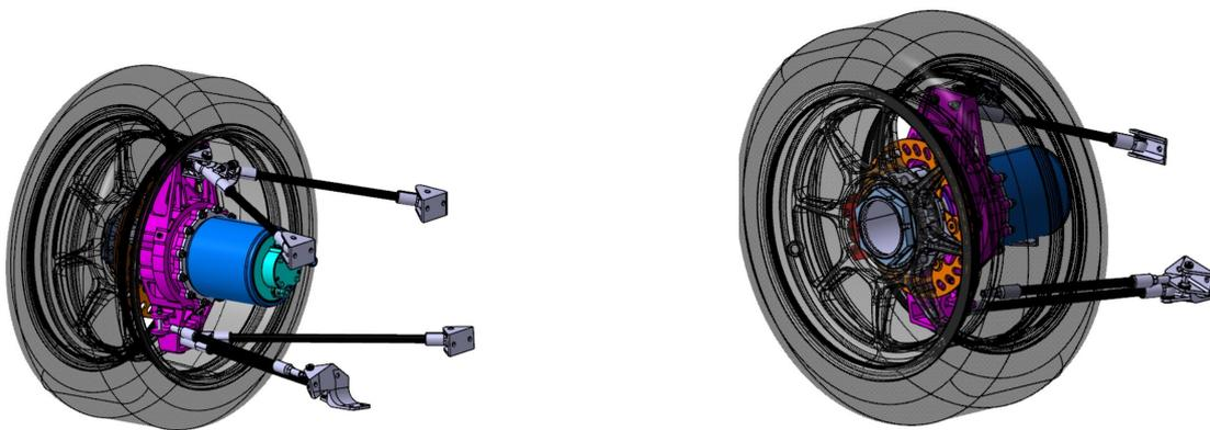
Figure 12.5. SC18integrale transmission assembled
