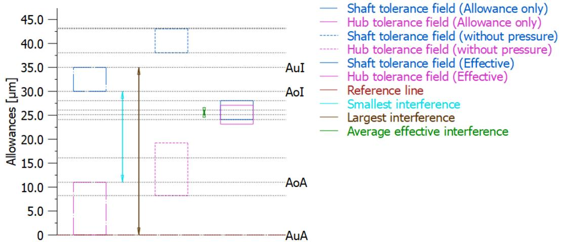
Figure 7.25. Left display: tolerance field only takes allowances into account, centre display: tolerance field takes into account temperature and centrifugal force (without pressure), right display: tolerance field takes into account temperature, centrifugal force and pressure
