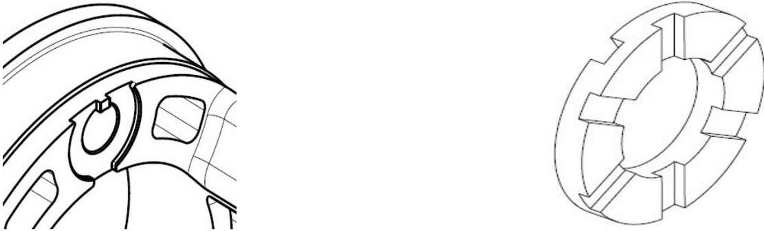
Figure 7.22. Anti-rotation pin in the carrier (left) and spacer (right)
