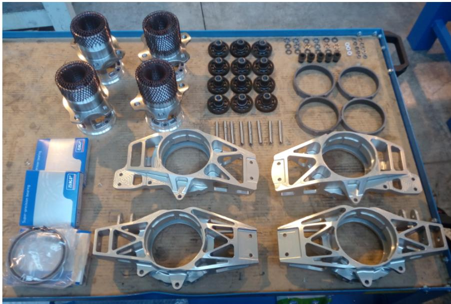
Figure 13.3. Transmission parts before assembly
