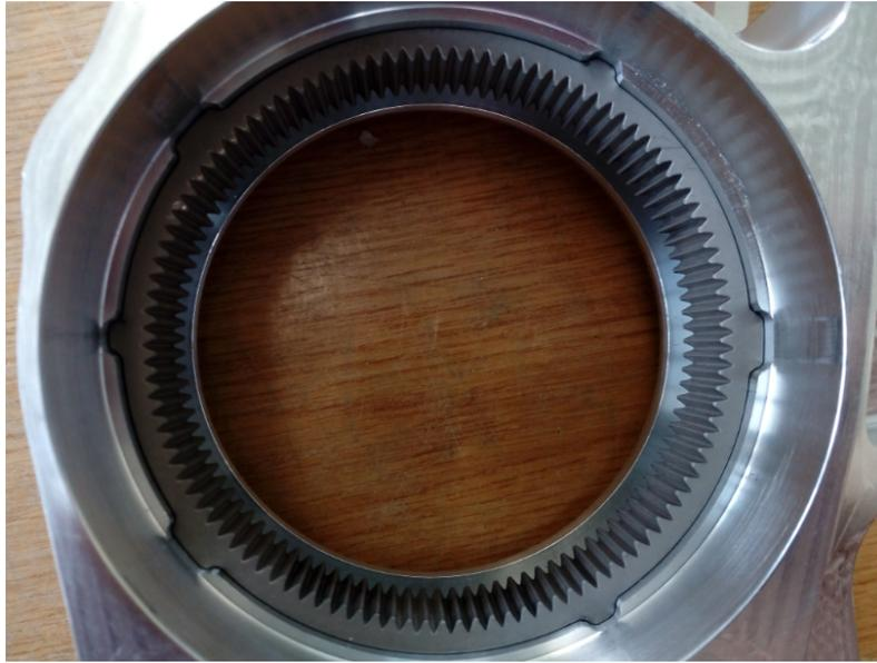
Figure 13.5. Ring gear mounted into the upright
