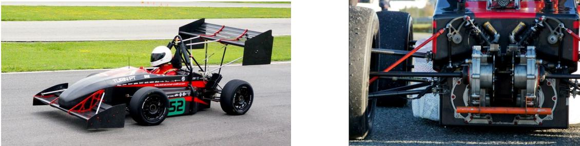
Figure 2.2. SCR with its geartrain [19]
