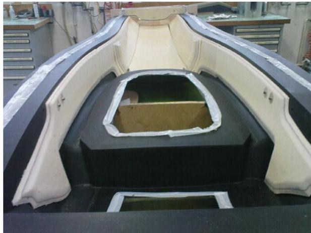
Figure 5.39: Monocoque sandwich foam core
