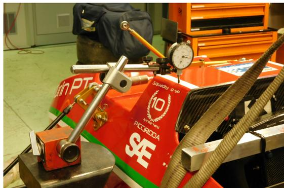
Figure 3.9: Displacements measurement on front roll hoop
