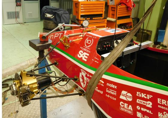
Figure 3.8: Displacements measurement on front dampers
