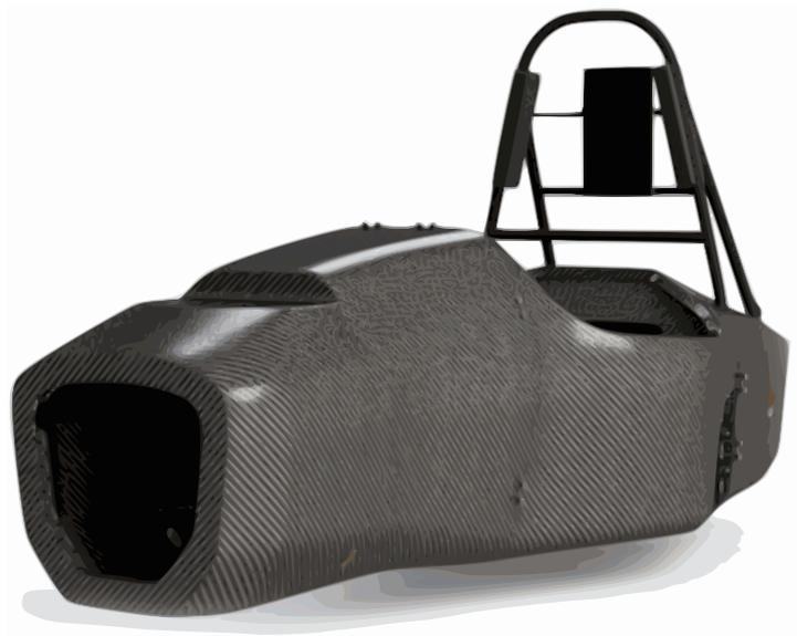
Figure 3.4: Monocoque chassis example
