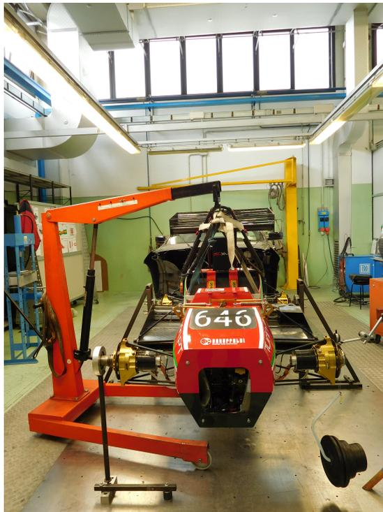
Figure 3.7: Squadra Corse asymmetric torsion test layout
