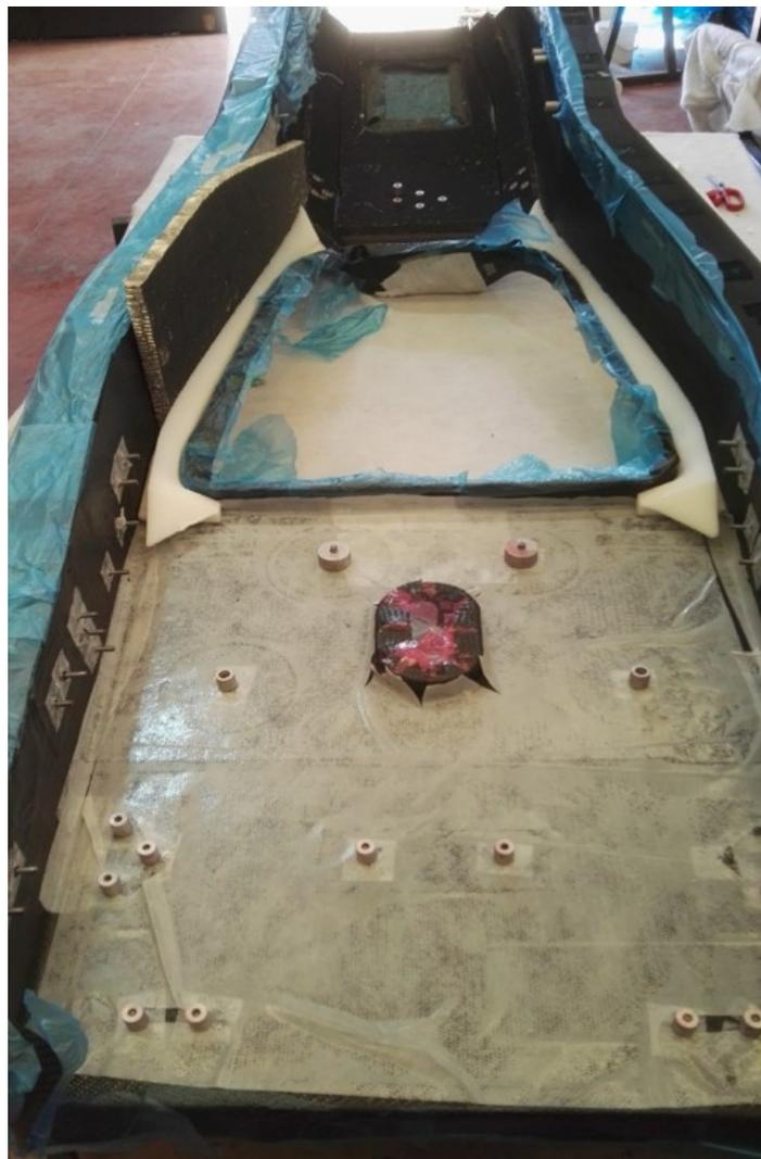
Figure 5.32: Lamination of the top half of the monocoque
