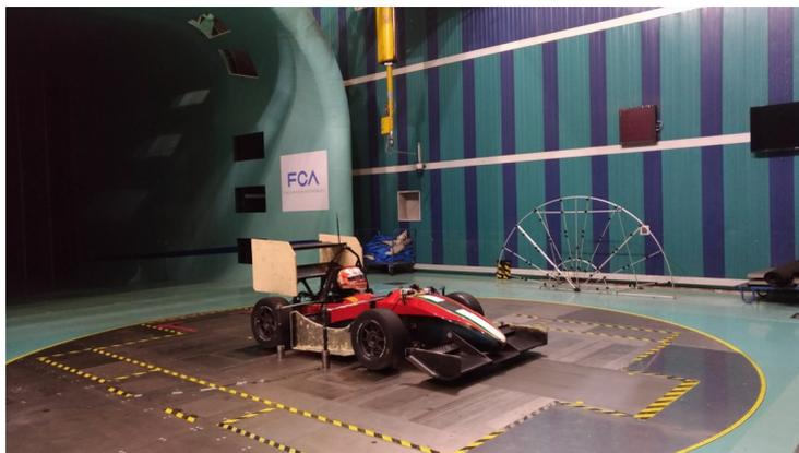
Figure 5.37: SC17 in the wind tunnel of Centro Ricerche FIAT during the validation of the aero-pack
