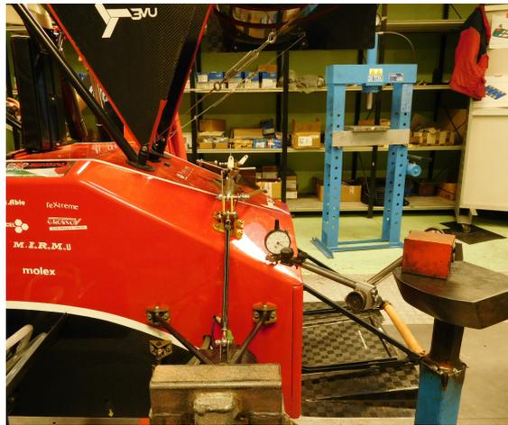
Figure 3.13: Displacements measurement at the rear-end
