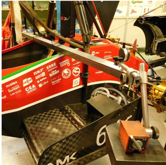
Figure 3.11: Displacements measurement at the end of the cockpit opening
