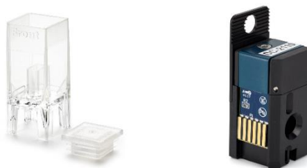
FIGURE 18 – DLS KIT: DISPOSABLE CUVETTES ON THE LEFT AND THE MOBIUS DIP CELL ON THE RIGHT. [3]
