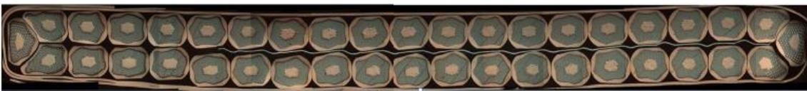
**Figure 3.6:** Cross-section of keystoneed 40-strand (0.7 mm diameter) Nb<sub>3</sub>Sn Rutherford cable with an 11 mm wide and 25 μm thick stainless-steel core [Fer2017].
