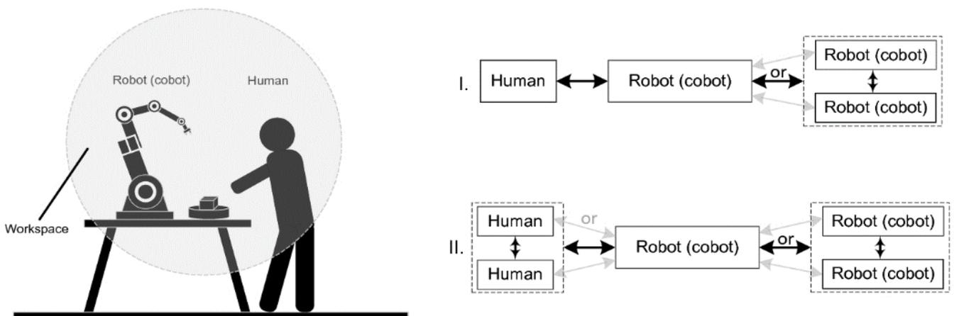
Fig. 4.26 - Human-Robot Collaboration sharing workspace (from link.springer.com)
