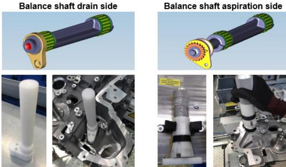
*Fig. 4.6 - Balance Shafts insertion (operator charts from Termoli T3 plant)*
