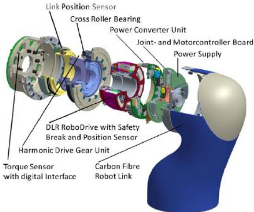
Fig. 4.5 - Mechatronic system of a Light Weight robot arm (from [8])
