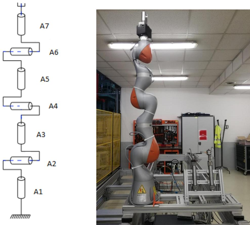
Fig. 4.3 - : Kinematic representation of the KUKA LBR IIWA 14 industrial robot and detail of the work-cell (from HRC LAB CRF)
