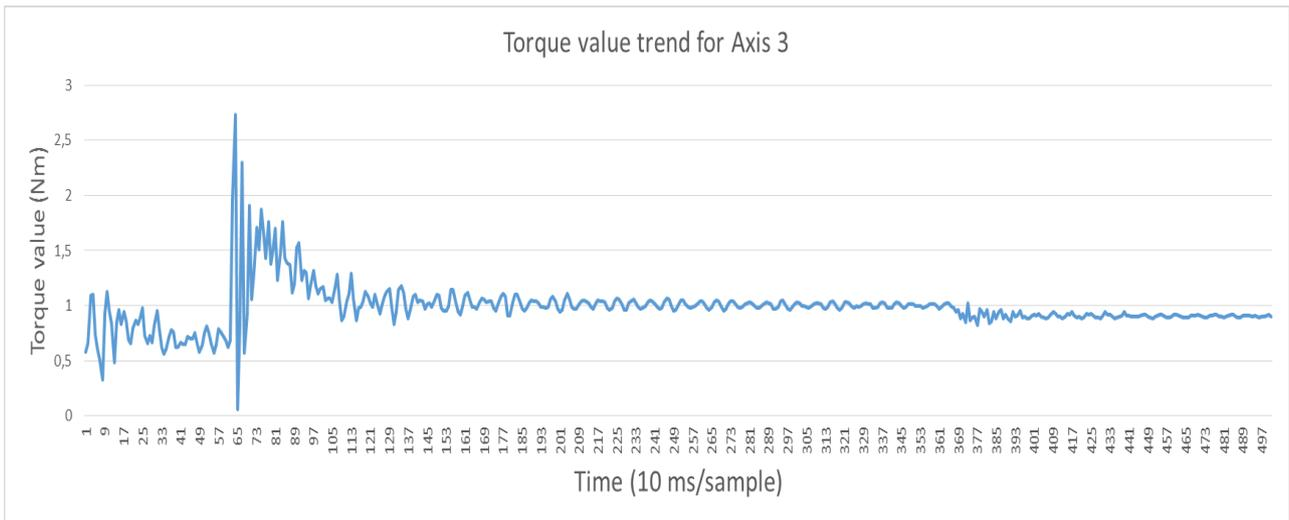
Fig. 4.14 - Torque signal from Axis 3 (drain side shaft)
