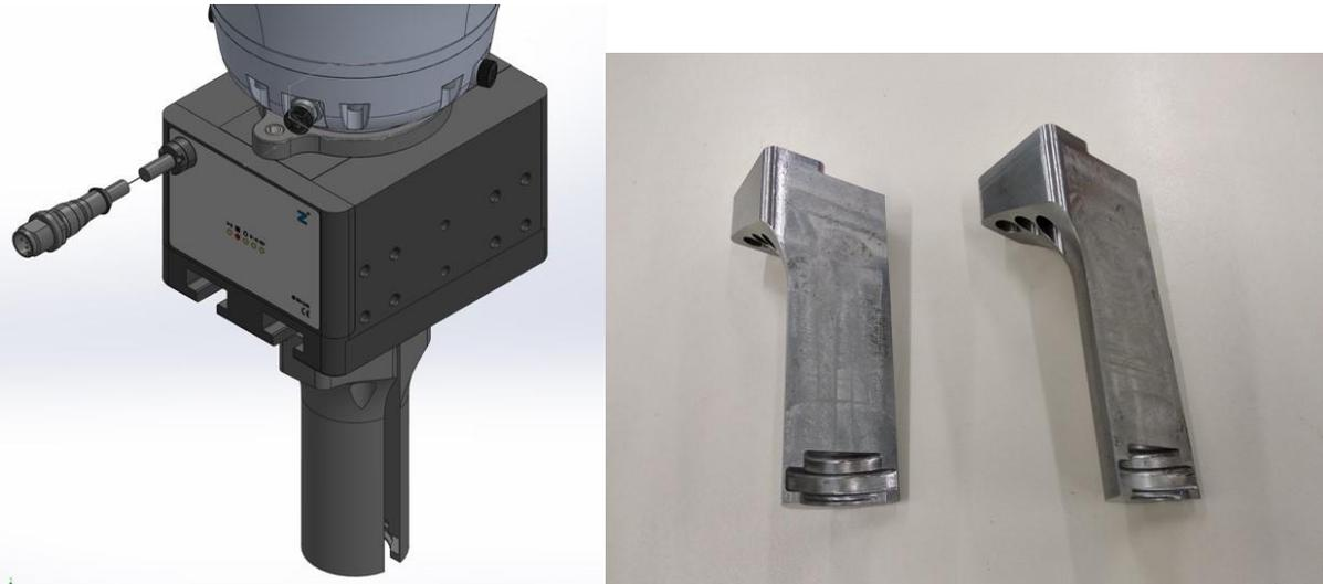
*Fig. 4.8 - Gripper CAD and Claws details (from HRC LAB CRF)*
