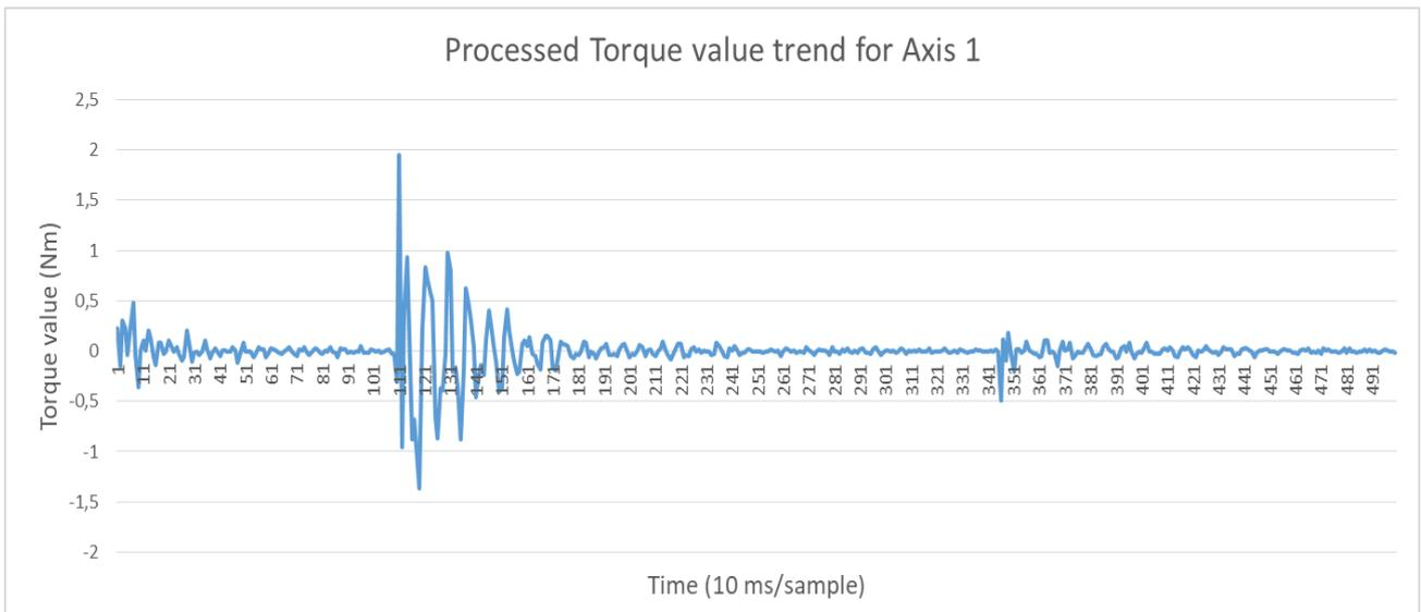
Fig. 4.23 - Processed Torque signal from Axis 1 (soft impact)
