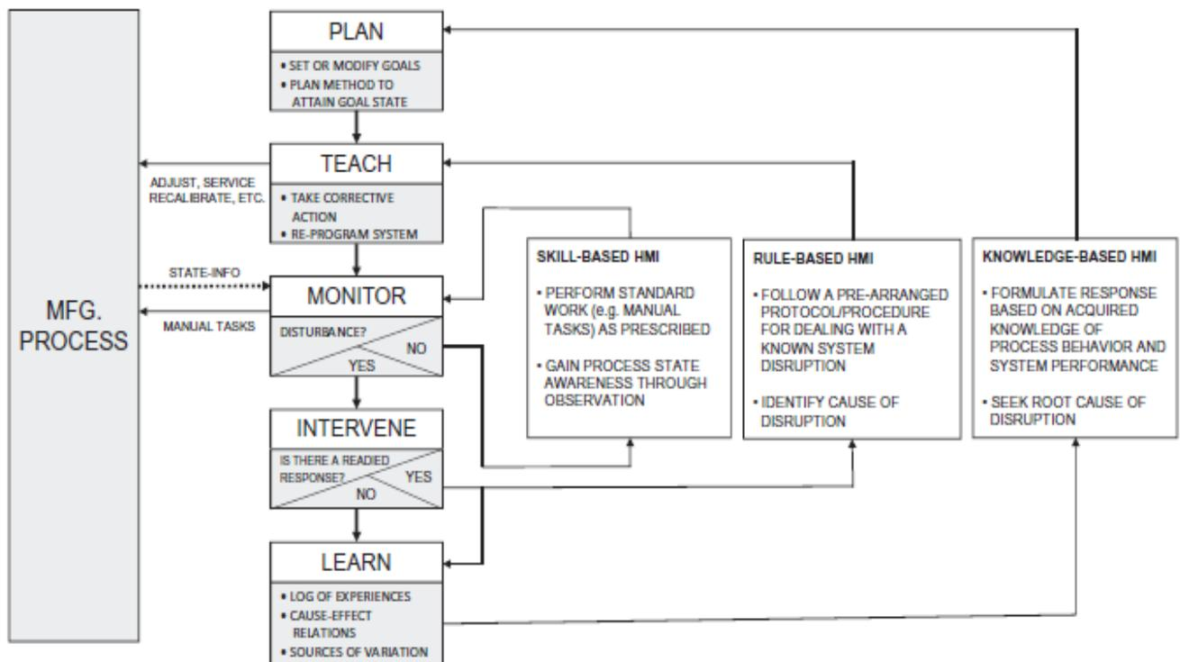
Fig. 3.5 - Nested supervisory control for three behavioural loops (from [4])
