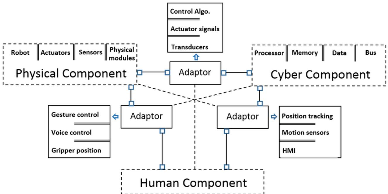
Fig. 1.6 - Diagram of a Human-Robot Collaboration framework (from ResearchGate)
