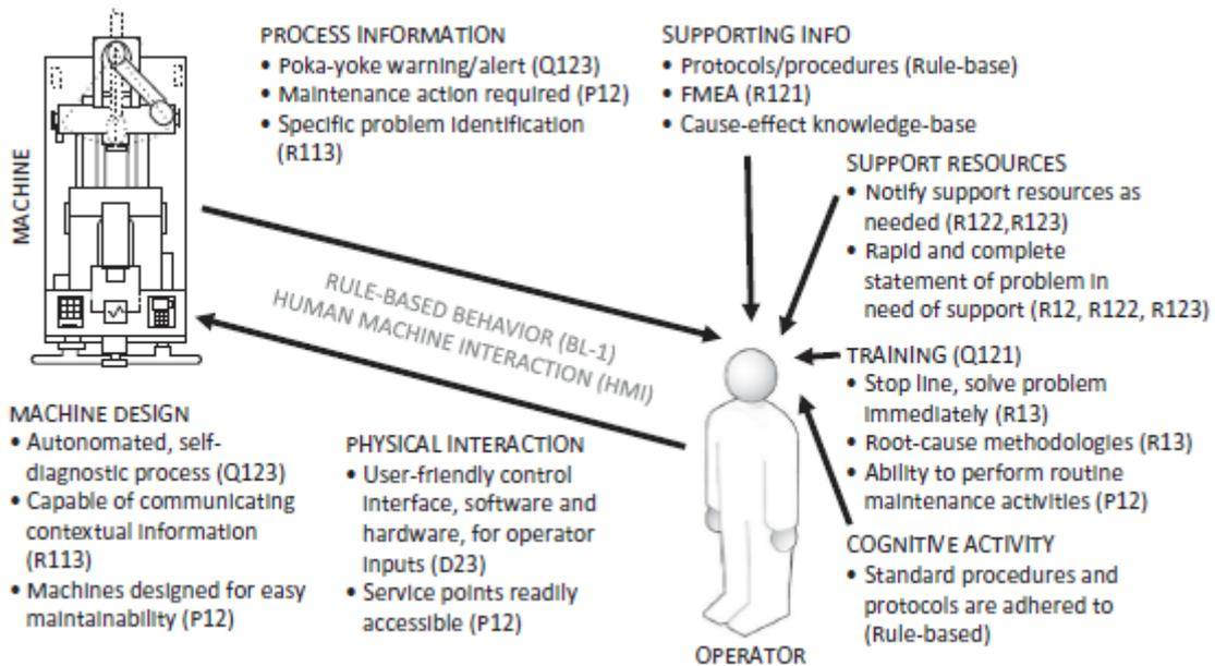
Fig. 3.3 - HMI Model for Rule-based behaviour BL-1 (from [4])
