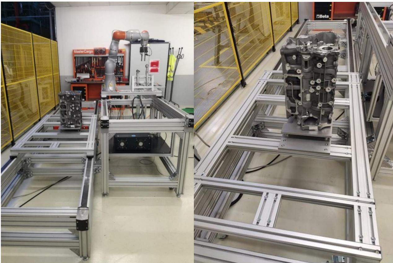
*Fig. 4.11 - Workstation and Engine block (from HRC LAB CRF)*
