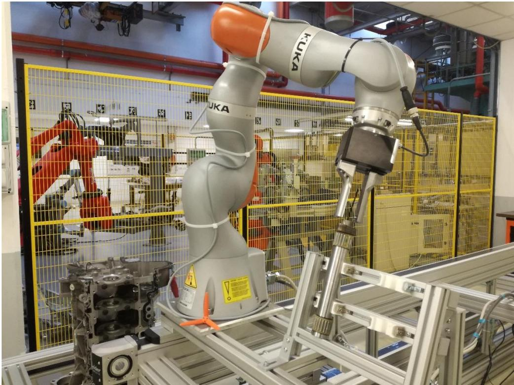
Fig. 4.17 - Gripping position for drain side shaft (from HRC LAB CRF)
