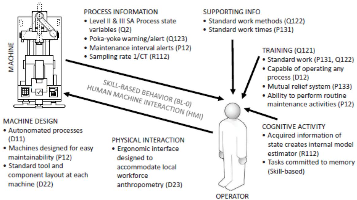
Fig. 3.2 - HMI Model for skill-based behaviour BL-0 (from [4])
