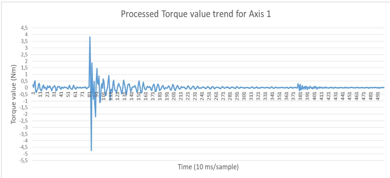
Fig. 4.25 - Processed Torque signal from Axis 1 (strong impact)
