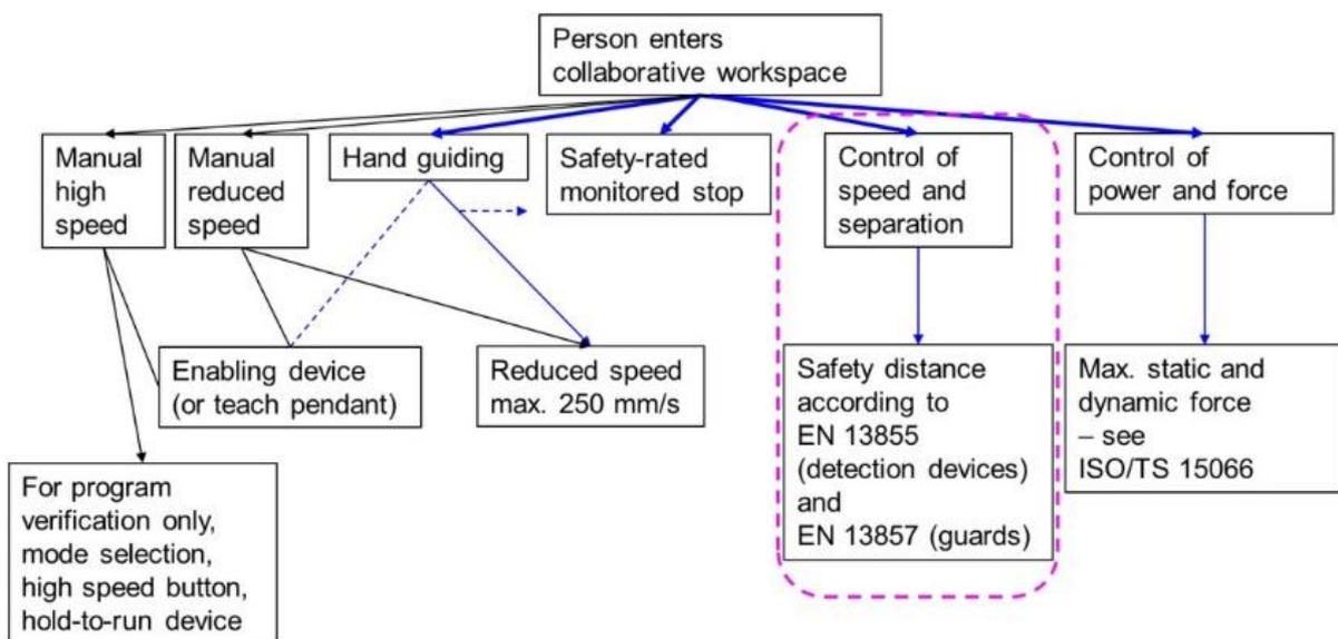
Fig.2.8 - Collaboration typologies diagram (from degruyter.com)
