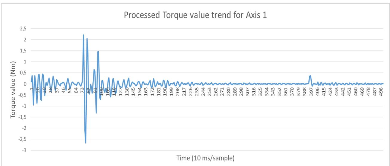
Fig. 4.24 - Processed Torque signal from Axis 1 (soft impact)
