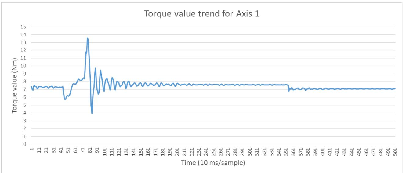
Fig. 4.15 - Torque signal from Axis 1 (aspiration side shaft, strong impact)
