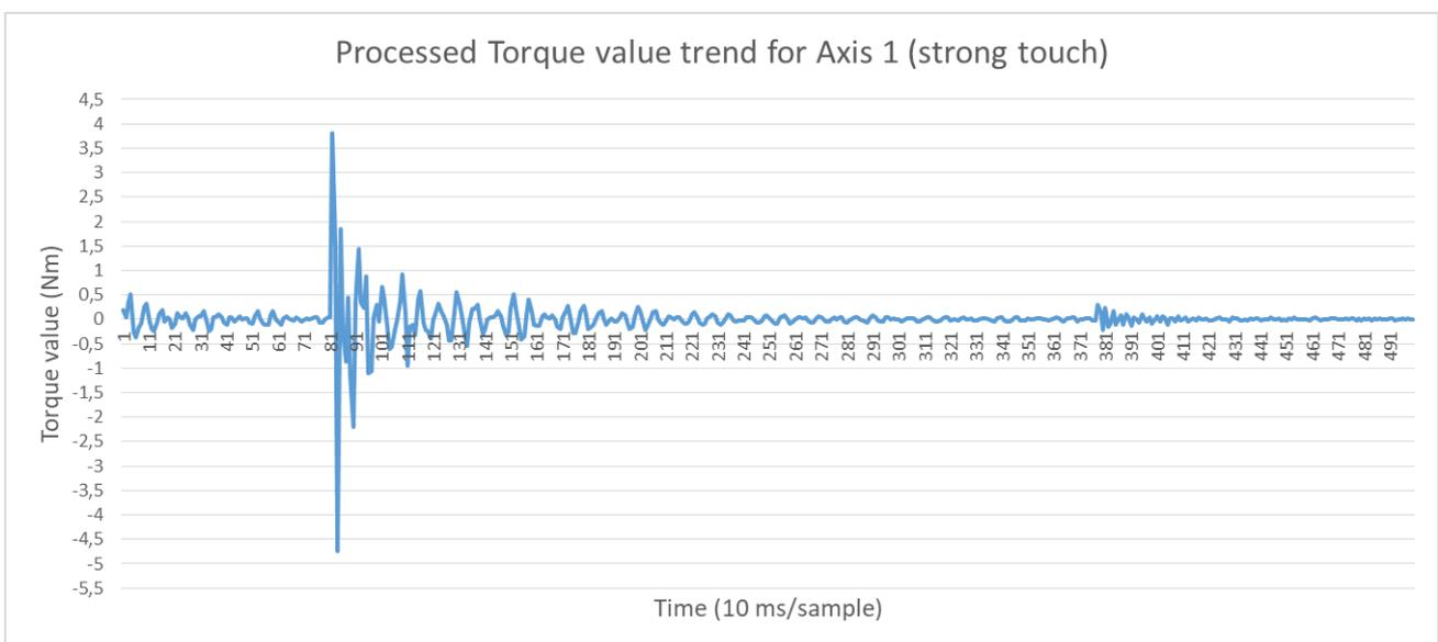
*Fig. 4.18 - Processed Torque signal from Axis 1 of Fig.4.16 (strong impact)*
