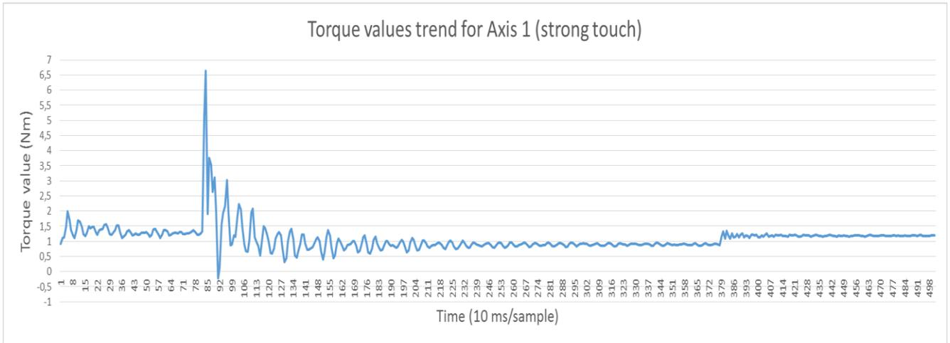
Fig. 4.16 - Torque signal from Axis 1 (drain side shaft, strong impact)
