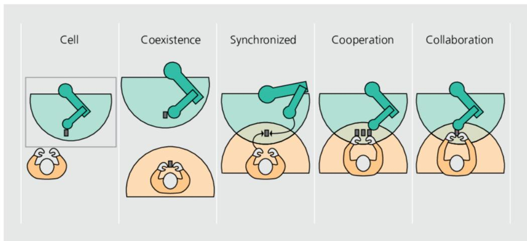
*Fig. 1.1 - Levels of Human-Machine interactions (from ResearchGate)*
