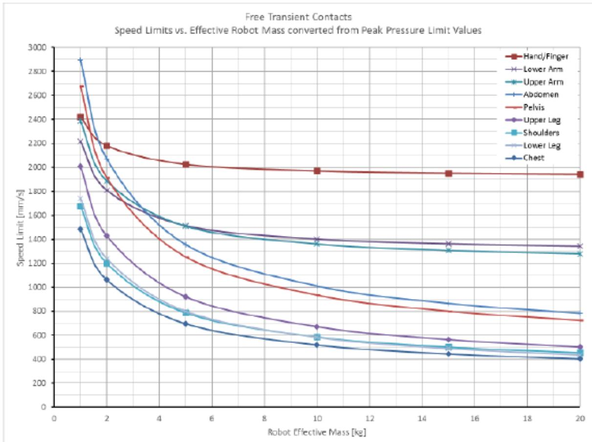
Fig. 2.17 - Mass (Pressure) VS Speed limit (from [3])
