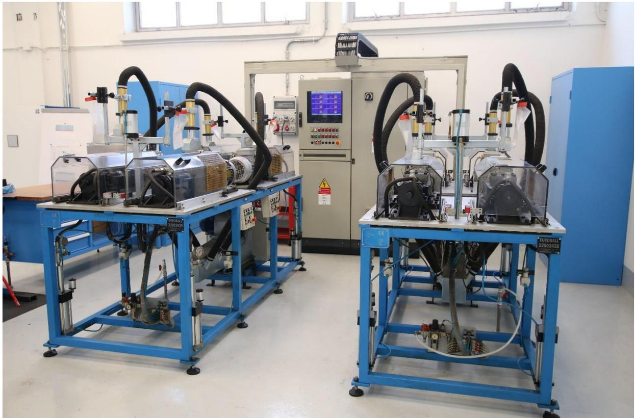
Figure 4.11 – Test rigs for ball bearing
