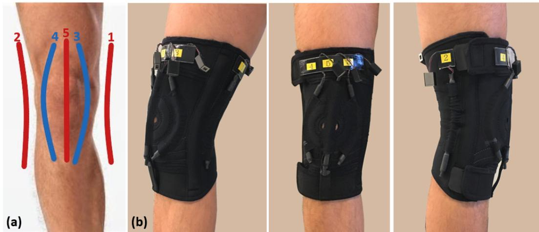
**Figure 2.11:** (a) Position and number of channel of the sensors integrated into the Mitsui Chemicals prototype; (b) Mitsui Chemicals prototype.
