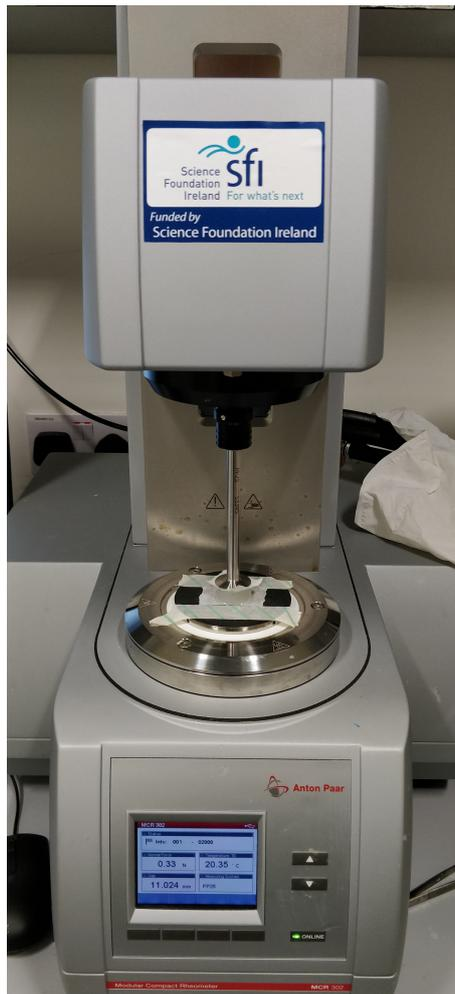
Figure 3.7 – Anton Paar rheometer.
