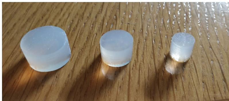
**Figure 3.6** – Cylindrical 2% agar gels of 25, 20 and 15 mm diameters ready for testing.
