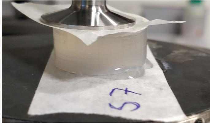
**Figure 3.10** – Example of a not centred sample.
