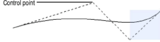
Figure 3.9: NURBS curve created by setting control points.
