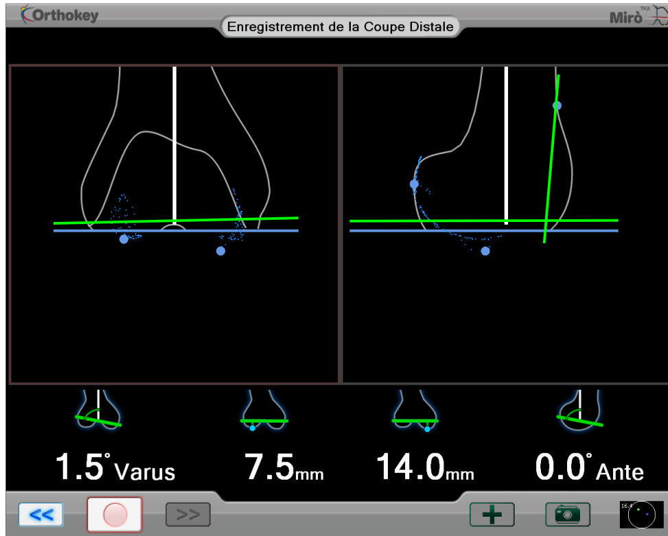
Figure 6.1: Screenshot of the software interface during a TKR surgery in which the acquisition is affected by outliers. The most distal point lies on a different plane compared to the expected bone surface. The planning of the cut is represented in a blue line, while the green line represents the real cut made by the surgeon.
