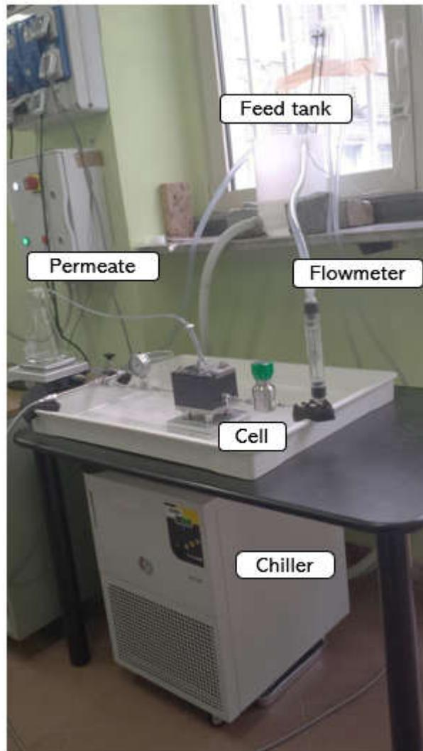
Figure 4.6: Laboratory Filtration plant
