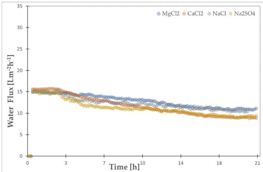
Figure 5.4: Results of the fouling tests performed at at 15 LMH, with different draw solutions and with a feed water without calcium ions. The flux decline was 30% for  $\text{NaCl}$ , 25% for  $\text{MgCl}_2$ , 42% for  $\text{CaCl}_2$  and 39%  $\text{Na}_2\text{SO}_4$ .
