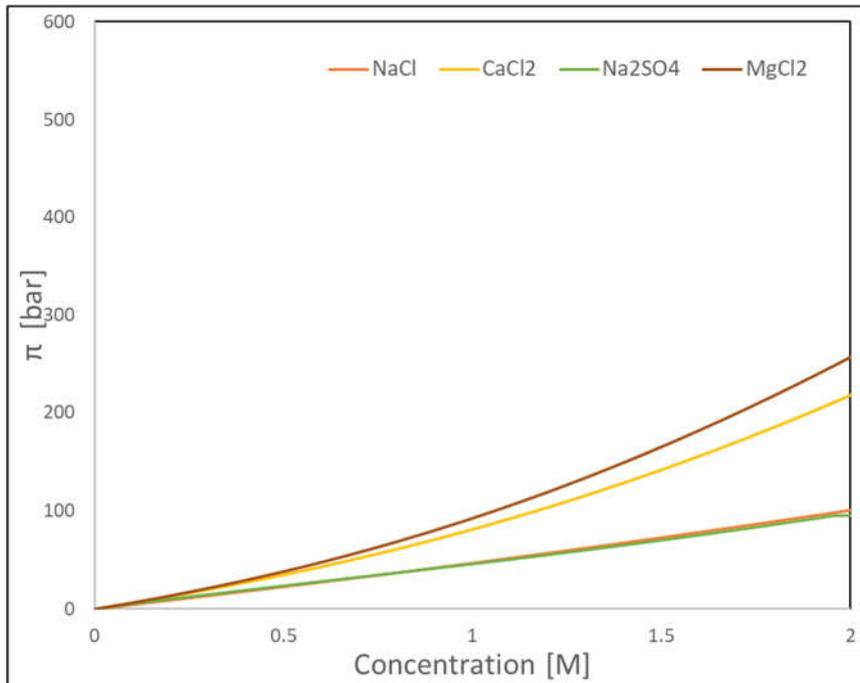
Figure 4.5: Concentration over osmotic pressure  $\pi$  for every draw solute considered. For MgCl<sub>2</sub> and CaCl<sub>2</sub>, an increase in concentration corresponds to an increase in osmotic pressure. For solutes such as Na<sub>2</sub>SO<sub>4</sub>, this is true only until a certain point, after which to an increase in concentration does not correspond an increase in osmotic pressure
