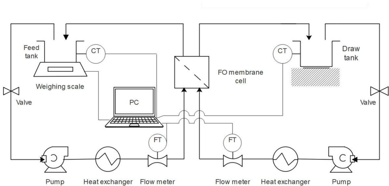
Figure 4.2: scheme of the FO lab scale set up
