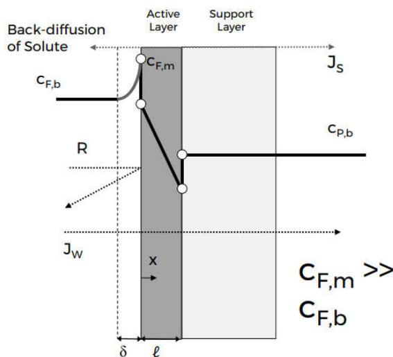
Figure 2.5: Concentration polarization stems from the solute back-up at the membrane surface, due to a difference in concentration of solute in the bulk and at the membrane. [6]
