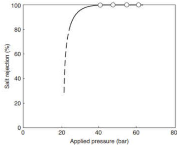
Figure 2.10: Salt rejection over applied pressure. This function is logarithmic and reaches a point in which by further increasing pressure, rejection slightly increases. [49]
