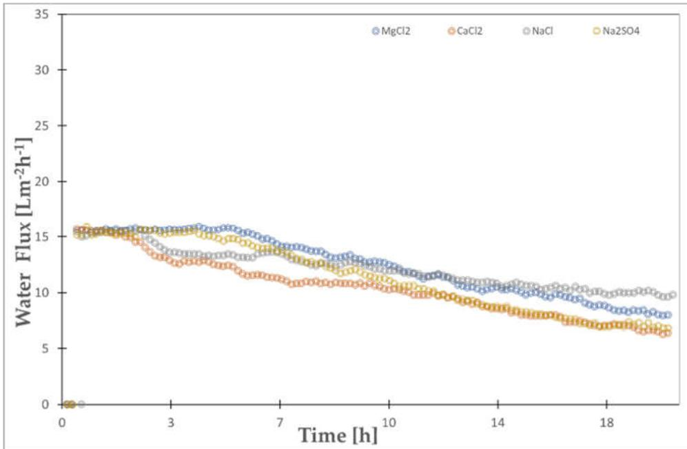
Figure 5.3: Results of the fouling tests performed at 15 LMH, with different draw solutions and with a feed water containing Calcium ions. The flux decline was respectively 50% for  $\text{MgCl}_2$ , 37% for  $\text{NaCl}$ , 58%  $\text{Na}_2\text{SO}_4$  and 56%  $\text{CaCl}_2$ .
