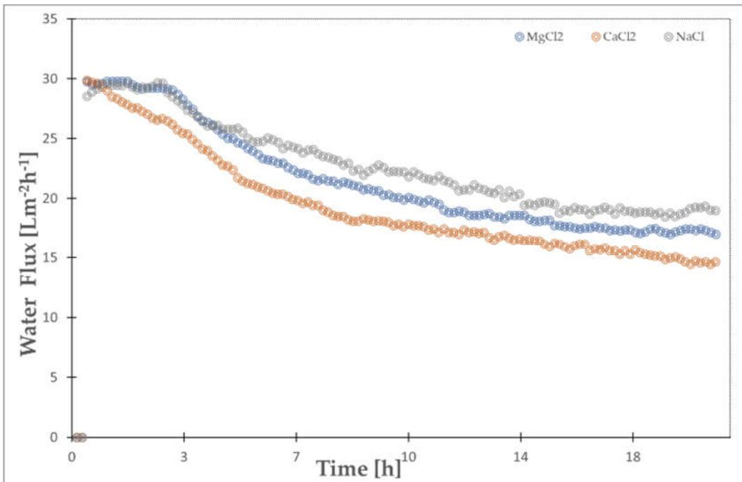
Figure 5.6 Results of the fouling tests performed at 30 LMH, with different draw solutions and with a feed water without Calcium ions. The flux decline was 34% for NaCl, 42% for MgCl<sub>2</sub>, 51% for CaCl<sub>2</sub>.
