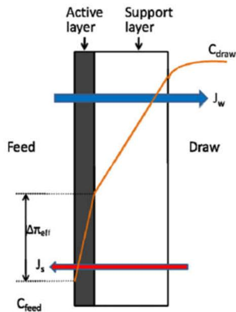
Figure 2.7: Dilutive Internal Concentration Polarization and External in Forward Osmosis. The active layer faces the feed stream. Since the Draw Solution is being diluted, its concentration inside the membrane is lower than the concentration in the draw side. [55]
