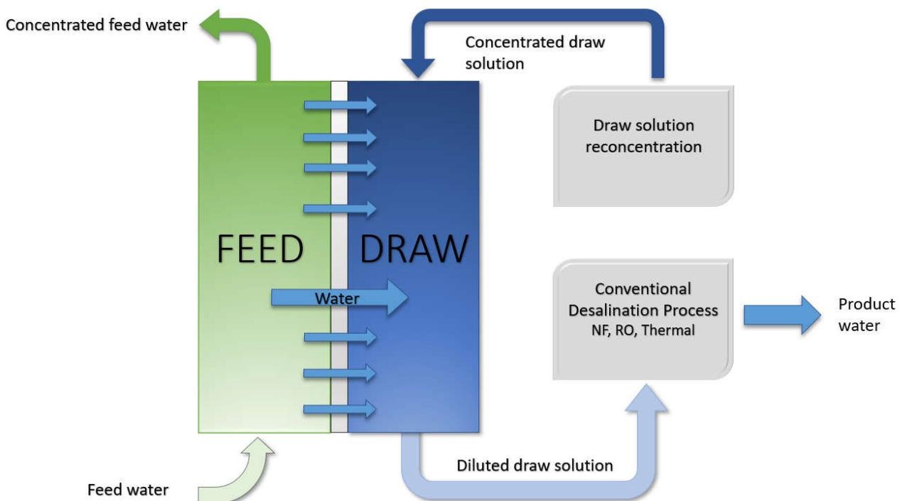
Figure 2.12: Scheme of a desalination process using FO as a pre-treatment. FO is able to dilute the feed water before it comes to the following treatment step, that could be RO, NF or a Thermal process, reducing the presence of foulants that would decrease the efficiency of the desalination process. The Concentrate can be sent back to FO, to be used as draw solution. [39]
