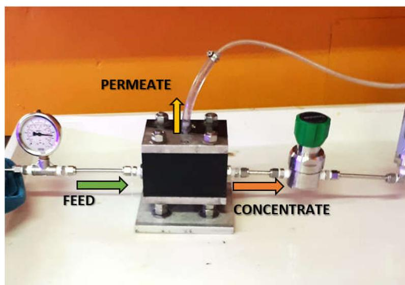
Figure 4.7: Cell used to allocate the membrane in RO mode
