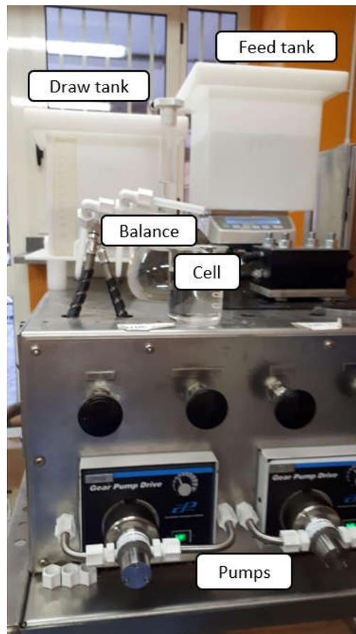
Figure 4.3: laboratory FO filtration plant
