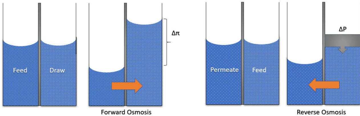
Figure 2.4: Water flux in FO and RO. At equilibrium, no movement occurs. In FO, due to a driving force, such as a difference in osmotic pressure, water is forced to pass to the more saline side of the membrane. ( $\Delta P=0$ ). For RO, water passes to the less saline side of the membrane, due to hydraulic pressure ( $\Delta P>0$ )
