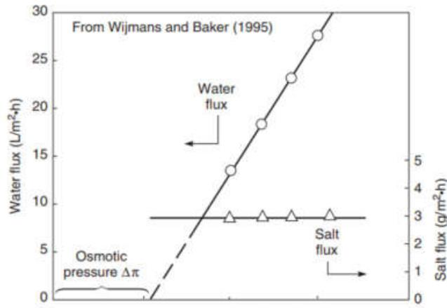
Figure 2.9: Water flux and salt flux over applied pressure. Below the osmotic pressure there is no flux. Water flux increases with applied pressure in a linear way. The salt flux has the same behaviour with increase in pressure. [49]
