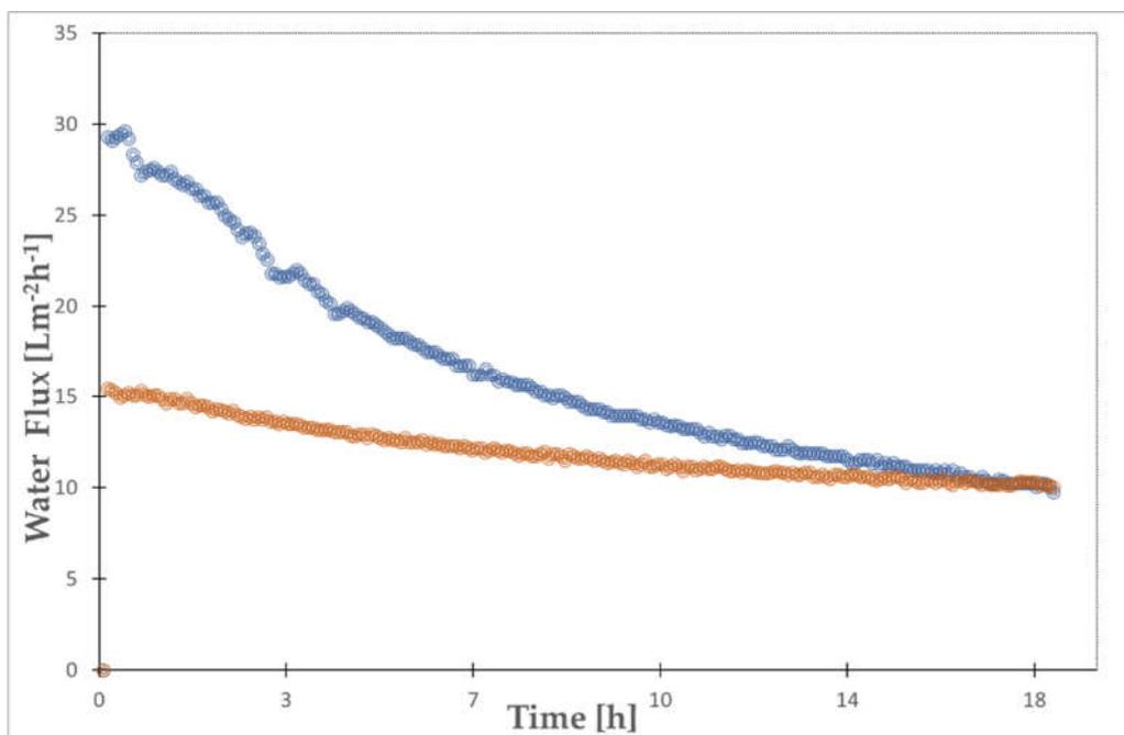
Figure 5.7: Results of flux decline in RO, at initial flux of 15 LMH and 30 LMH. The loss in flux is respectively 66% and 35%.
