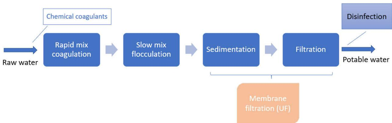
Figure 2.3: scheme of a conventional water treatment plant, compared to a membrane-based plant. The steps of sedimentation and filtration can be substituted by membrane, for example UF, and no chemicals are needed.
