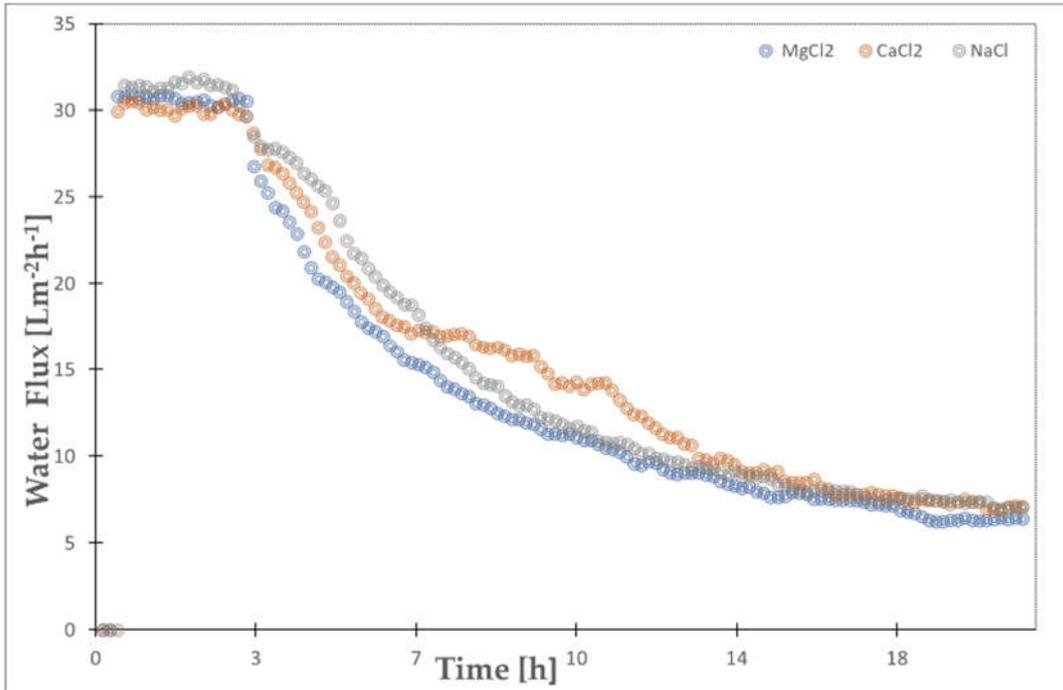
Figure 5.5: Results of the fouling tests performed at 30 LMH with different draw solutions and with a feed water containing Calcium ions. The flux decline was respectively 79% for MgCl<sub>2</sub>, 78% for NaCl and 76% CaCl<sub>2</sub>.
