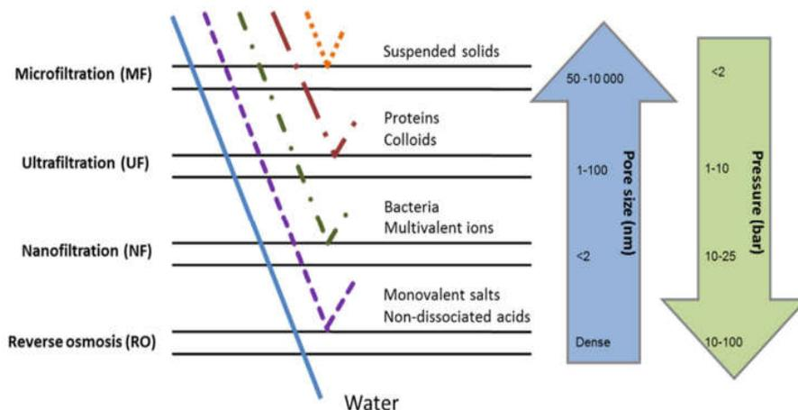
Figure 2.2: application of each membrane processes depends on pore size, but also on the pressure to be applied. Pressure is inversely related to pore size. [33]
