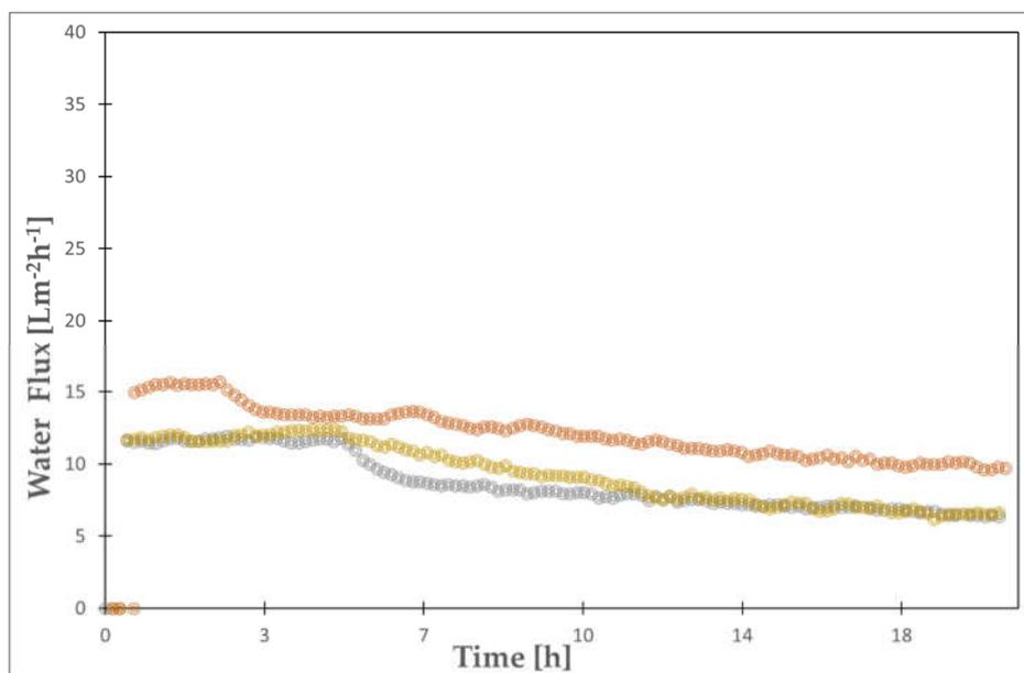
Figure 5.1 Results of the fouling tests performed with NaCl as draw solution, at different concentration, yielding different water fluxes, in the range between 0-15 LM.
