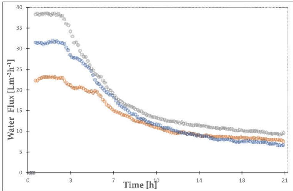
Figure 5.2: Results of the fouling tests performed with NaCl as draw solution at different concentration, yielding different water fluxes, in the range 15-40 LMH
