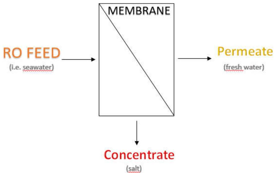
*Figure 2.8 example of seawater RO plant. The feed stream, containing a certain amount of dissolved solids, is separated in a permeate stream, with less solids, and a concentrate stream, where the concentration of solutes is higher.*
