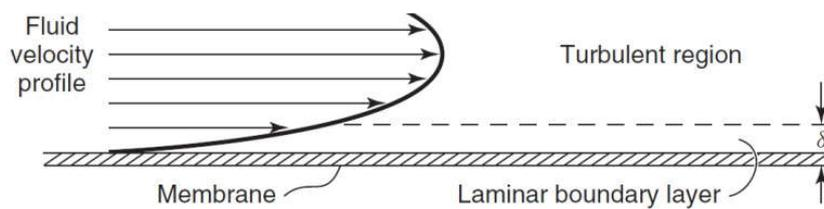
Figure 2.6: Fluid velocity profile at the membrane surface. Between the turbulent region and the membrane, there is a thin laminar layer, where the solute builds-up and causes concentration polarization. [6]
