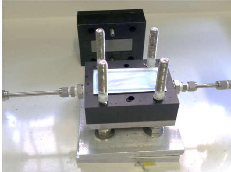
*Figure 4.8: Membrane sample located inside the cell*
