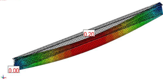
Figure 103: Dead load effect. left is expressed the continuous behaviour
