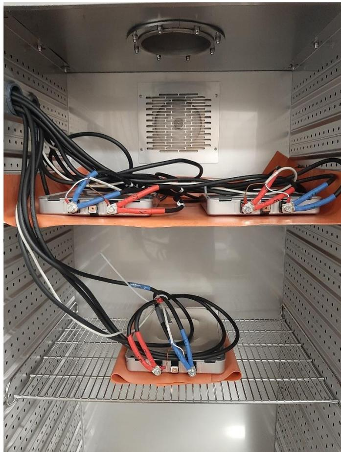
**Figure 5.9 Three Nissan Leaf 2011 Edition (24 kWh) modules during the testing.**
