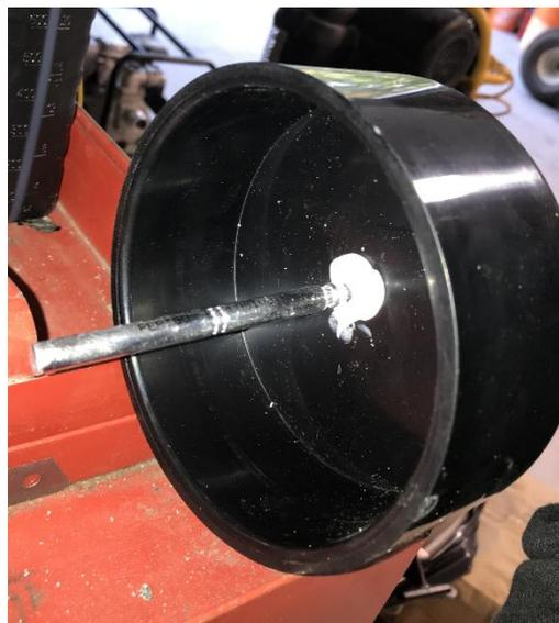
*Figure 67- NONEL Detonator Glued at the Bottom Plastic Cup*
