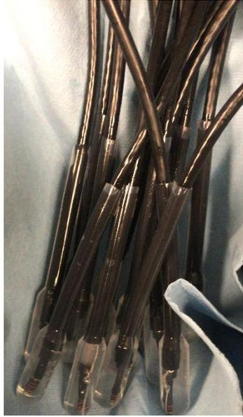
*Figure 51- Finished sensors, second typology, not sealed yet (always through using plastic ties)*
