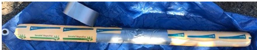
Figure 69- Connection of Two Cartridges of Emulsion.
