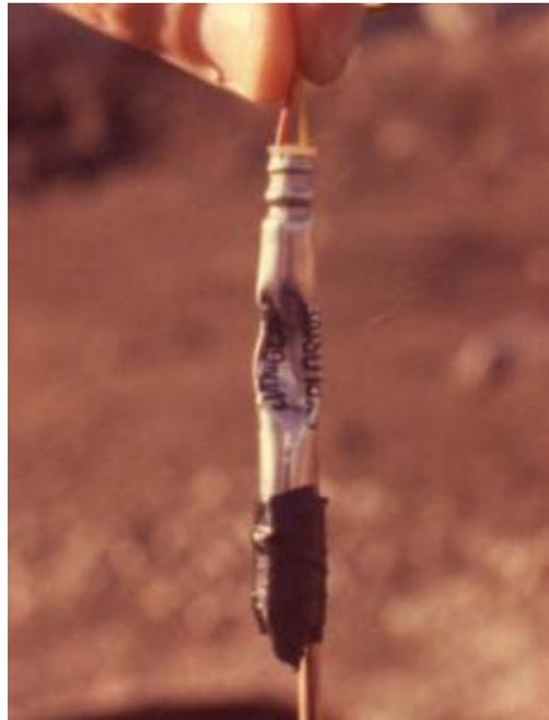
Figure 29- Damage due to a shock wave from an adjacent charge placed in a side borehole. Source: [www.iring.ca](http://www.iring.ca)
