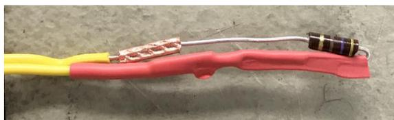
*Figure 52- CCR, third typology, before being insulated*
