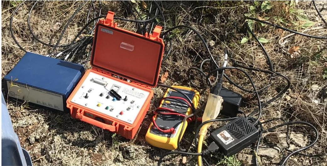
*Figure 54- First test's setup, starting from the left side, rightwards: Signal conditioner, Microtrap, Multimeter, Chargers.*
