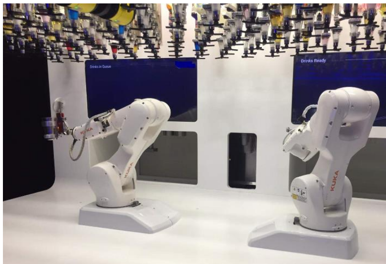
Figure 29, right robotic arm going back to homing, Taken from the factory of company D
