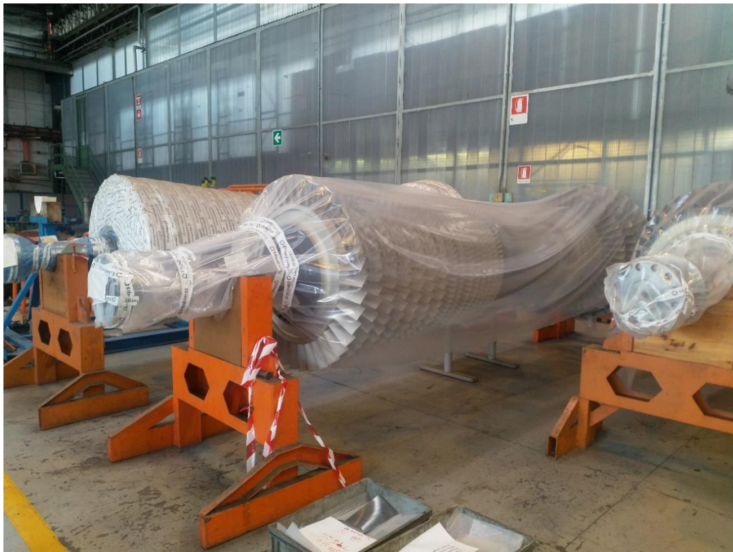
Figura 25: Turbina a gas
